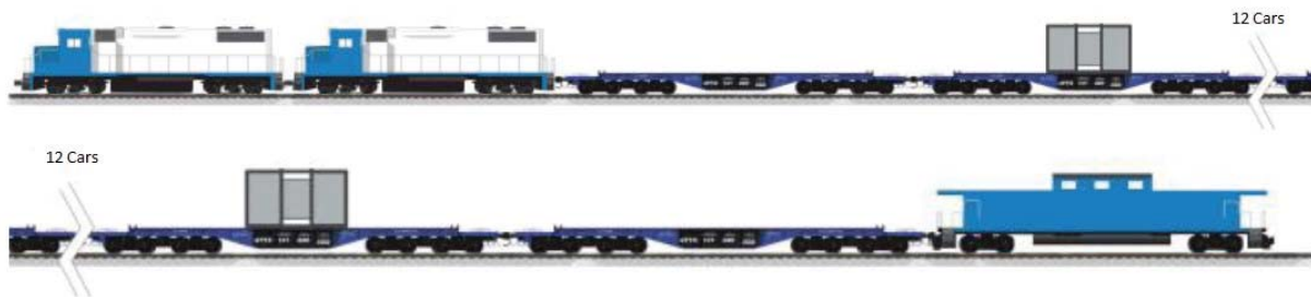
Figure 4: An illustration of the 8-axle Dry Storage Container Transportation Package Railcar
