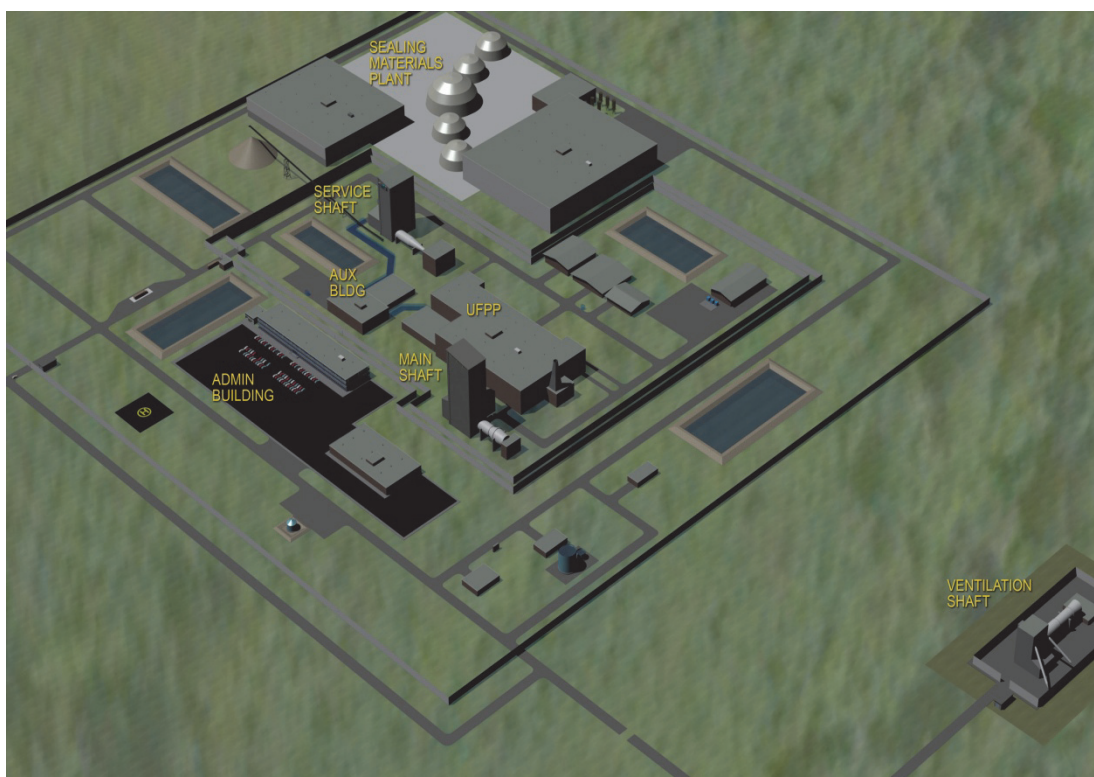
Figure 3-3: APM Surface Facilities
