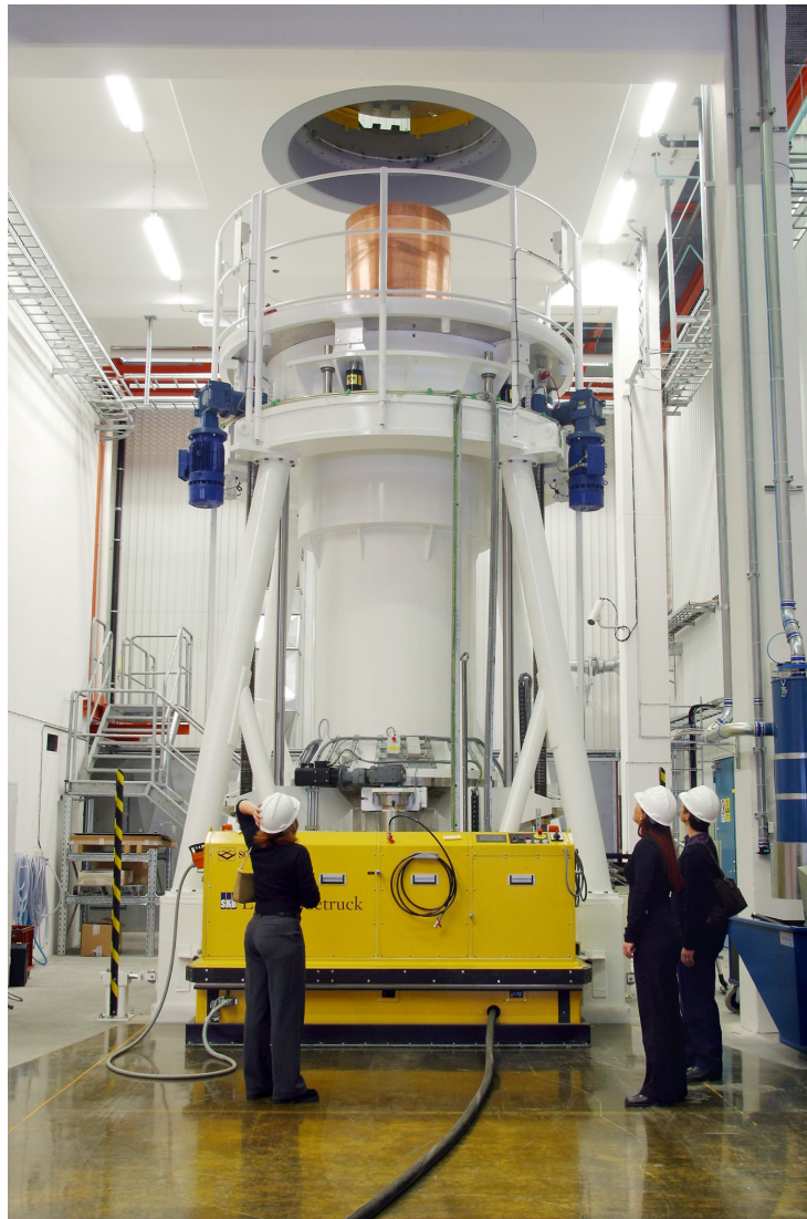
Figure 4-4: Shielded Frame and Air-cushion Transporter
