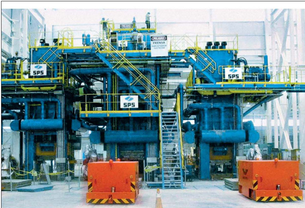
Figure 4-14: Example of a Closed-Die Forging Press
