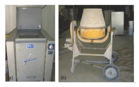
Figure 2: Equipment Used to Prepare Sand Component: (a) Powered Sieve Machine; (b) Concrete Mixer
