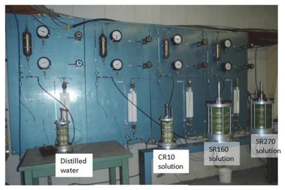
Figure 20: Four Triaxial Cells Used for Testing
