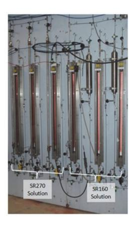
Six (6) permeability board ready for tests using SR160 and SR270 solutions
