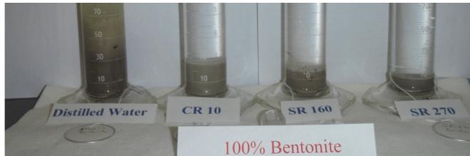
(a) Free Swell Tests of 100% Bentonite with Different Solutions
