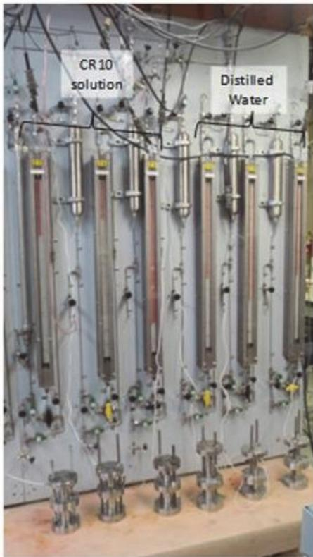
Six (6) Apparatus for Testing Using DW and CR10 Solutions
