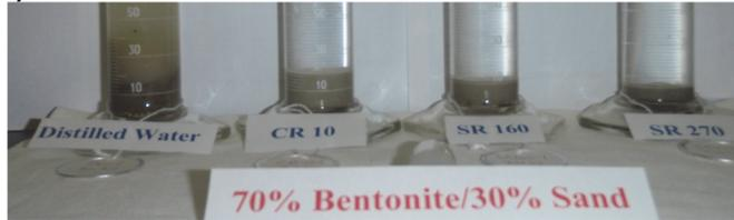
(b) Free Swell Tests of 70-30 Bentonite-Sand Mixture with Different Solutions
