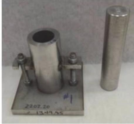
**Figure 9: Miniature Compaction Mould (Inside Diameter = 32 mm)**
