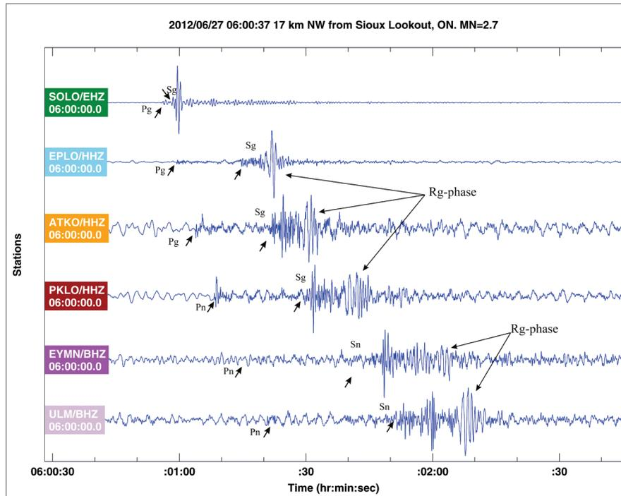
**Figure 8: Rg Surface Waves from the  $m_N$  2.7 on 2012/06/27, 18 km northwest of Sioux Lookout, ON**
