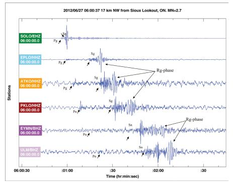
Figure 8: Rg Surface Waves from the  $m_N$  2.7 on 2012/06/27, 18 km northwest of Sioux Lookout, ON
