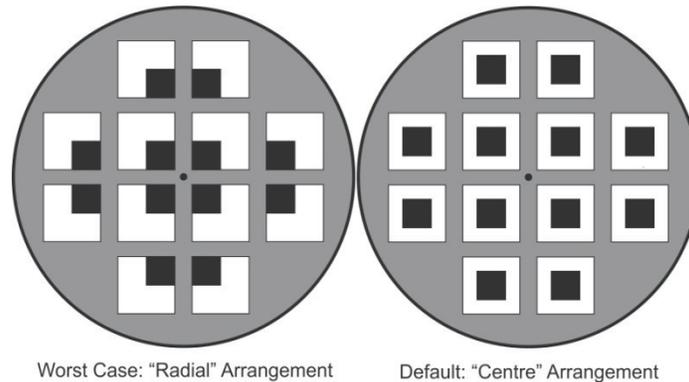
**Figure 2-1: Fuel Assembly Arrangement**
