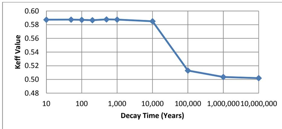
**Figure 7-1: Decay Time Versus  $k_{\text{eff}}$  – Intact-Container (log scale)**
