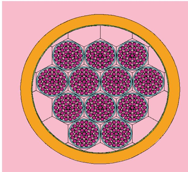
**Figure 5-3: 4L012 MCNP Model: Z Plane Slice**
