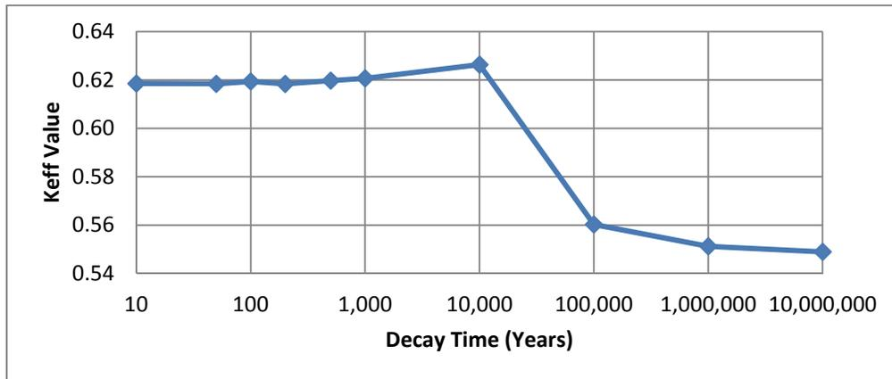
**Figure 7-2: Decay Time Versus  $k_{\text{eff}}$  – Degraded-Container (log scale)**
