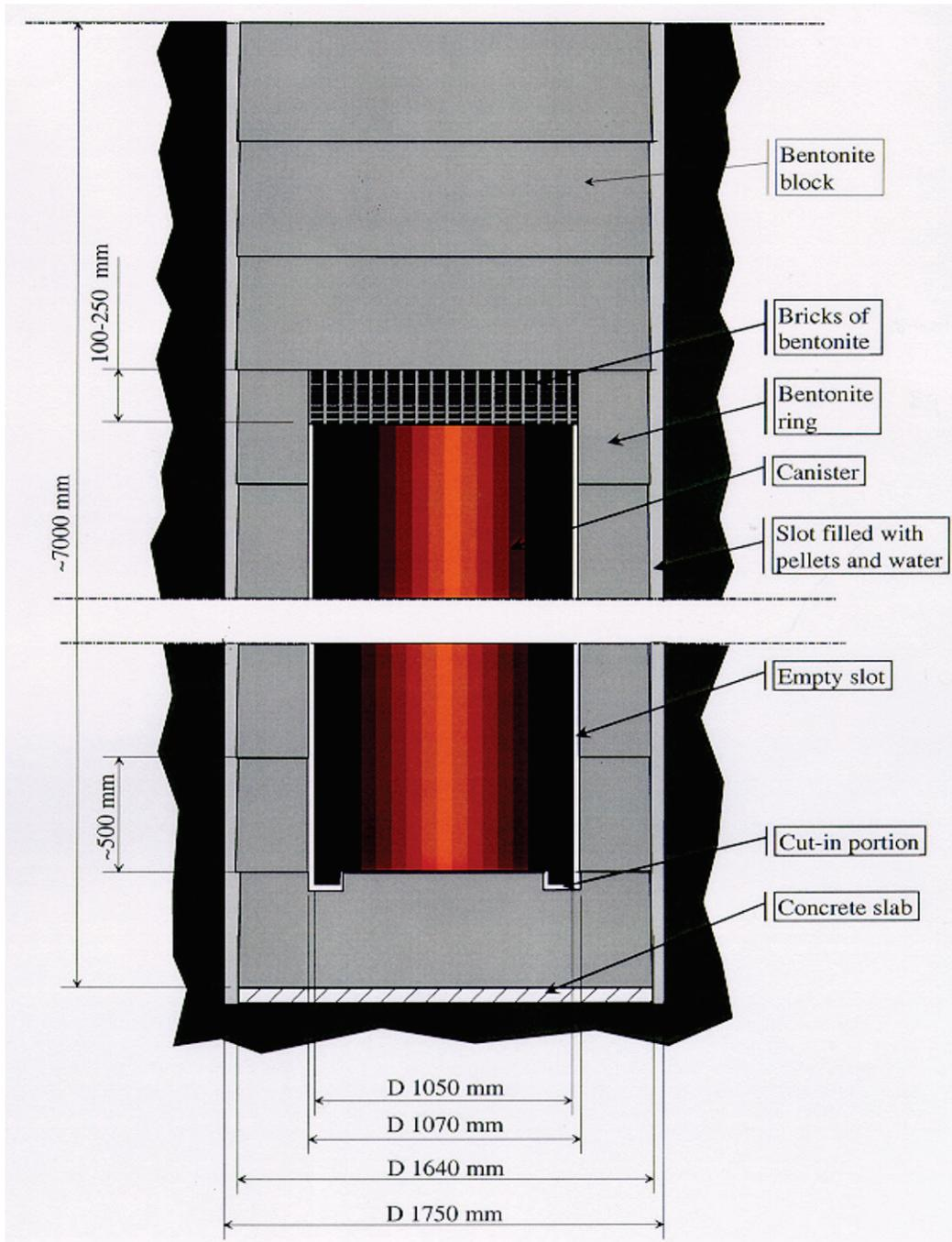
**Figure 3: Schematic Drawing of the CRT Canister Hole with Bentonite Blocks with Dimensions in mm**
