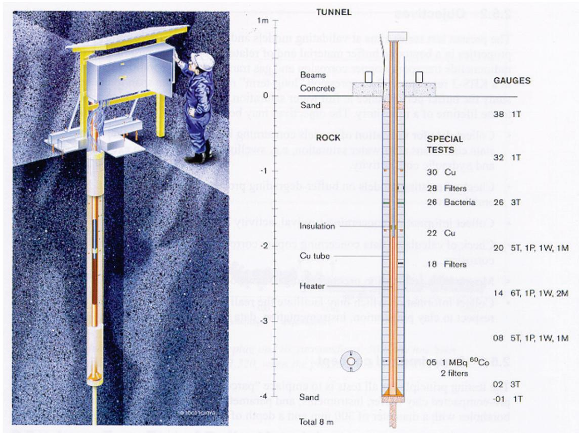
**Figure 1: Illustration of the Experimental Set-up in the Long-Term Test (LOT) of Buffer Material (left) and a Cross-section View of an S-type Parcel (right)**
