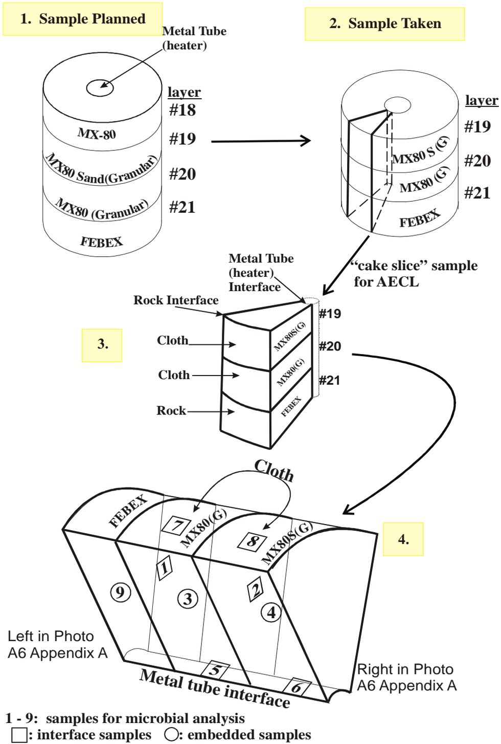
**Figure 43: Schematic of the ABM Test Package 1 Sample Analyzed by AECL and Location of the Nine Sub-samples for Microbial Analysis**
