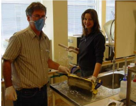
Figure B5: After cutting the outer steel bars of the two granulate cages (block 19 and 20), the stack of 3 blocks could be cut radially with a band saw. After these two radial cuts the “piece of cake” could be gently separated from the inner steel tube. The result is shown above with the clamp still attached. The sample was placed on plastic film.
