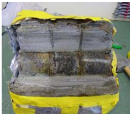
Figure B8: View of the triple block after cutting out the “piece of cake” for AECL studies. The FEBEX bentonite block (21) is on the left, MX-80 granulate (20) in the middle, and MX-80 s/b granulate on the right.
