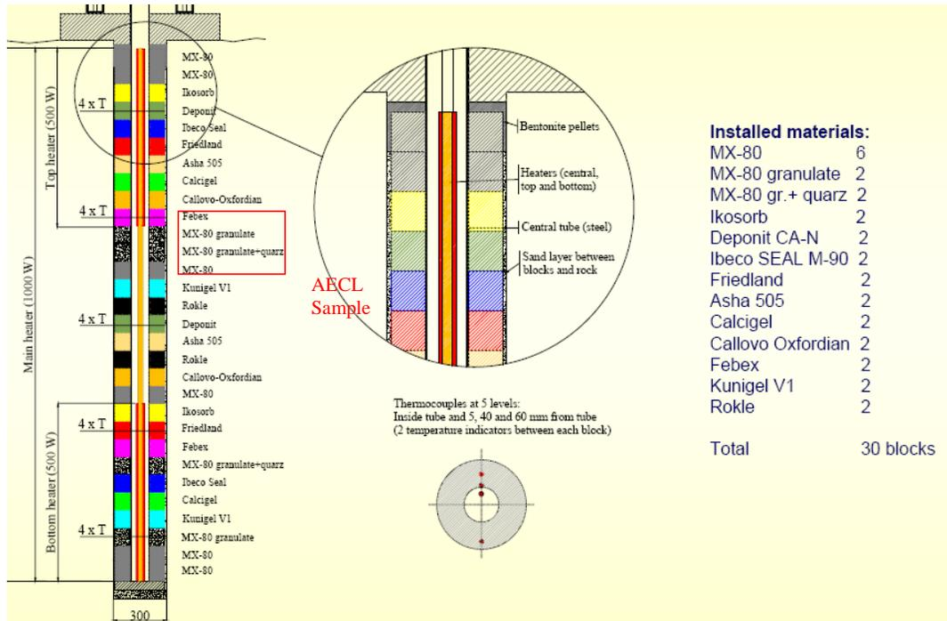
**Figure 33: Detailed Schematic of ABM Test Package 1**
