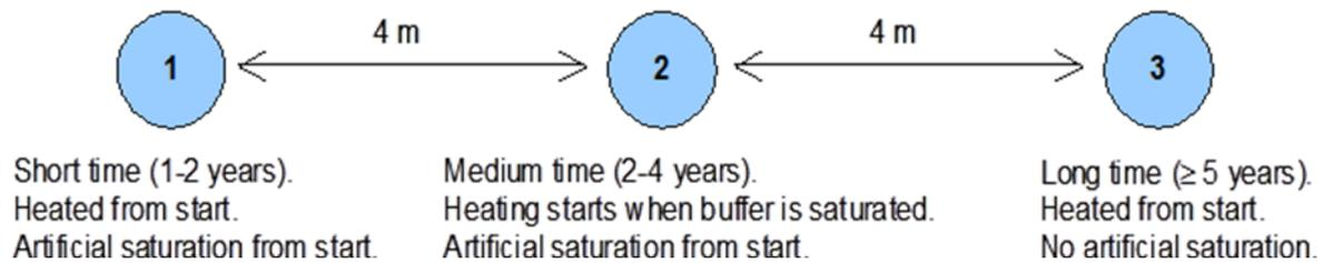
**Figure 2: Experimental Design for the Three ABM Experiments at Äspö**
