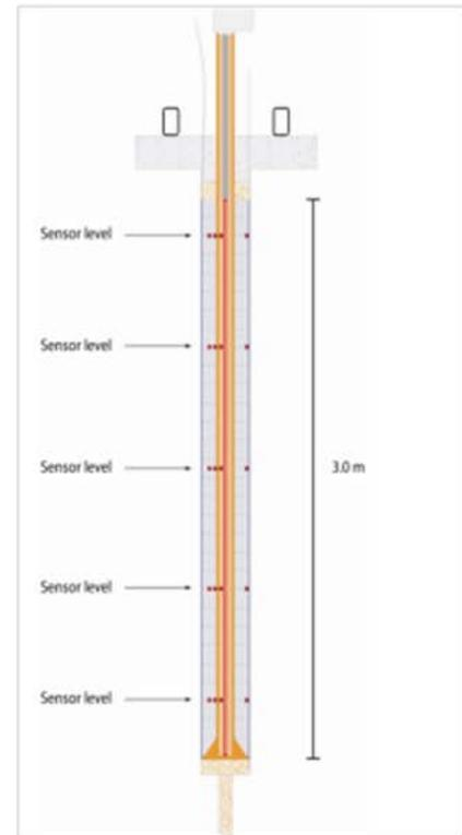
**Figure 5: Number and Type of Sensors in ABM Package Design**
