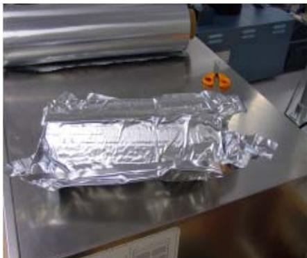
Figure B7: AECL sample after vacuum packaging with plasticized aluminum. Two sealed bags were applied for better physical stability of the sample. There is some plastic film as an innermost wrapping.
