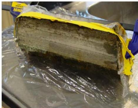
Figure B6: Close up of the “piece of cake”. There are no separation lines visible between the blocks. The slightly greenish colour of the FEBEX bentonite (block 21) is visible on the left. The MX-80 granulate is in the middle (block 20), and the MX-80 s/b granulate is on the right side (block 19). There is fabric still attached to the outer surface of the granulate material. This fabric was placed there initially to allow filling of the granulate into the stack.
