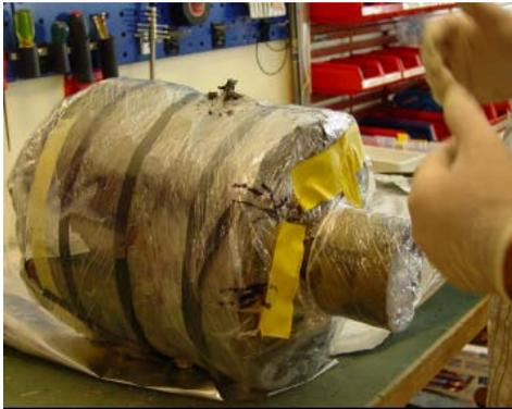
Figure B3: Packet of three blocks (19/20/21) after removal of MX-80 bentonite block (18). Block 18 was removed by mistake – it should have been block 21 (FEBEX). The packet was protected by plastic film immediately after it was unpacked from the plasticized aluminum foil (e.g. after image 19 was taken).
