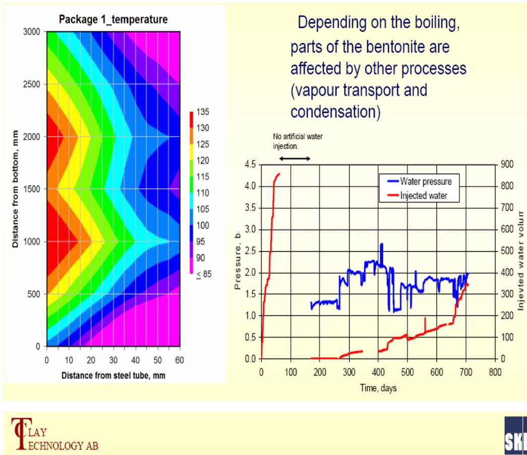
Figure 36: Artificial Water Saturation in ABM Test Package 1
