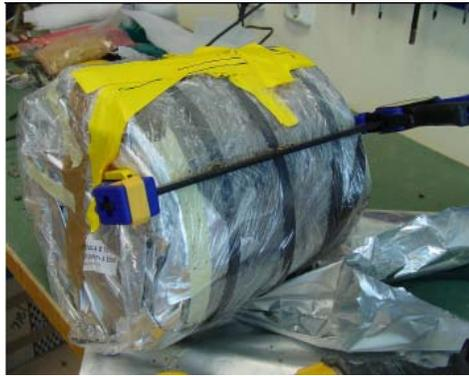
Figure B4: Packet of three blocks (19/20/21) after removal of MX-80 bentonite block (18). A clamp was used to ensure that the blocks would not part during sample handling. Sample handling included cutting through the outer steel bars of the two granulate cages. This was done with a tiger saw and involved some force. The “piece of cake” to be cut out was located between the radial “spokes” of the cage placed at 90° angles.
