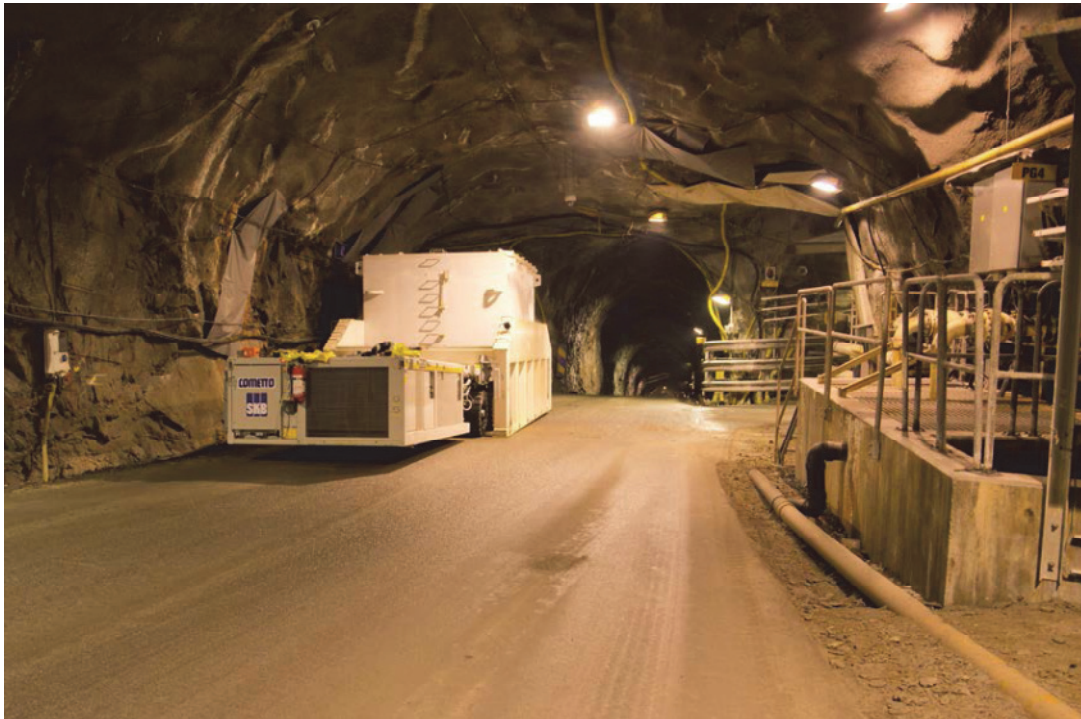
Figure 2.3: Prototype of SKB's Ramp Vehicle for Canister Transport Casks
