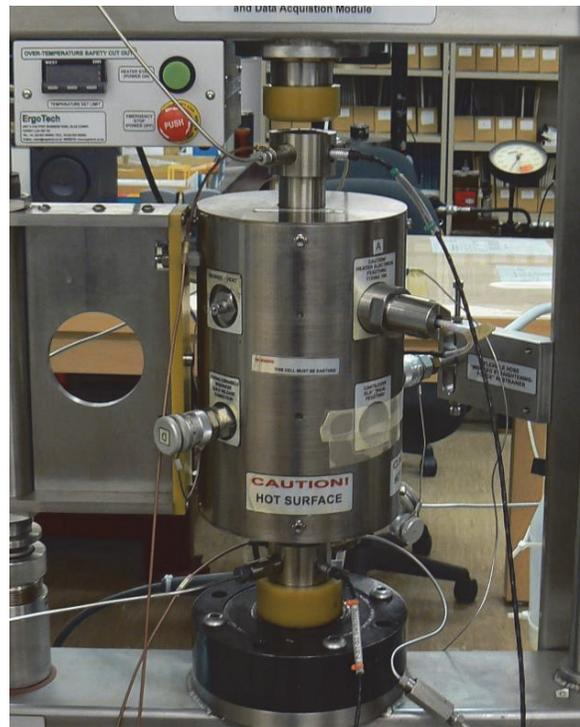
**Figure 2: Floor Standing Acoustic System for testing under thermal treatment and hydrostatic pressures**
