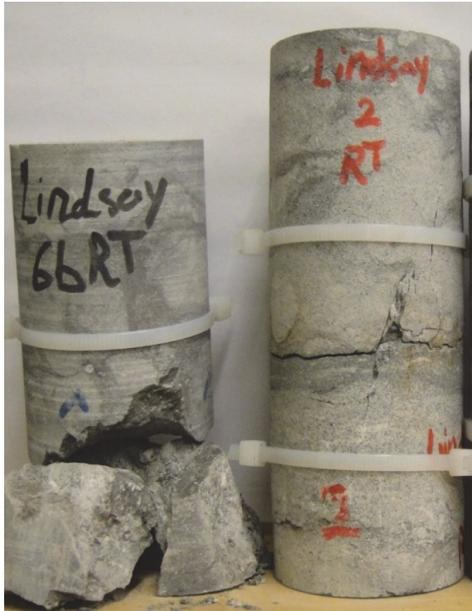
**Figure 64: A photo of Specimens L2 and L6b after tests**
