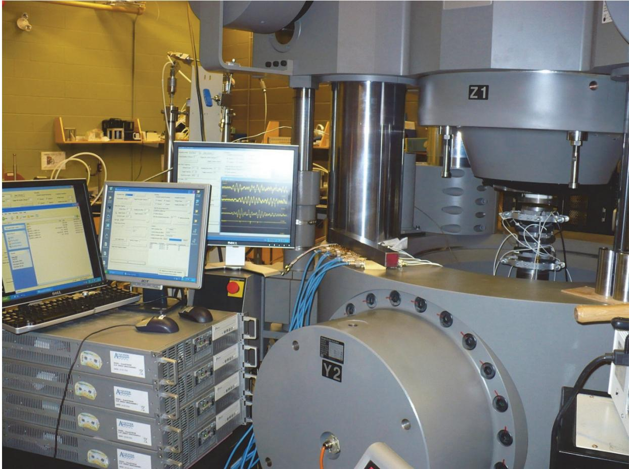
**Figure A2: Experimental set-up, showing larger specimen of Cobourg limestone secured with 8 PAC AE sensors and continuous data acquisition system under UCS test**
