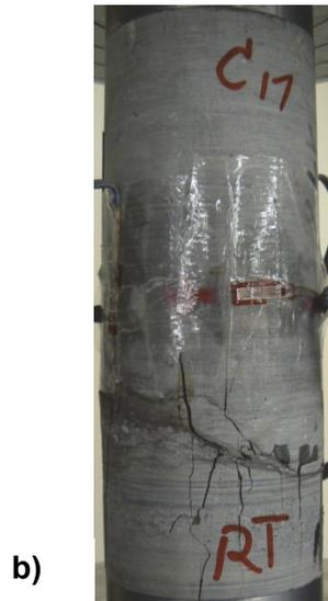
Figure 17: (a) Volumetric strain for saturated Specimens, C3 and C17, for ambient temperature and (b) a 75° inclined failure plane of Specimen C17
