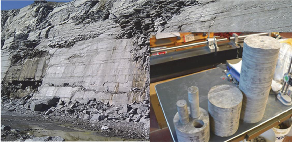
**Figure 45: St. Mary's cement's quarry in Bowmansville and cored samples**
