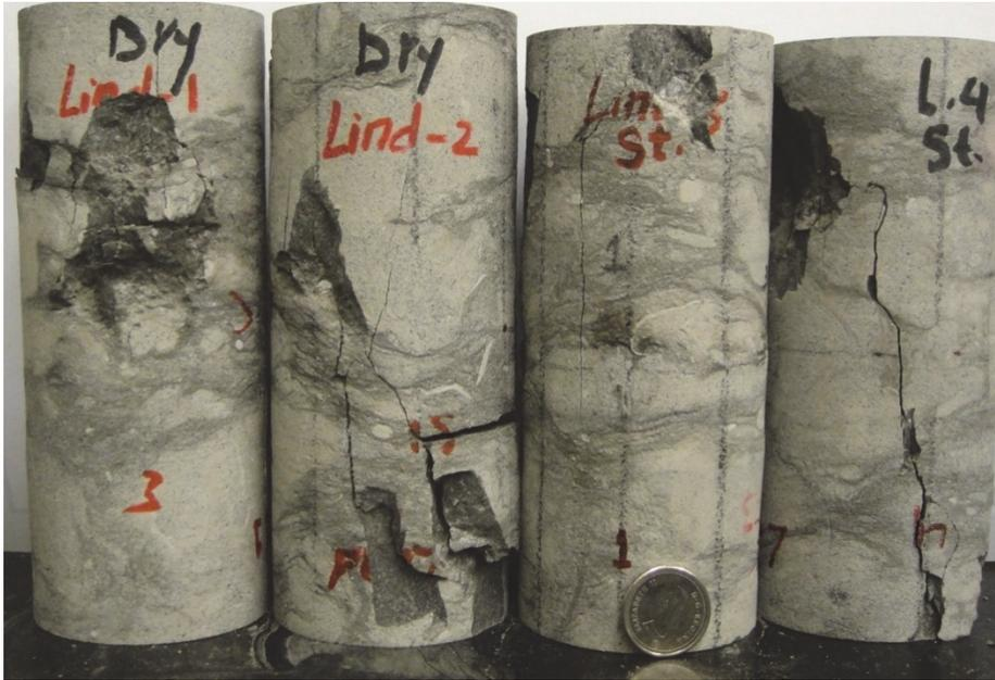
Figure 53: A photo of Specimens L1-RT, L2-RT, L3-RTS and L4-RTS after tests
