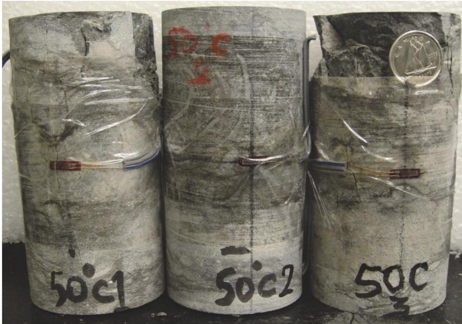
Figure 57: A photo of thermally treated Specimens L1-50 C, L2-50 C and L3-50 C after tests
