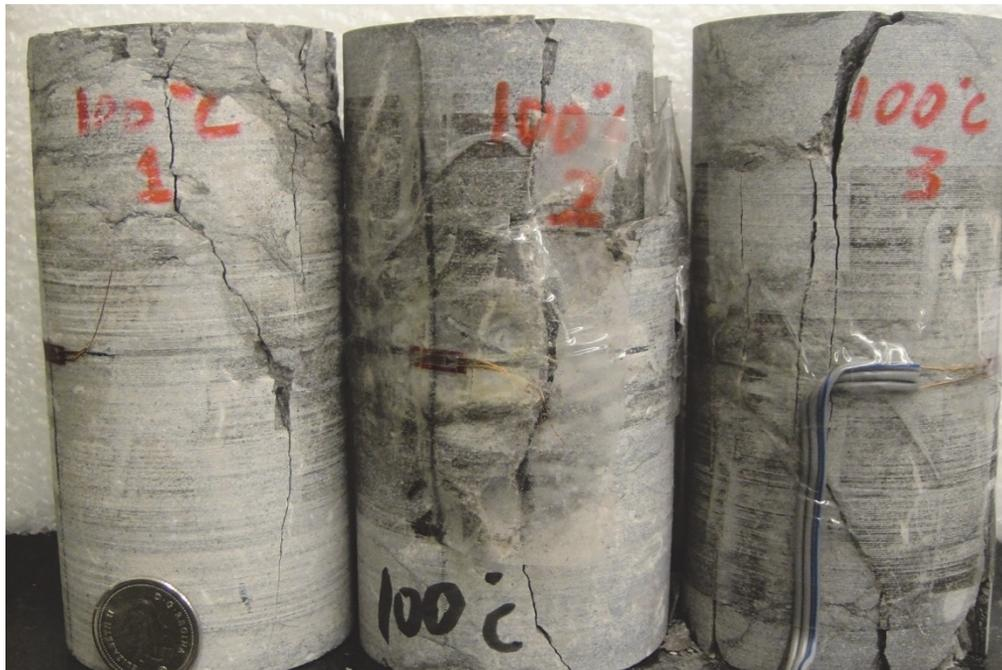
Figure 58: A photo of thermally treated Specimens L1-100 C, L2-100 C and L3-100 C after tests
