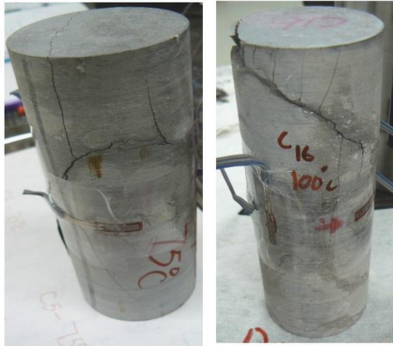
**Figure 5: Pictures of pre-mature failure of Specimen C16 and C24 (saturated), thermally treated at 75 and 100°C before testing**
