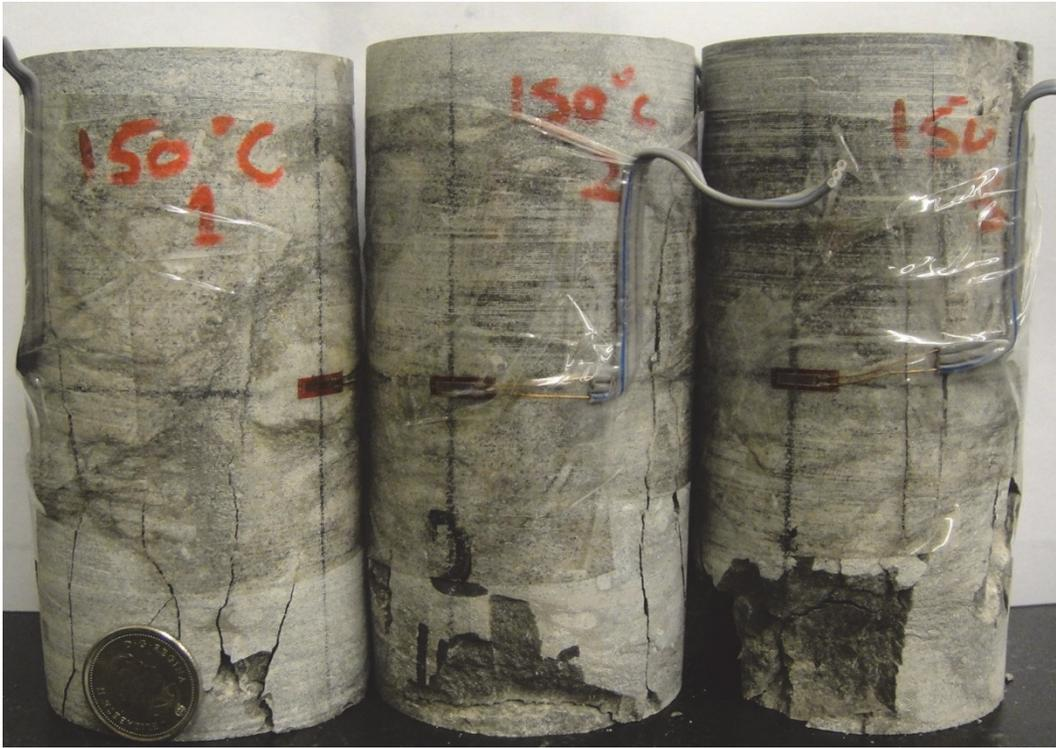
**Figure 59: A photo of thermally treated Specimens L1-150 C, L2-150 C and L3-150 C after tests**
