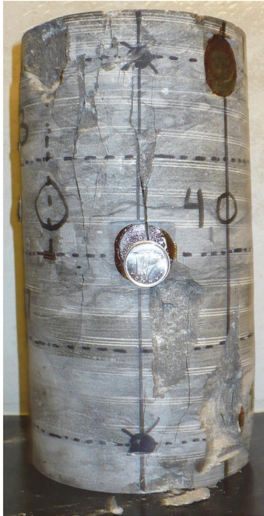
**Figure A7: Tested larger Cobourg limestone specimen for AE analysis showing failure pattern characterized with axial failure planes**
