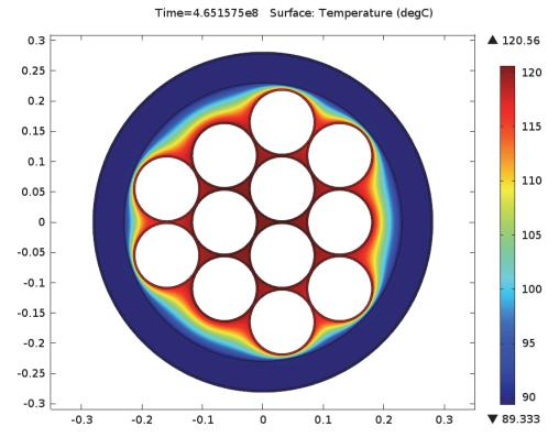
Figure 47: Temperature on the z = 0 Plane (Middle Cross Section of a Container) at 14.7 Years for the Container inside the Buffer Box in the Crystalline Repository Case
