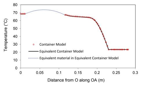
Figure 64: Container Temperature Comparison along Line OA at 8.6 Days between the Container Model and the Equivalent Container Model
