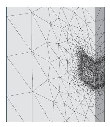
Figure 6: Finite Element Discretization of the Central Part of the Unit Cell of the Sedimentary DGR Model for Near-Field Analyses
