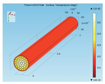
Figure 40: Fuel Temperature in the Bundle Model at 14.7 Years for the Container inside the Buffer Box in a Sedimentary Repository Case
