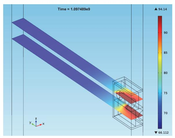
Figure 44: Rock Temperature at the Repository Level at 34.8 Years for the Container inside the Buffer Box in the Crystalline Repository Case
