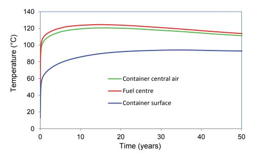
Figure 50: Temperatures for the Container inside the Buffer Box in the Crystalline Repository Case
