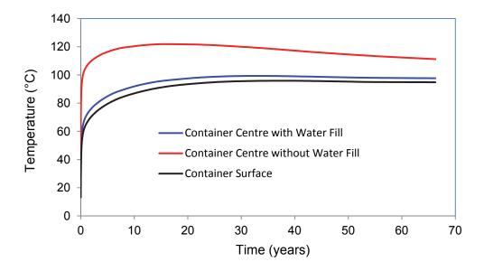
Figure 75: Effect of Water Entering the Container on Container Centre Temperature for the Container inside the Buffer Box in a Sedimentary Repository Case
