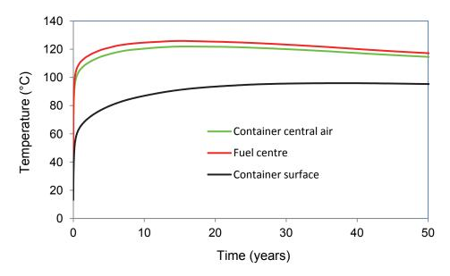
Figure 42: Temperatures as a Function of Time for the Container inside the Buffer Box in a Sedimentary Repository Case
