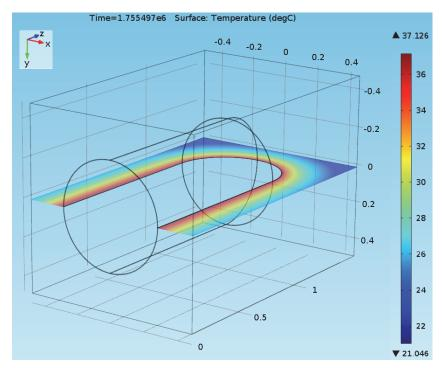
Figure 28: Buffer Box Temperature on the y = 0 Plane at 20 Days for the Container inside the Buffer Box in Air Case
