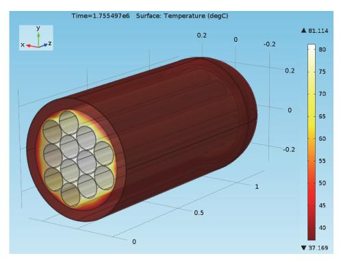
Figure 29: Container Temperature at 20 Days for the Container inside the Buffer Box in Air Case
