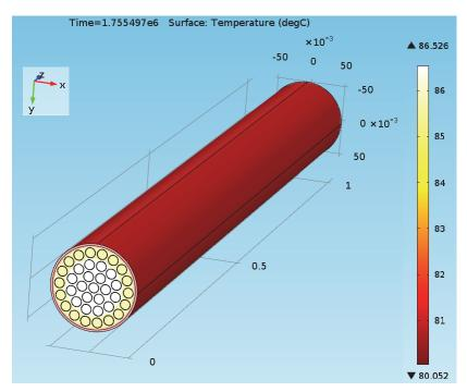
Figure 32: Fuel Temperature at 20 Days for the Container inside the Buffer Box in Air Case
