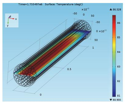
Figure 33: Fuel Temperature on the y = 0 Plane at 20 Days for the Container inside the Buffer Box in Air Case
