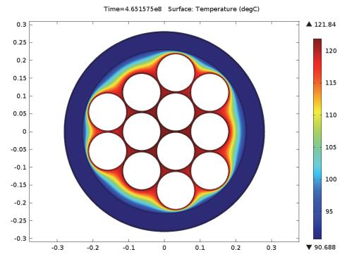
Figure 39: Temperature Distribution on the z = 0 Plane (Middle Cross Section of a Container) at 14.7 Years for the Container inside the Buffer Box in a Sedimentary Repository Case
