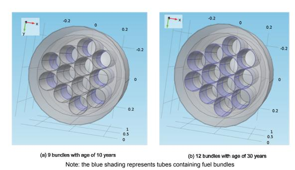
Figure 51: Bundle Distribution in a Mixed Heat Source Model I in a Sedimentary Repository
