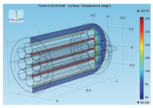
Figure 46: Temperature on the x = 0 Plane at 14.7 Years for the Container inside the Buffer Box in the Crystalline Repository Case
