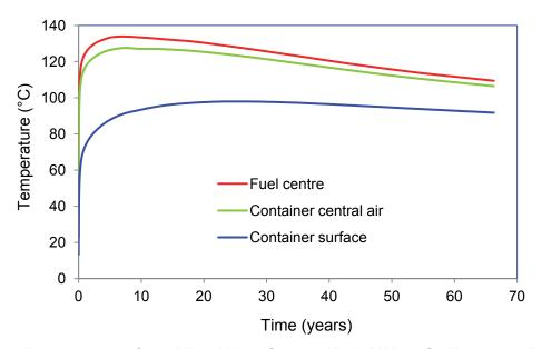
Figure 54: Temperatures from Mixed Heat Source Model II in a Sedimentary Repository
