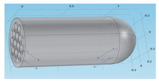
Figure 72: Container Model with Partial Connections (Only connections A, B, C and D are effective)
