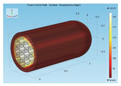
Figure 37: Container Temperature at 14.7 Years for the Container inside the Buffer Box in the Sedimentary Repository Case
