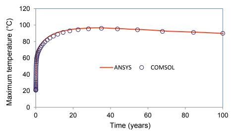
Figure 19: Maximum Temperatures in the Sedimentary Rock DGR Model obtained using ANSYS and COMSOL
