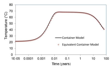
Figure 63: Container Centre Air Temperature Comparison between the Container Model and the Equivalent Container Model
