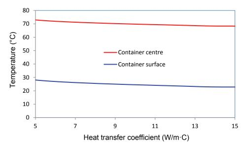
Figure 88: Influence of the Convective Heat Transfer Coefficient on Container Centre Air Temperature
