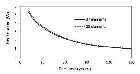
Figure 15: Heat Source per 28-Element Bundle and per 37-Element Bundle for a Discharge Burnup of 220 MWh/(kgU)
