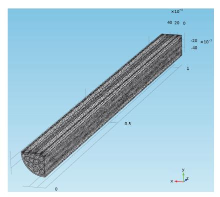
Figure 84: Radiation Bundle Model Mesh
