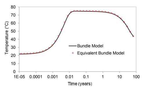
Figure 60: Fuel Centre Temperature Comparison between the Bundle Model and the Equivalent Bundle Model
