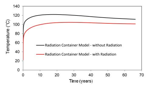
Figure 82: Influence of Radiation Heat Transfer on Container Air Temperature
