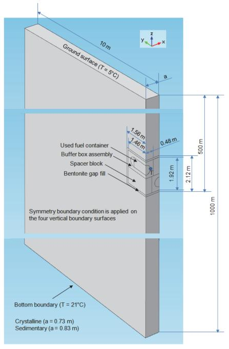
Figure 5: Sedimentary and Crystalline DGR Model Geometry
