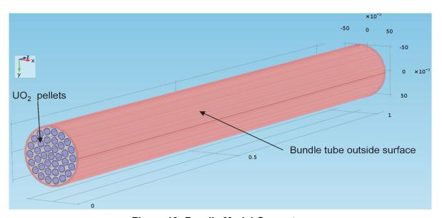
Figure 18: Bundle Model Geometry
