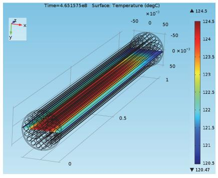
Figure 49: Fuel Temperature on the y = 0 Plane at 14.7 Years for the Container inside the Buffer Box in the Crystalline Repository Case
