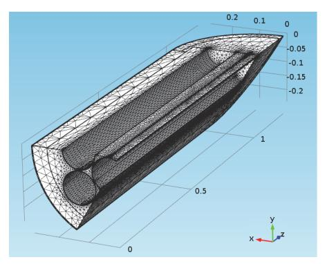
Figure 77: Radiation Container Model Mesh
