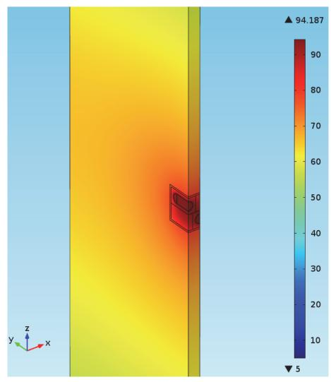
Figure 43: Rock Temperature at 34.8 Years for the Container inside the Buffer Box in the Crystalline Repository Case
