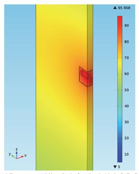
Figure 35: Rock Temperature at 40 Years for the Container inside the Buffer Box in the Sedimentary Repository Case
