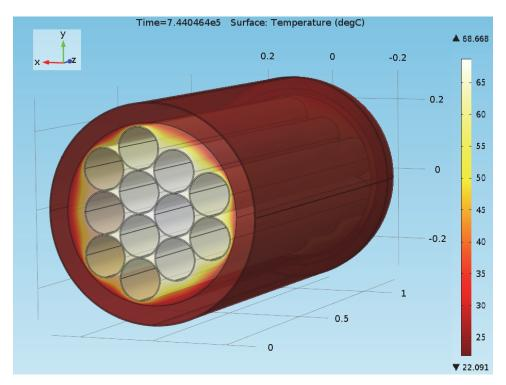
Figure 21: Container Temperatures at 8.6 Days for the Container in Air Case
