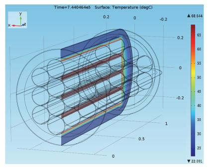
Figure 22: Container Temperatures on the x= 0 Plane at 8.6 Days for the Container in Air Case
