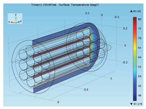
Figure 30: Container Temperature on the x = 0 Plane at 20 Days for the Container inside the Buffer Box in Air Case
