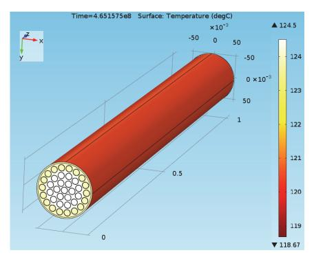
Figure 48: Fuel Temperature in the Bundle Model at 14.7 Years for the Container inside the Buffer Box in the Crystalline Repository Case
