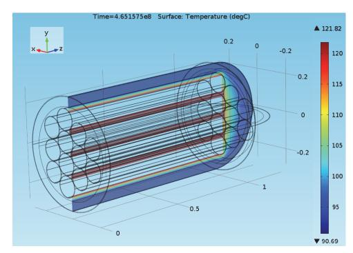
Figure 38: Temperature on the x= 0 Plane at 14.7 Years for the Container inside the Buffer Box in a Sedimentary Repository Case
