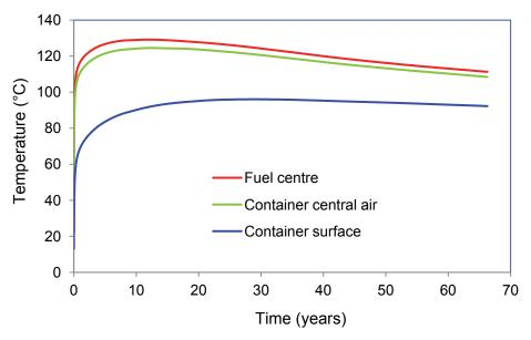
Figure 52: Temperatures from Mixed Heat Source Model I in a Sedimentary Repository
