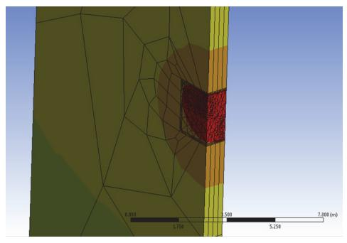
Figure 20: Finite Element Discretization of the Central Part of the Unit Cell for Near-Field Analyses for the ANSYS Model
