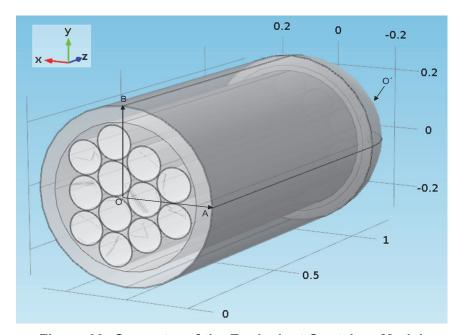
Figure 62: Geometry of the Equivalent Container Model
