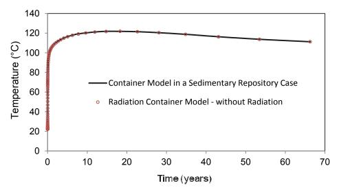
Figure 78: Container Centre Temperature for the Container inside the Buffer Box in the Sedimentary Repository Case
