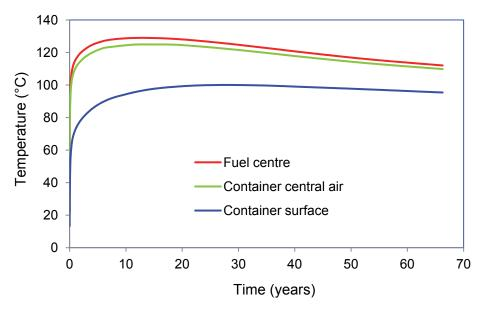
Figure 56: Temperatures from Mixed Heat Source Model III in a Sedimentary Repository
