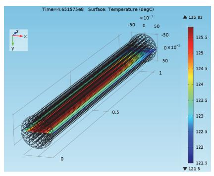
Figure 41: Fuel Temperature on the y = 0 Plane at 14.7 Years for the Container inside the Buffer Box in a Sedimentary Repository Case
