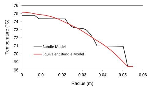
Figure 61: Fuel Temperature Comparison along Radius (OA) between the Bundle Model and the Equivalent Bundle Model
