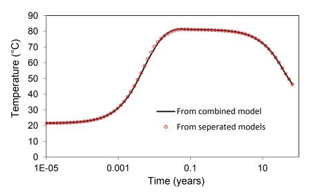
Figure 67: Container Air Temperatures Comparison between the Buffer Box Combination Model and the Separated Models
