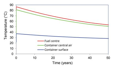
Figure 34: Temperatures as a Function of Time for the Container inside the Buffer Box in Air Case
