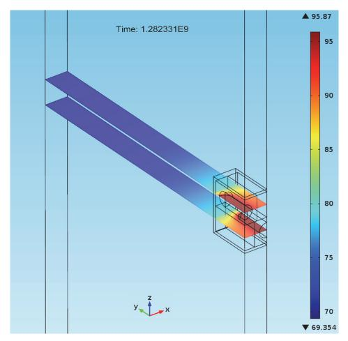
Figure 36: Rock Temperature at the Repository Level at 40 Years for the Container inside the Buffer Box in the Sedimentary Repository Case
