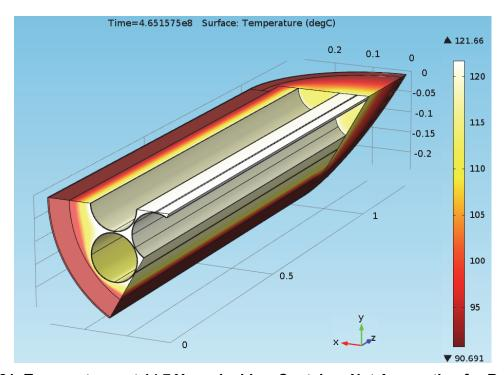
Figure 81: Temperatures at 14.7 Years inside a Container Not Accounting for Radiation Heat Transfer
