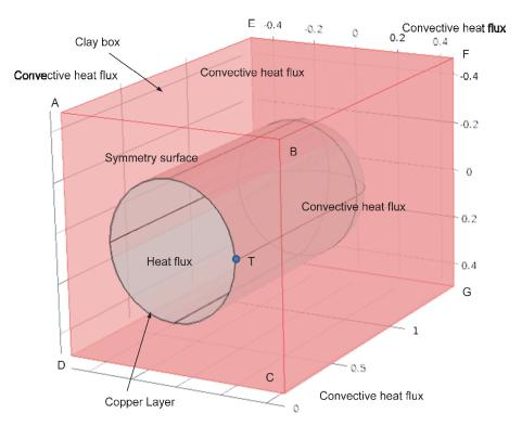
Figure 16: Buffer Box Model Heat Flux Boundary Conditions
