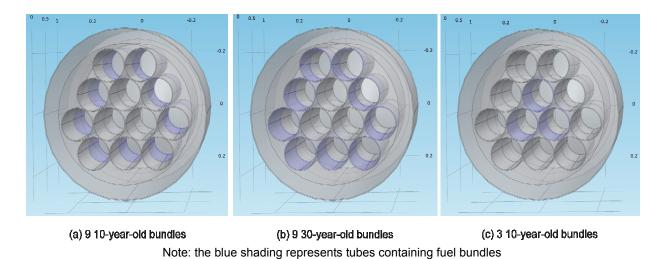
Figure 57: Bundle Distribution in Mixed Heat Source Model IV in a Sedimentary Repository
