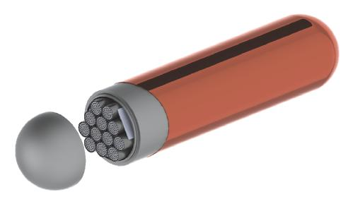
Figure 1: Mark II Used Fuel Container View
