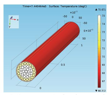
Figure 24: Fuel Temperatures at 8.6 Days for the Container in Air Case
