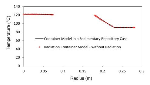
Figure 79: Temperature along Line OA for the Container inside the Buffer Box in the Sedimentary Repository Case
