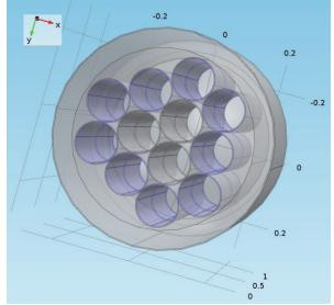
Note: the blue shading represents tubes containing fuel bundles
