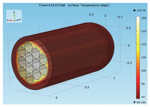
Figure 45: Container Temperature at 14.7 Years for the Container inside the Buffer Box in the Crystalline Repository Case
