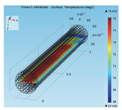
Figure 25: Fuel Temperatures on the y = 0 Plane at 8.6 Days for the Container in Air Case
