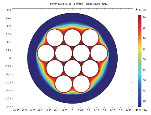
Figure 31: Container Temperatures on the z = 0 Place (Middle Cross Section of a Container) at 20 Days for the Container inside the Buffer Box in Air Case
