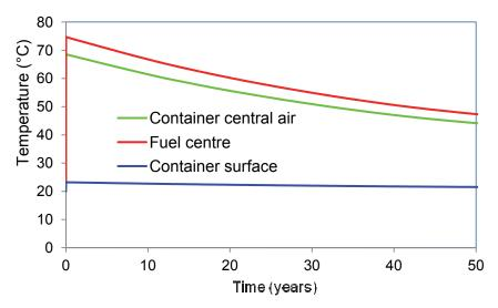
Figure 26: Temperatures as a Function of Time for the Container in Air Case
