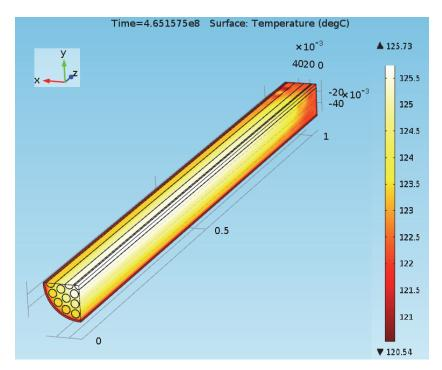
Figure 86: Temperatures in the Bundle Model (radiation not modelled)
