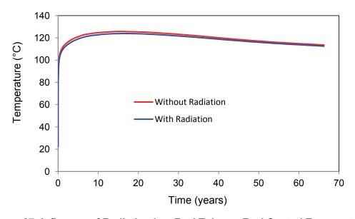
Figure 87: Influence of Radiation in a Fuel Tube on Fuel Central Temperature
