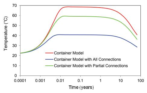
Figure 73: Influence of Connections on the Maximum Container Air Temperature for the Container in Air Case
