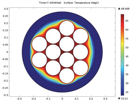
Figure 23: Container Temperatures on the z = 0 Plane (Middle Cross Section of a Container) at 8.6 Days for the Container in Air Case
