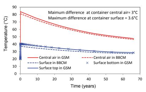
Figure 70: Container Temperature Comparison between Buffer Box Combination Model (BBCM) and Gap Sensitivity Model (GSM)
