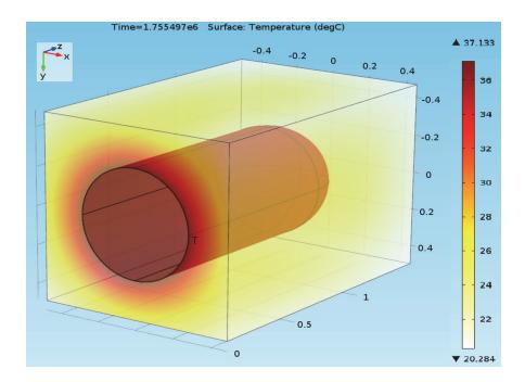
Figure 27: Buffer Box Temperature at 20 Days for the Container inside the Buffer Box in Air Case
