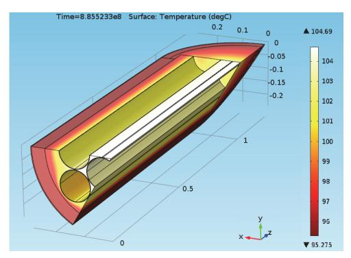
Figure 80: Temperatures at 28 Years inside the Container Accounting for Radiation Heat Transfer
