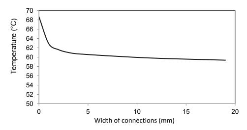
Figure 74: Influence of Connection Width on the Container Central Air Temperatures
