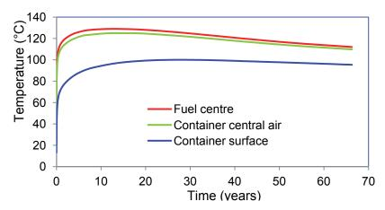
Figure 58: Temperatures from Mixed Heat Source Model IV in a Sedimentary Repository
