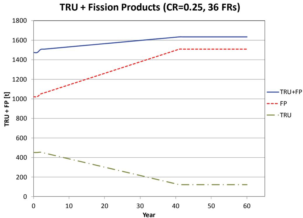
**Figure 3: Total TRU and Fission Products System Inventory for Scenario with Fast Reactors with a Favourable Very Low Conversion Ratio (CR=0.25), Starting from 103,000  $t_{HM}$  CANDU Used Fuel, (a) 2 FR; (b) 36 FR**
