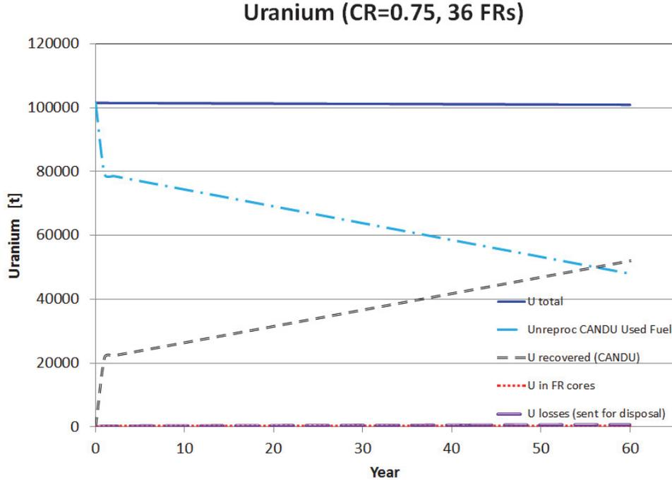
**Figure 6 (cont.): Total Uranium System Inventory for Scenario with 36 Fast Reactors Starting from 103,000 t<sub>HM</sub> CANDU Used Fuel, for Three Conversion Ratios (0.25, 0.5, 0.75)**
