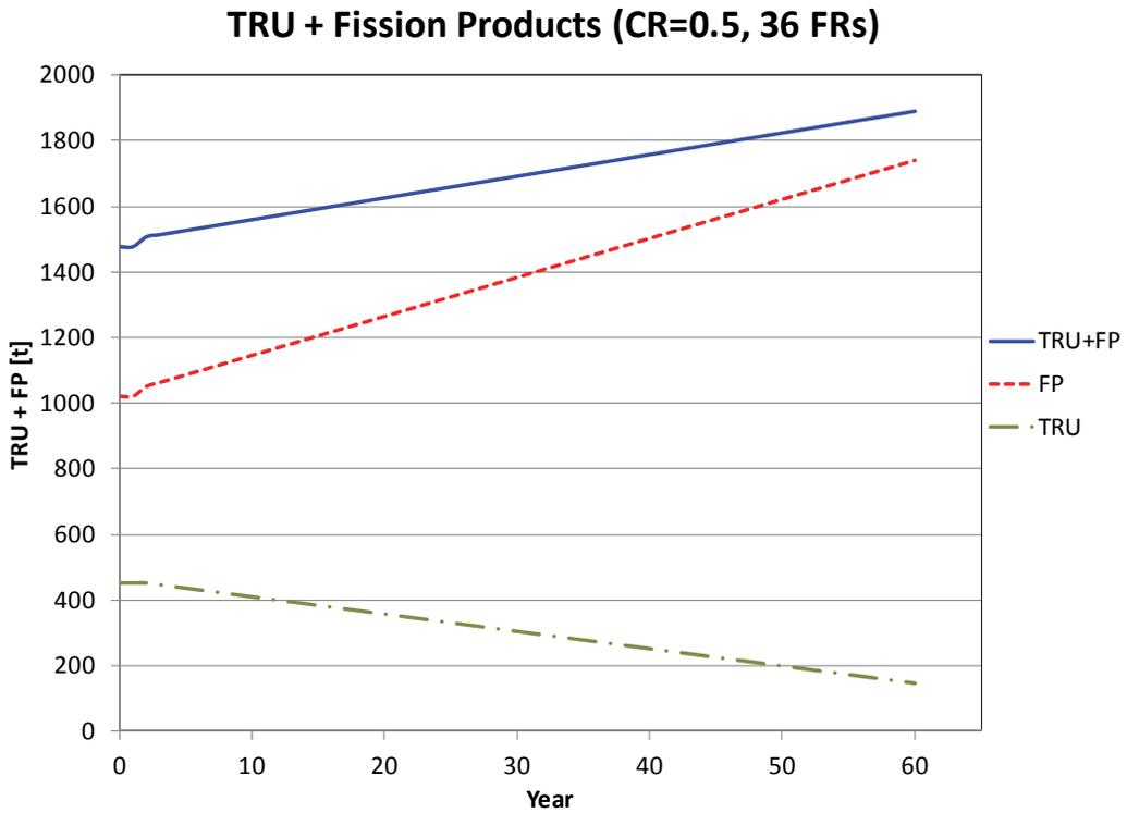
**Figure 4: Total TRU and Fission Products System Inventory for Scenario with Fast Reactors with a Low Conversion Ratio (CR=0.5), Starting from 103,000 t<sub>HM</sub> CANDU Used Fuel, (a) 2 FR; (b) 36 FR**
