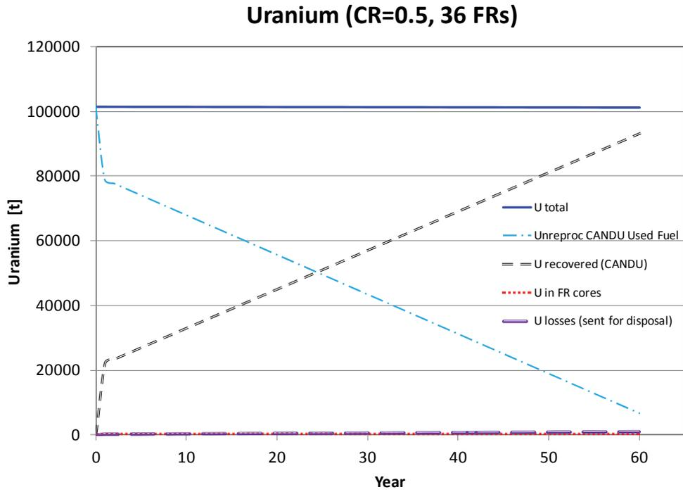
**Figure 6: Total Uranium System Inventory for Scenario with 36 Fast Reactors Starting from 103,000 t<sub>HM</sub> CANDU Used Fuel, for Three Conversion Ratios (0.25, 0.5, 0.75)**
