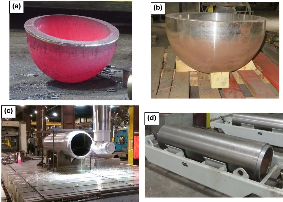
**Figure 3.7: Mark 2 Steel Shell and Hemi-Head Components Fabricated as Part of UFC Machining Program. Hemi-head in (a) as-formed Condition and (b), After Intermediate Machining Step. Shell During Machining (c) and, (d) in Final Configuration**
