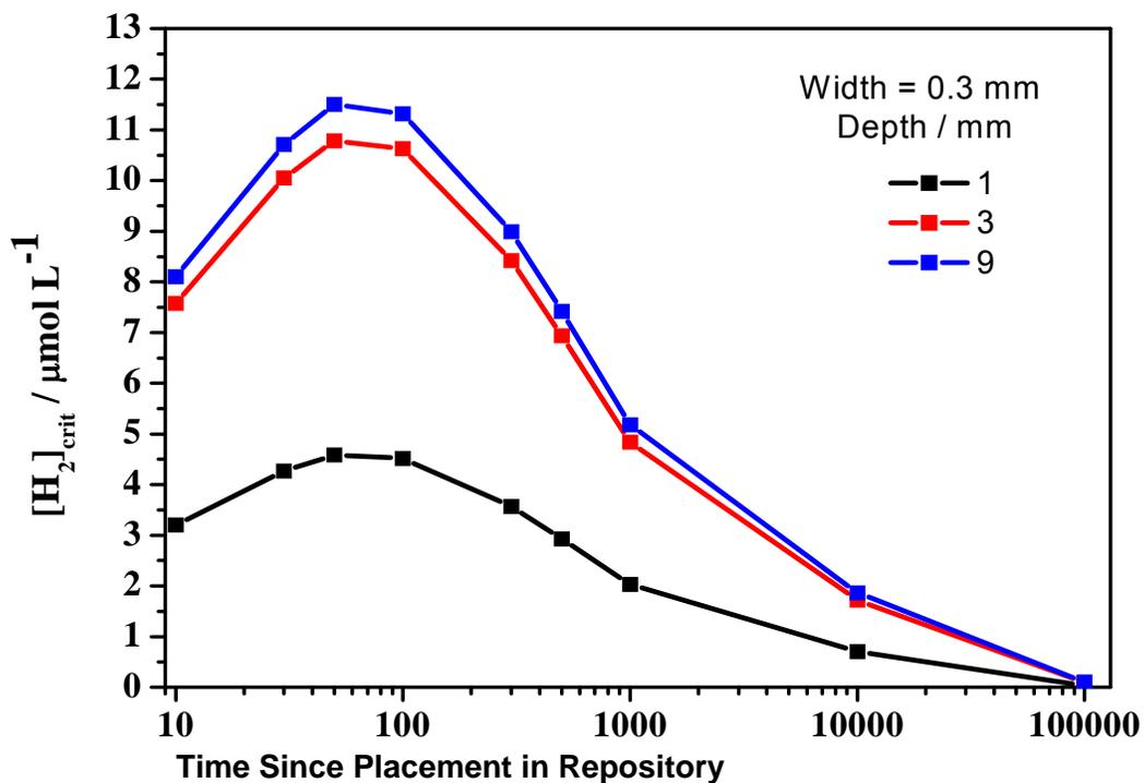
Figure 5.2: The critical [H<sub>2</sub>] as a Function of Time Since Placement of the Fuel in the Repository for Various Crack Depths and a Crack Width of 0.3 mm.
