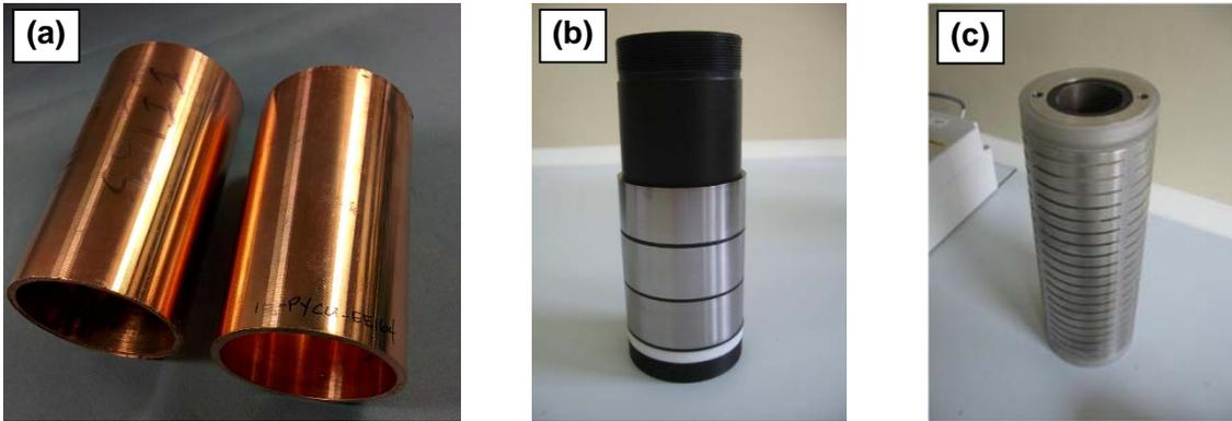
**Figure 3.16: Collaborative Analysis Program MaCoTe Components, Including (a) Electrodeposited Copper Samples; (b) A Test Module That Has Been Partly Assembled Using Steel Samples; (c) A Complete Module Ready For Emplacement in the Grimsel Test Site**
