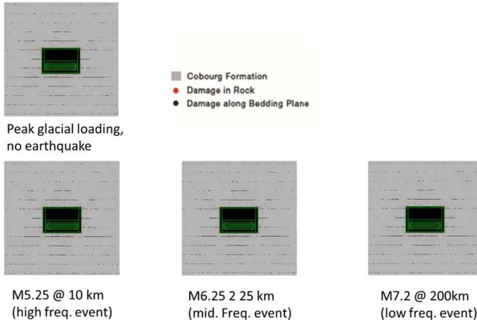
**Figure 4.4: Microcracks in the Rock at Peak Glacial Load Subjected to Three Different Earthquakes at  $10^{-6}$  p.a. Probability Level in Sedimentary Rock**
