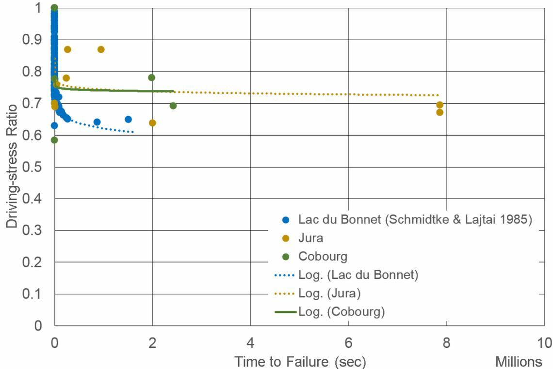
**Figure 4.1: Comparison of Time-to-Failure Results from Static Fatigue Testing on the Lac du Bonnet Granite, the Jura Limestone and the Cobourg Limestone**
