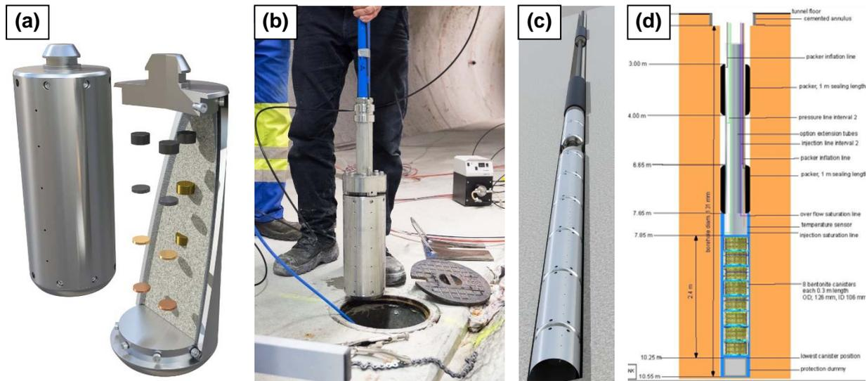
**Figure 3.29: Materials Corrosion Test at the Grimsel Underground Research Laboratory Illustrating (a) Copper and Steel Corrosion Coupons in Bentonite (b) Insertion/removal of Borehole Module and Series of Modules Within the Borehole as (c) Cartoon and (d) Schematic Showing Depths and Packers**
