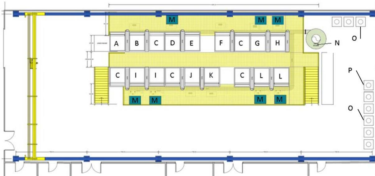
**Figure 3.15: Layout of an Optimized Electroplating Pilot Cell Facility for Copper Coating UFC's: (A) Hot Rinse, (B) Soak Clean, (C) Spray Rinse, (D) Electroclean, (E) Immersion Rinse, (F) Pickle [acid salts], (G) Electropolish, (H) Nickel Strike, (I) Copper Plate [Nanovate], (J) Microetch, (K) H<sub>2</sub>SO<sub>4</sub> Dip, (L) Cyanide Copper Plate, (M) Rectifier, (N) Vertical Scrubber, (O) Process Chemicals Tote, (P) Wastewater Tote**
