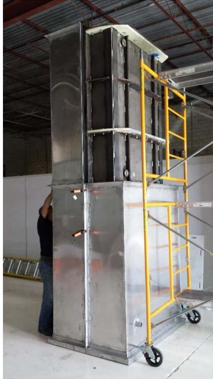
**Figure 3.23: Vacuum Can Assembly**
