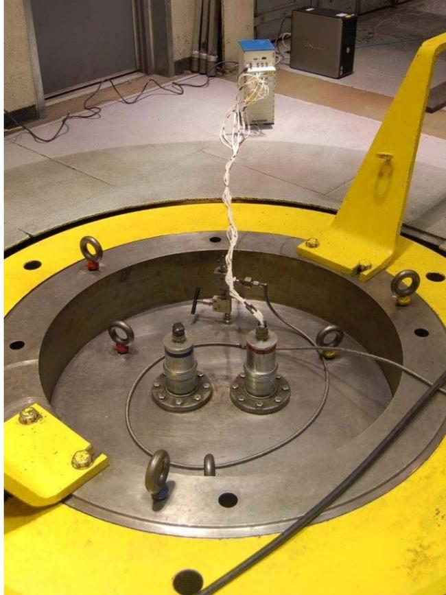
**Figure 3.13: Final Closure Complete. Through-wall Connectors Attached to Data Acquisition System**
