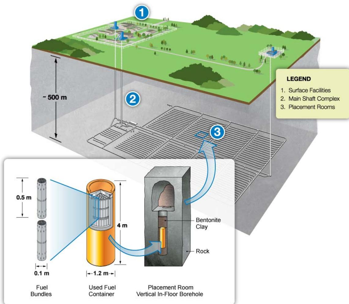
**Figure 1.1: Illustration of a Deep Geological Repository – In-floor Borehole Placement (Mark I Design)**
