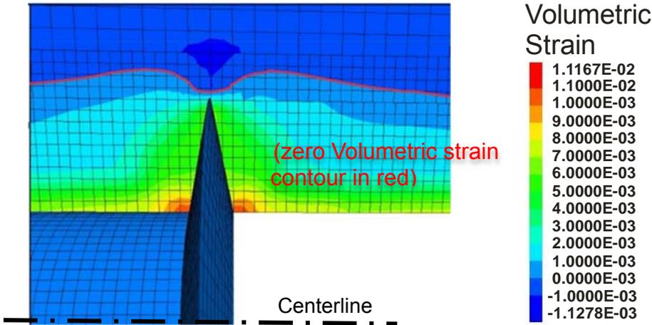
**Figure 4.2: Contours of volumetric strain around a triangular cut-off seal (T/D ratio of 1:3). The transition from extension (inner EDZ) to contract (outer EDZ) is indicated by the red line.**
