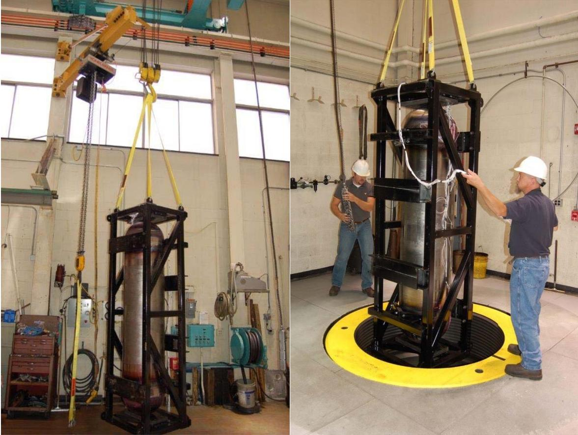
**Figure 3.10: Vertical Orientation and Emplacement Into The Pressure Vessel**
