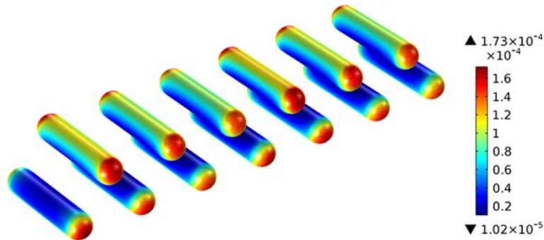
**Figure 3.30: Flux of Sulphide in mol/m<sup>2</sup>/year at the Container Surface Using a Generic Concentration of 3 ppm Sulphide at the Host Rock-bentonite Interface**
