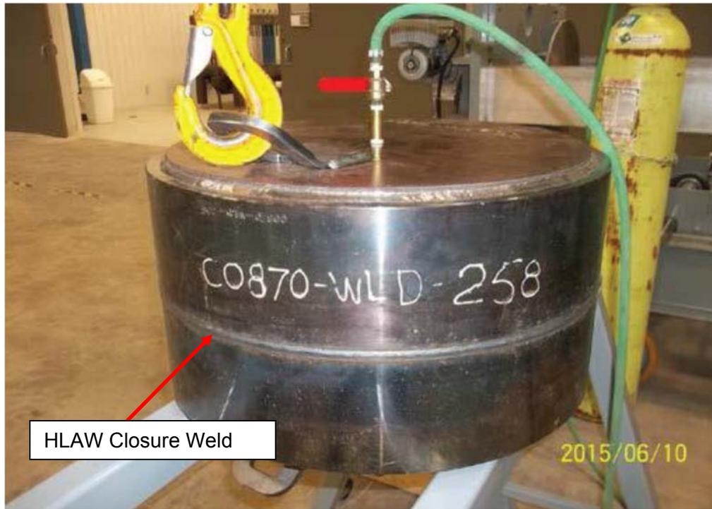
**Figure 3.4: Helium Pressurizing of UFC Closure Weld Mock-up Assembly**
