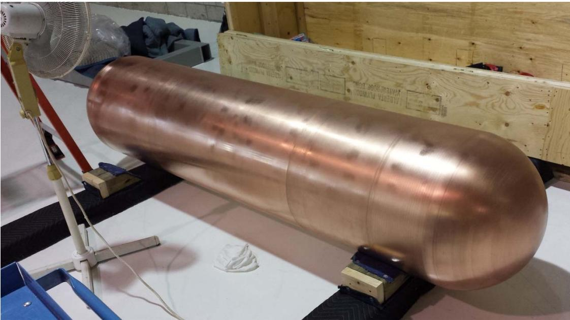
**Figure 3.2: Leading Copper Coated Mark 2 Used Fuel Container**
