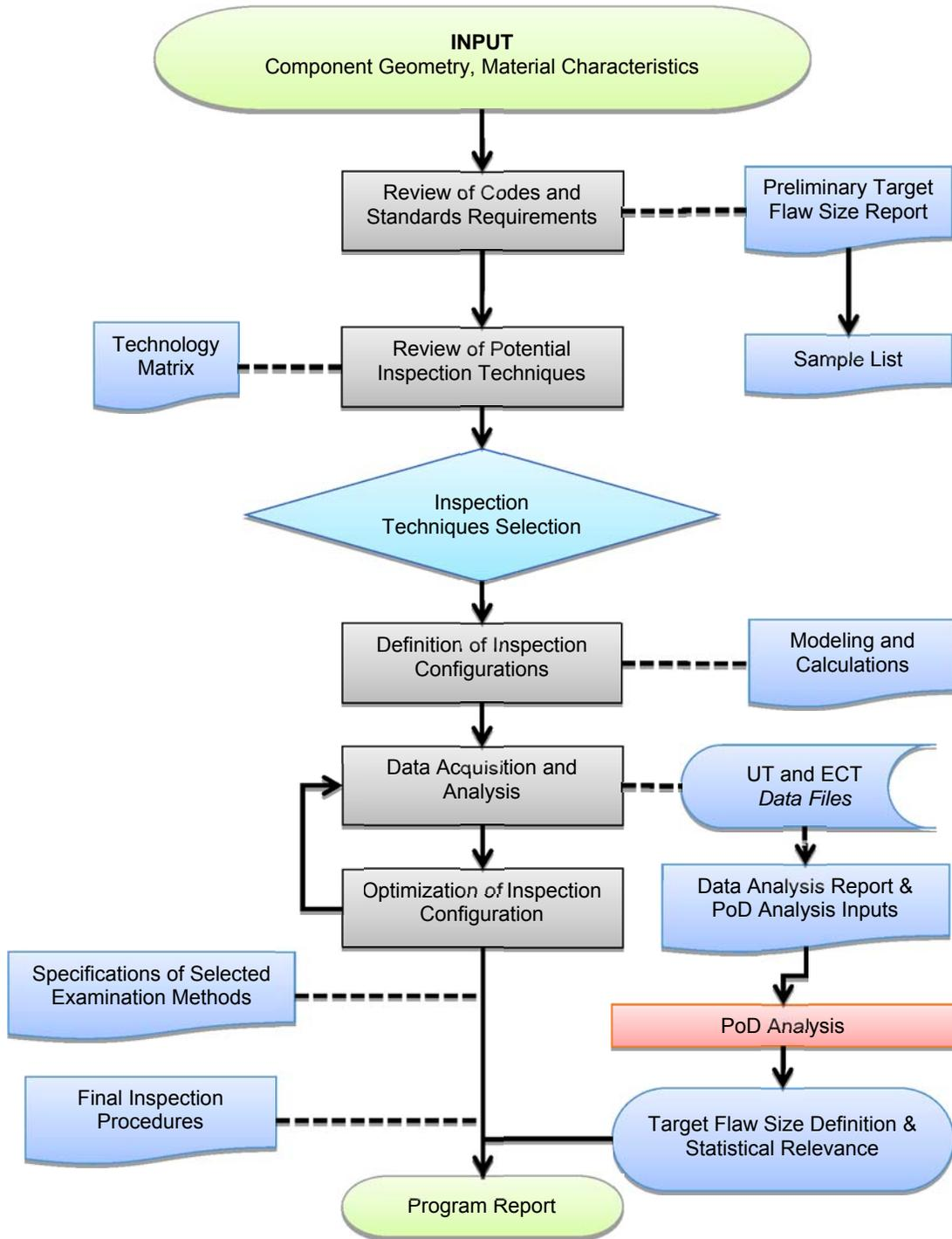
**Figure 3.5: Design Development Process Flowsheet for Non-Destructive Examination program**
