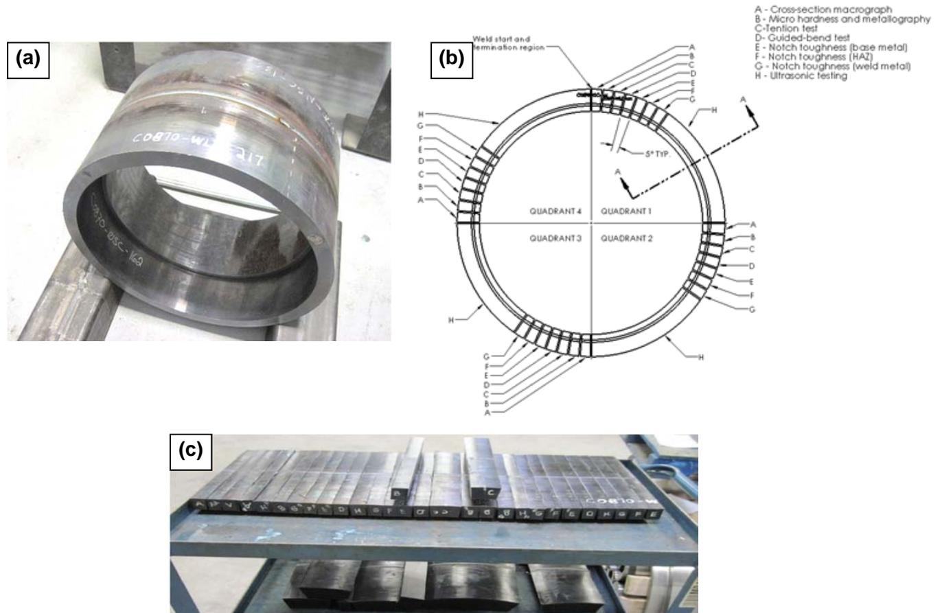
**Figure 3.3: (a) UFC Closure Weld Mock-up Assembly Simulating Shell-to-Head Geometry for WPS/PQR Testing, (b) Sampling Locations and (c) Coupons for Mechanical/metallurgical Tests**
