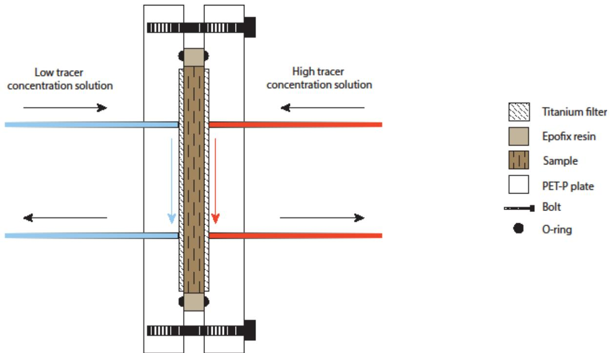
**Figure 4.18: Cross-Section View of the Diffusion Cell. The Diffusion Cell Comprised Two Plates Consisting Of Ertalyte<sup>®</sup>, An Unreinforced Polyester Based on Polyethylene Terephthalate (PET-P). Titanium Filters were Implemented in the Plates (Diameter = 0.065m; Thickness = 0.0012m; Pore Diameter =  $1 \times 10^{-5}$ m). The Solution in the Low Tracer Concentration Container is Replaced Regularly to Maintain the Concentration Gradient Driving Diffusion (Wigger et al. 2016)**
