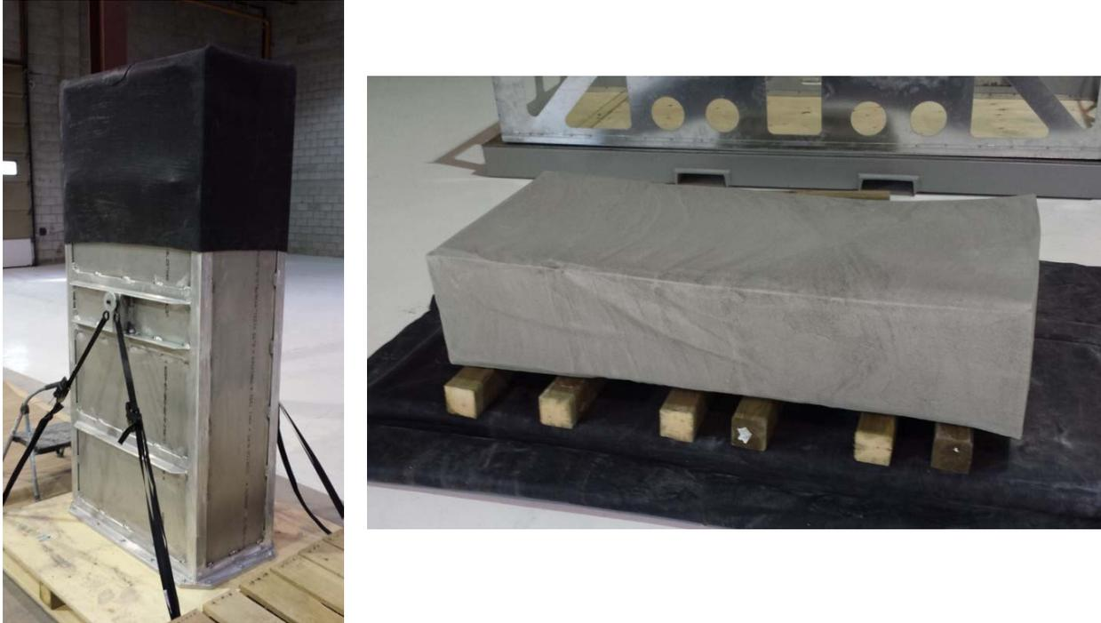
**Figure 3.21: a) Isostatic Bag and Container (left) and b) Highly Compacted Bentonite Block (right)**
