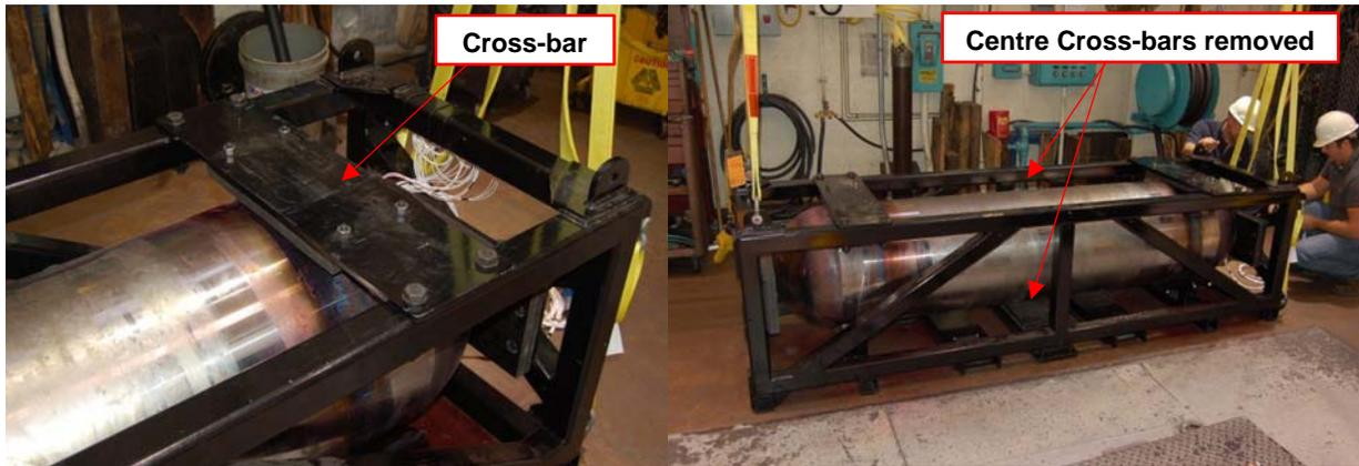
**Figure 3.8: Used Fuel Container Fixture Configured for Testing**
