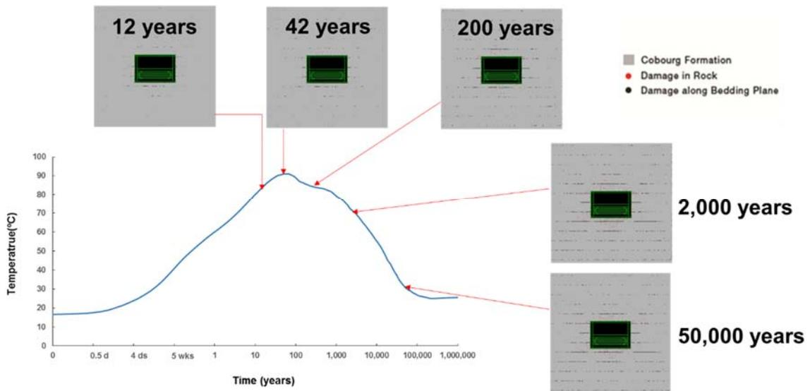
**Figure 4.3: Evolution of Damage in Sedimentary Rock**
