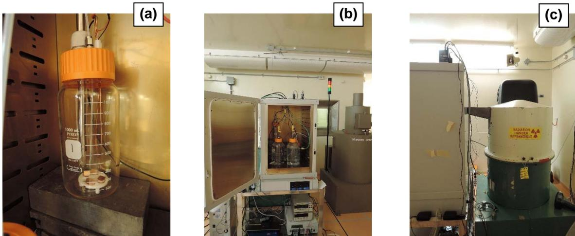
**Figure 3.19: Vapour Phase Copper Radiolysis Cell Showing (a) Copper Samples at the Base of the Sample Vessel (b) Sample Vessels Loaded Into Exposure Oven and (c) Radiation Source at the Back of the Oven**
