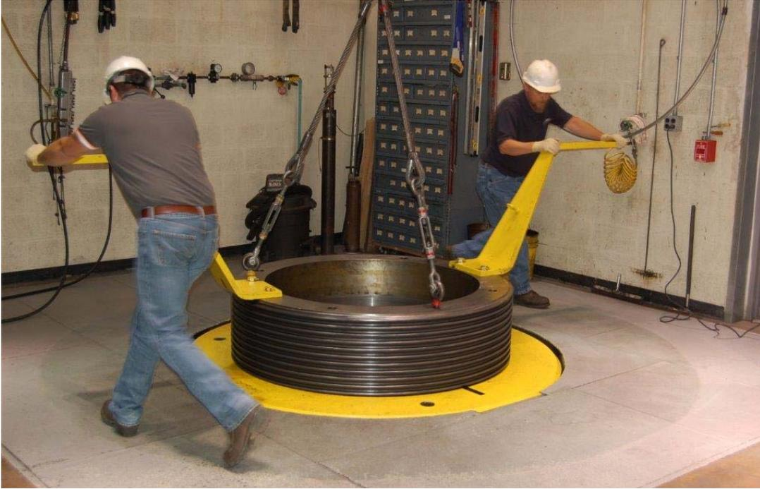
**Figure 3.12: Lid Retaining Ring Installed**
