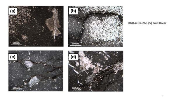
Figure 4.12: Petrographic Features of the Gull River Formation. (a) PPL of the Internodule Matrix and the Intra-nodule Fine Crystalline Dolomite. Note Also the Coarse Dolomite Filling Fracture. (b) PPL of Medium Crystalline, Euhedral Intra-nodule Dolomite. (c) Nodular Facies with Micritic Matrix Cut with Stylolites (black fractures). (d) Selective Dolomitization in the Matrix and Associated with Stylolites
