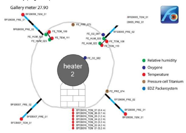
Figure 4.23: Layout of Instruments Around Heater 2 (middle; Garitte 2016)
