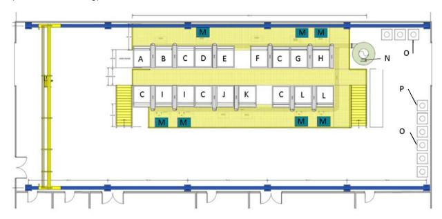
Figure 3.15: Layout of an Optimized Electroplating Pilot Cell Facility for Copper Coating UFC's: (A) Hot Rinse, (B) Soak Clean, (C) Spray Rinse, (D) Electroclean, (E) Immersion Rinse, (F) Pickle [acid salts], (G) Electropolish, (H) Nickel Strike, (I) Copper Plate [Nanovate], (J) Microetch, (K) H2So<sub>4</sub> Dip, (L) Cyanide Copper Plate, (M) Rectifier, (N) Vertical Scrubber, (O) Process Chemicals Tote, (P) Wastewater Tote
