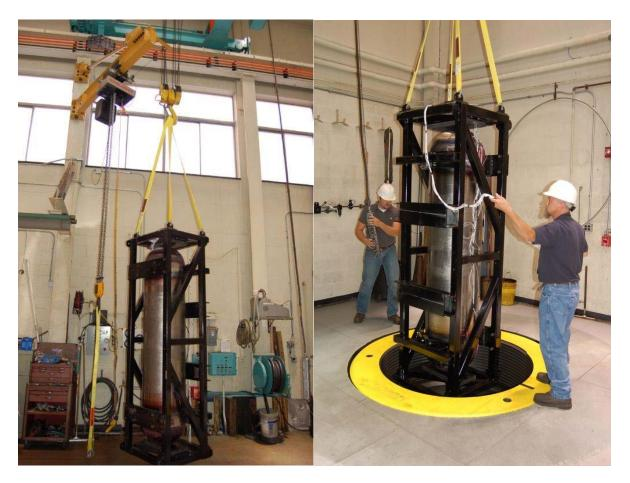
Figure 3.10: Vertical Orientation and Emplacement Into The Pressure Vessel
