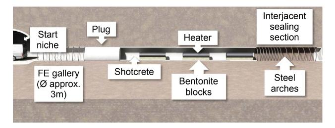
Figure 4.22: Visualization of Final Arrangement of FE Experiment at Mont Terri Rock Laboratory (Vogt 2013)
