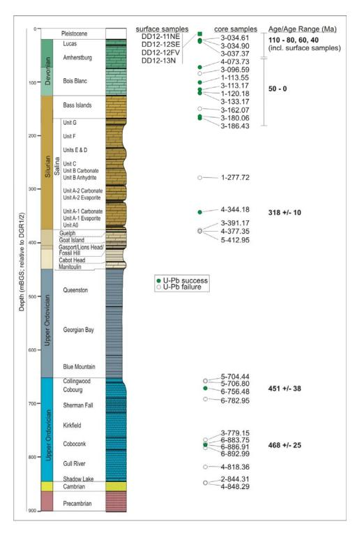
Figure 4.13: Sample Numbers, Locations and Ages Obtained In Relation to the Paleozoic Stratigraphy Beneath the Bruce Nuclear Site for Secondary Calcite Analysed by Davis Between 2013 and 2015. Samples for which U-Pb Geochronology was Successful are Green-Filled and Unsuccessful Samples are White.
