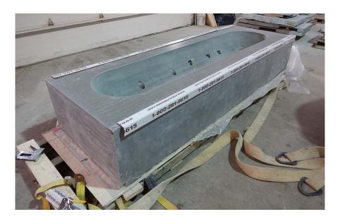
Figure 3.27: Full Size HCB Block Shaping Trial
