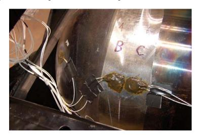
Figure 3.9: Strain Gauges Potted Onto the Used Fuel Container (UFC) at Closure Weld Location
