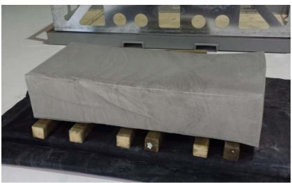
Figure 3.21: a) Isostatic Bag and Container (left) and b) Highly Compacted Bentonite Block (right)
