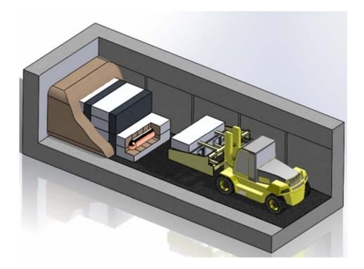
Figure 3.31: Illustration of Revised Concept Showing Direct Stacking of Buffer Box
