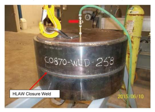
Figure 3.4: Helium Pressurizing of UFC Closure Weld Mock-up Assembly
