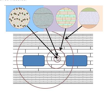
Figure 4.5: An Illustration Showing the Transition From Intact (GBM) to a Bedded-Jointed Rock Mass (DFN) with Increasing Sample Size
