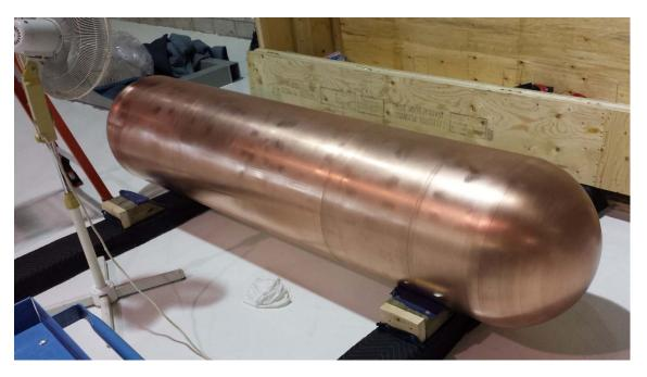
Figure 3.2: Leading Copper Coated Mark 2 Used Fuel Container
