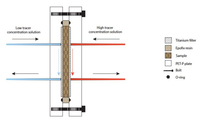
Figure 4.18: Cross-Section View of the Diffusion Cell. The Diffusion Cell Comprised Two Plates Consisting Of Ertalyte®, An Unreinforced Polyester Based on Polyethylene Terephthalate (PET-P). Titanium Filters were Implemented in the Plates (Diameter = 0.065m; Thickness = 0.0012m; Pore Diameter = 1x10<sup>-5</sup>m). The Solution in the Low Tracer Concentration Container is Replaced Regularly to Maintain the Concentration Gradient Driving Diffusion (Wigger et al. 2016)
