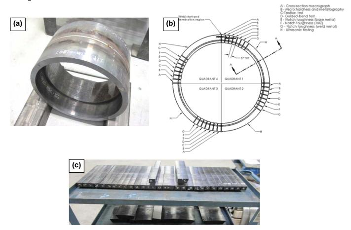
Figure 3.3: (a) UFC Closure Weld Mock-up Assembly Simulating Shell-to-Head Geometry for WPS/PQR Testing, (b) Sampling Locations and (c) Coupons for Mechanical/metallurgical Tests
