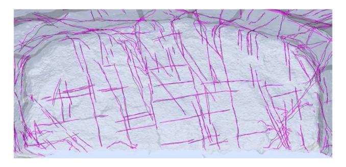
Figure 4.27: Comparison of Field and Generated Fracture Traces for Tunnel Wall
