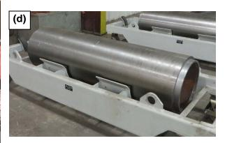
Figure 3.7: Mark 2 Steel Shell and Hemi-Head Components Fabricated as Part of UFC Machining Program. Hemi-head in (a) as-formed Condition and (b), After Intermediate Machining Step. Shell During Machining (c) and, (d) in Final Configuration
