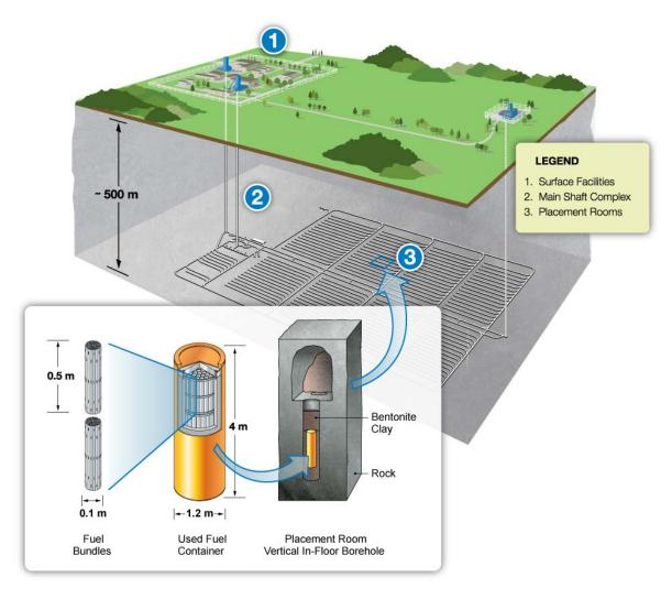
Figure 1.1: Illustration of a Deep Geological Repository – In-floor Borehole Placement (Mark I Design)
