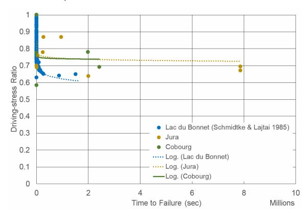
Figure 4.1: Comparison of Time-to-Failure Results from Static Fatigue Testing on the Lac du Bonnet Granite, the Jura Limestone and the Cobourg Limestone
