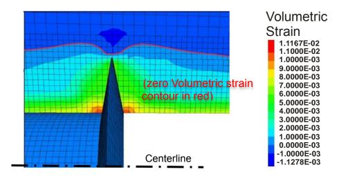
Figure 4.2: Contours of volumetric strain around a triangular cut-off seal (T/D ratio of 1:3). The transition from extension (inner EDZ) to contract (outer EDZ) is indicated by the red line.
