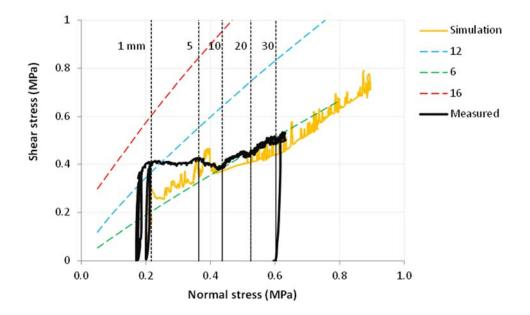
Figure 4.9: Shear vs Normal Stress Plot, with Theoretical Peak Shear Strength Envelopes for Joint Roughness Coefficient (JRC)'s of 6, 12 and 16 Illustrated as Green, Blue and Red Dashed Lines, Respectively. Measured Values are Plotted as a Solid Black Line and the Model Simulation from the Unmated Model in Gold
