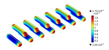
Figure 3.30: Flux of Sulphide in mol/m²/year at the Container Surface Using a Generic Concentration of 3 ppm Sulphide at the Host Rock-bentonite Interface
