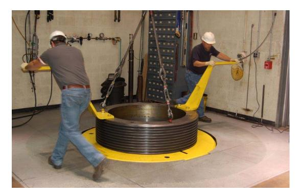
Figure 3.12: Lid Retaining Ring Installed
