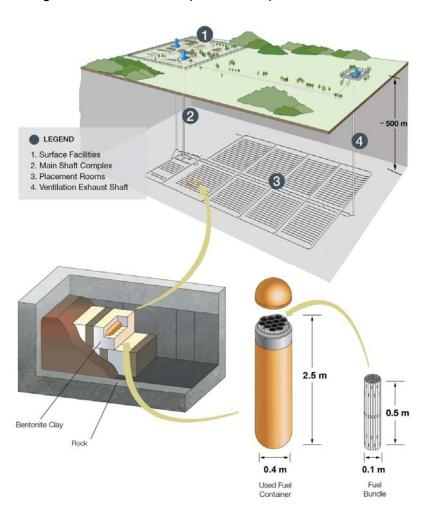
Figure 1.2: Illustration of a Deep Geological Repository – Horizontal Placement (Mark II Design)
