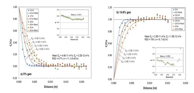
Figure 4.14: Tracer Diffusion Data for a) Fully Brine-saturated and b) Partially Brine-Saturated Samples of Queenston Formation Shale. Note the 53% Decrease in D<sub>e</sub> for lodide that is Observed for Partially Saturated Conditions (14.6% gas, 85.4% brine)
