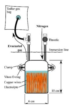
Figure 3.18: Schematic of The Experimental Cell Used for Sensor-monitored Experiments
