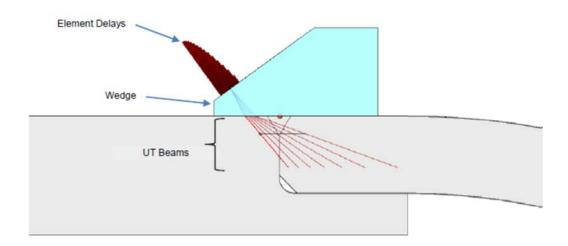
Figure 3.6: Beam Simulation of Shear Wave Phased-Array-Ultrasonic-Testing (PAUT) Applied to Mark 2 Closure Weld / Joint Configuration
