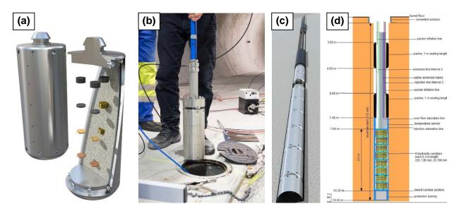
Figure 3.29: Materials Corrosion Test at the Grimsel Underground Research Laboratory Illustrating (a) Copper and Steel Corrosion Coupons in Bentonite (b) Insertion/removal of Borehole Module and Series of Modules Within the Borehole as (c) Cartoon and (d) Schematic Showing Depths and Packers
