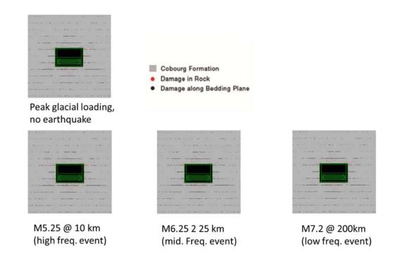
Figure 4.4: Microcracks in the Rock at Peak Glacial Load Subjected to Three Different Earthquakes at 10<sup>-6</sup> p.a. Probability Level in Sedimentary Rock
