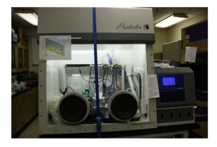
Figure 4.16: Glove Box with Controlled O<sub>2</sub> Concentration (<1.0 ppm) for Sorption Tests Under Reducing Conditions
