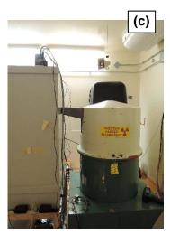
Figure 3.19: Vapour Phase Copper Radiolysis Cell Showing (a) Copper Samples at the Base of the Sample Vessel (b) Sample Vessels Loaded Into Exposure Oven and (c) Radiation Source at the Back of the Oven
