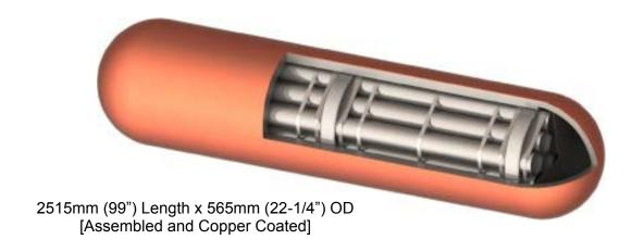
Figure 3.1: Illustration of NWMO's Mark 2 Used Fuel Container Consisting of Steel Containment (core), External Copper Coating and Internal Fuel Baskets
