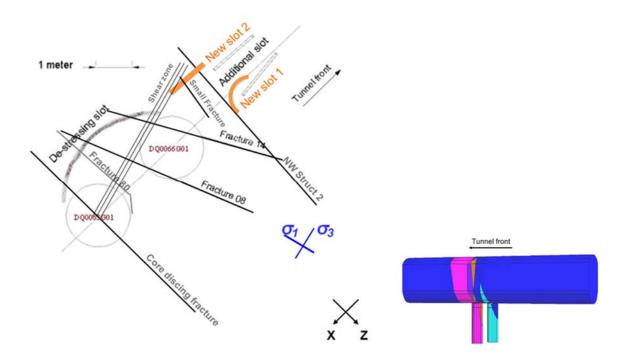
Figure 4.7: Proposed Insitu Shear Test Setup for Äspö TASQ Tunnel Using Slot Drilling to Activate Shear Displacements in a Vertical Fracture (NW structure 2) (Mas Ivars et al. 2015)
