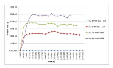
Figure 4.19: a) Effect of Ionic Strength on the Anion Accessible Porosity of Opalinus Clay and Helvetic Marl. The Accessibility is Given as Fraction of the Total Porosity; and b) Anion Diffusion Experiment on Blue Mountain Samples with Varying Ionic Strength. The Flux is Relative to the Total Tracer <sup>36</sup>Cl<sup>-</sup> Concentration in the System Plotted
