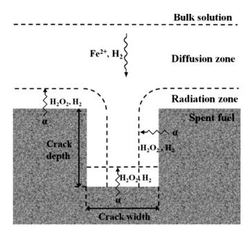
Figure 5.1: Model Arrangement Showing a Cross-section of the Fuel/solution Interface for Simulation of Radiolytic Corrosion Inside a Crack in a Fuel Pellet
