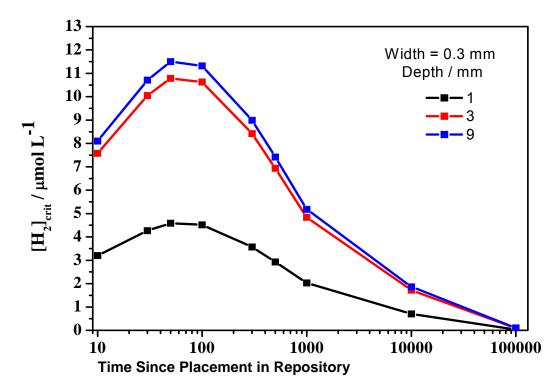
Figure 5.2: The critical  $[H_2]$  as a Function of Time Since Placement of the Fuel in the Repository for Various Crack Depths and a Crack Width of 0.3 mm.
