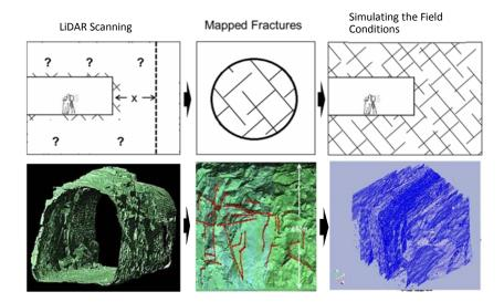
Figure 4.6: Geometric Modelling of DFNs and Their Implementation into SRM Modelling
