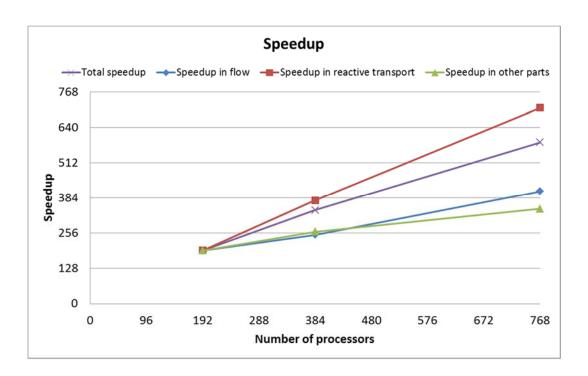
Figure 4.21: Speedup of MPI Parallel Version ParMIN3P-THCm for Flow and Reactive Transport in a Sedimentary Basin, Executed on the WestGrid Jasper Cluster, Total Degrees of Freedom is 103,680,000
