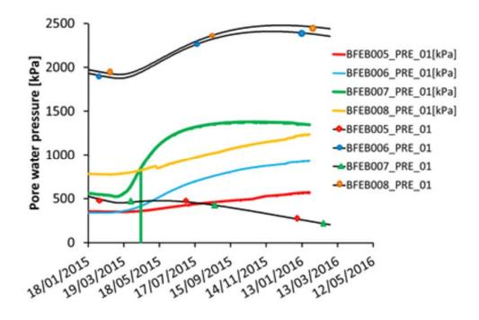
Figure 4.25: Comparison of Predicted and Measured Pore Water Pressure
