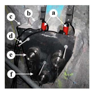
Figure 4.8: In Situ Shear Test Set up on a Fracture Associated with the BFZ300 Structure: a) Hydraulic Jacks, b) Removed Sample, c) Concrete Backfill, d) Attachment Sars, e) Anchor Bolt with Load Cell, f) Steel Loading Plate
