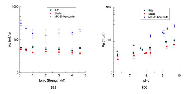
Figure 4.17: (a) Ionic Strength Dependence of Np(V)  $K_d$  Values in Highly Saline Na-Ca-CI Solutions; and (b) pH<sub>c</sub> Dependence of Np(V)  $K_d$  Values in the Na-Ca-CI (I = 4.6 M) Brine. The Initial Concentration of Np(V) was  $1.0 \times 10^{-5}$  M
