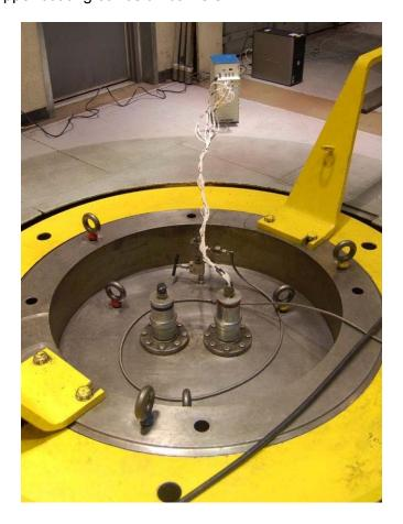
Figure 3.13: Final Closure Complete. Through-wall Connectors Attached to Data Acquisition System
