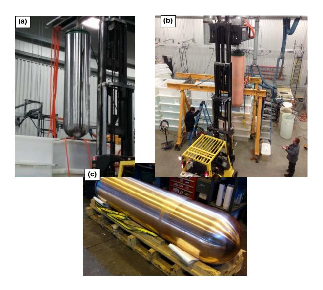
Figure 3.14: Electrodeposition of Copper on a Full-Sized UFC Lower Assembly : (a) Steel Part Being Immersed into Cleaning Solution; (b) Following Deposition of Initial Copper Layer; (c) Coated and Machined
