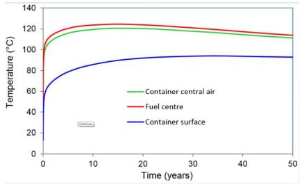
Figure 5.6: Figure 5.7: Mark II Container Temperatures in a Hypothetical Crystalline Repository
