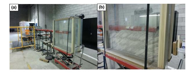
Figure 3.28: Photographs of a) Utility Auger and Test Frame and b) Utility Auger filling the 4<sup>th</sup> layer
