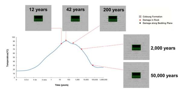
Figure 4.3: Evolution of Damage in Sedimentary Rock
