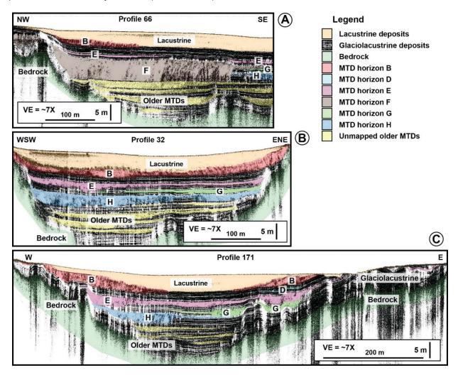
Figure 4.11: Sub Bottom Profiles of Sediments in Lac Dasserat. Six Submarine MTD Deposits Within the Lake Have Been Identified and Labelled
