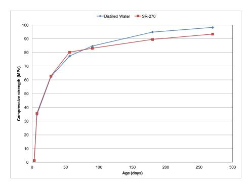
Figure 5.4: Unconfined Compressive Strength Results for LHHPC
