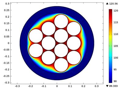
Figure 5.5: Temperature (°C) Across the Middle Section of a Mark II Container After ~15 years in a Hypothetical Crystalline Repository
