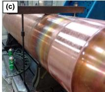
Figure 3.17: Cold Spray Copper Coating Applied to Closure Weld Region (a) Before (b) During and (c) After Machining
