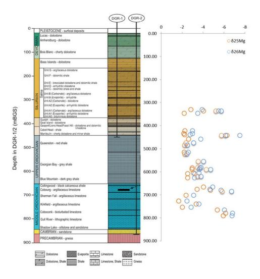
Figure 4.15: Magnesium Isotope Data for the Pore and Groundwater in the Upper Ordovician and Lower Silurian Sediments.
