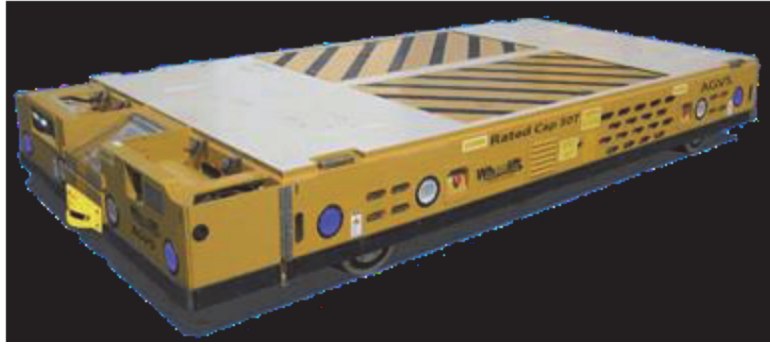
Figure 9: Example Low Profile AGV Transporter- 50 Ton Cap
