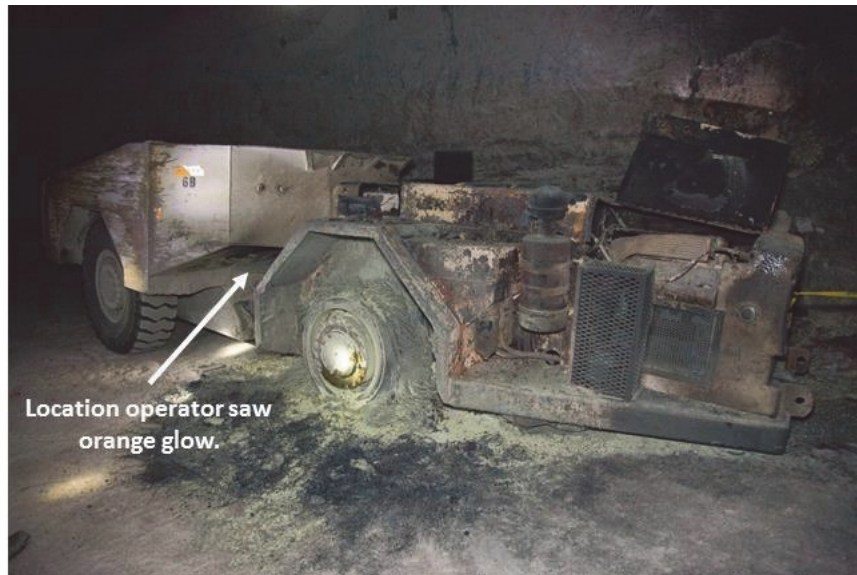
Figure 27: Burned Salt Hauler Involved in the WIPP Fire
