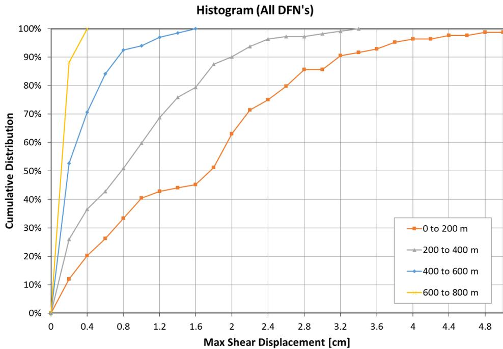
**Figure 4-34: Cumulative Distributions of Shear Displacement For All DFNs For a Magnitude M6.1 Earthquake and a 40° Dipping Fault**
