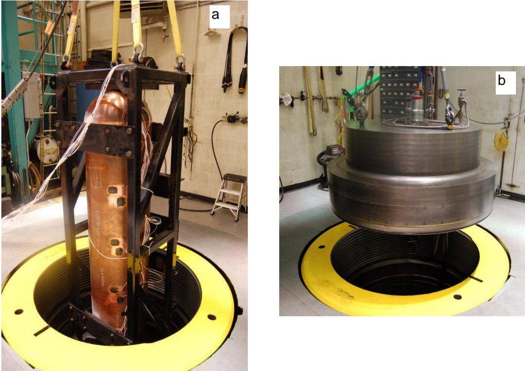
**Figure 3-16: Copper Coated UFC Being Lowered into the External Pressure Test Vessel (a) at Penn State and Pressure Test Vessel Lid Applied (b)**
