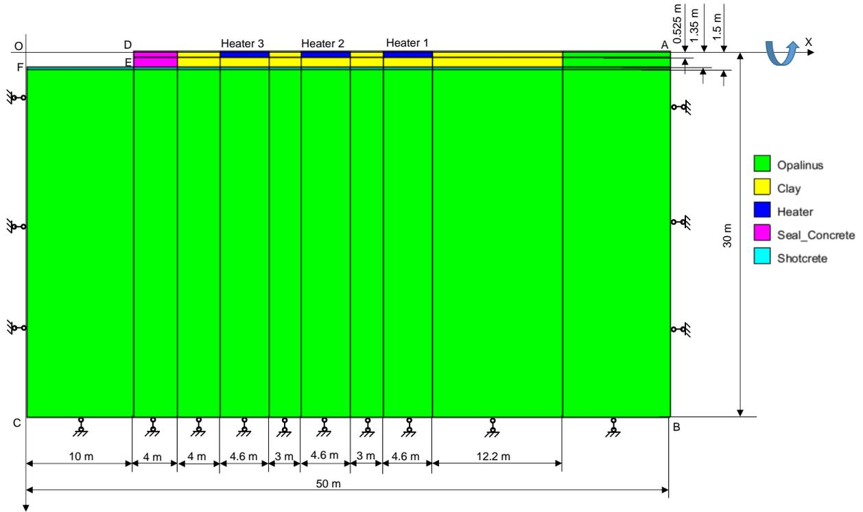
Figure 4-23: Two-Dimensional Axial-Symmetric Model of FE Experiment
