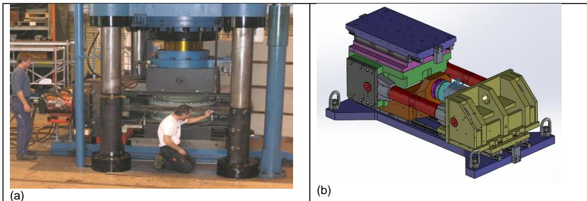
**Figure 4-10: Large Capacity Four-column Load Frame With Maximum Normal Capacity of 20 MPa and Maximum Height of 4 m, Research Institute of Sweden; (b) Conceptual Design of Large-scale Shear Box**
