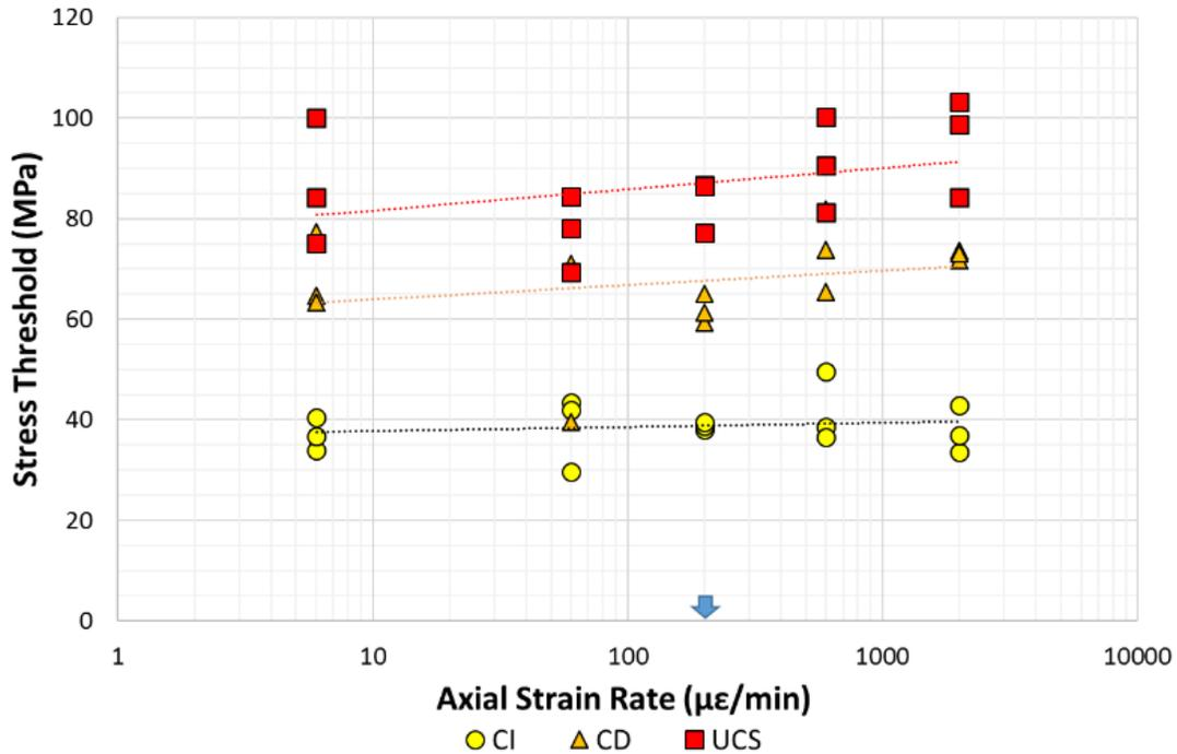
**Figure 4-21: Comparison of CI, CD, and UCS Stress Thresholds with Respect to Axial Strain Rate for One Month Saturated Specimens. Blue Arrow Represents Standard Axial Strain Rate Used in Saturation and Scaling Studies**
