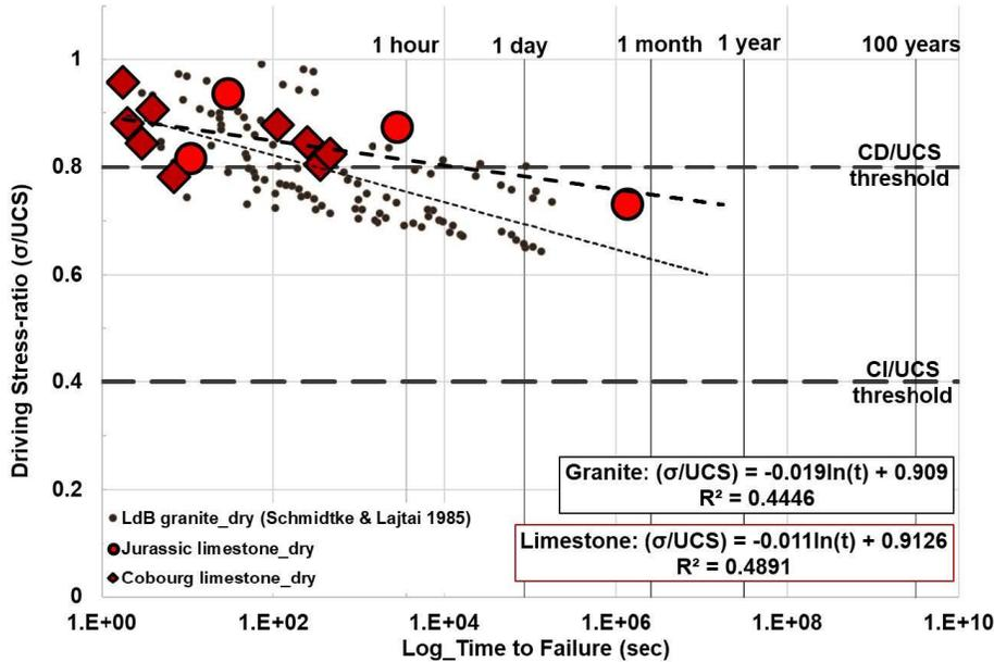
Figure 4-16: Comparison of Static Load Creep Test Data on Limestone and Granite Performed at Room Temperature in Dry Conditions
