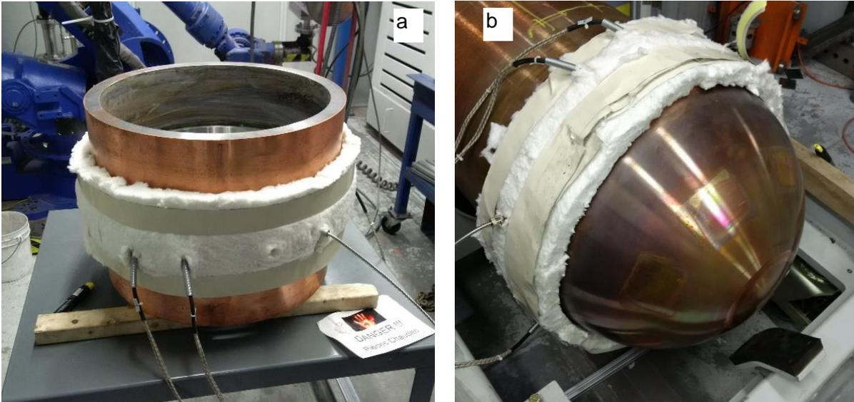
**Figure 3-13: Application of Heat Band Treatment Technique to Short Pipe Segments during Optimization (a) and the UFC to be Used for External Pressure Testing (b)**
