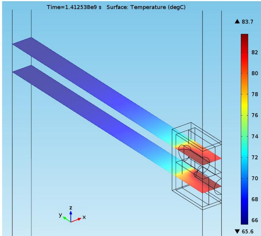
**Figure 5-7: Temperatures in the Rock along the Horizontal Cross-sections Through the Container Axis at Time of 45 Years after Placement**
