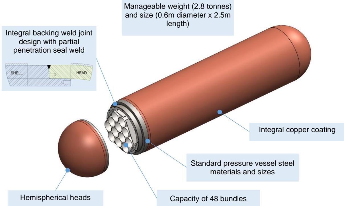
**Figure 3-5: Illustration of Used Fuel Container with Design Features Identified**
