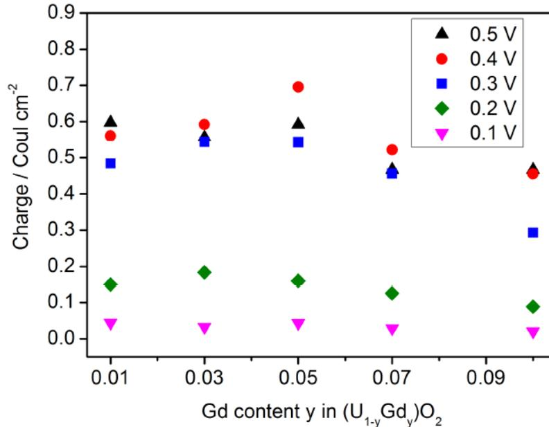
**Figure 5-2: Total Anodic Charge Obtained by Integrating Current Measured Potentiostatically for One Hour on  $(U_{1-y}Gd_y)O_2$  Electrodes at Different Potential in Solution Containing 0.05 mol/L Carbonate/ Bicarbonate**
