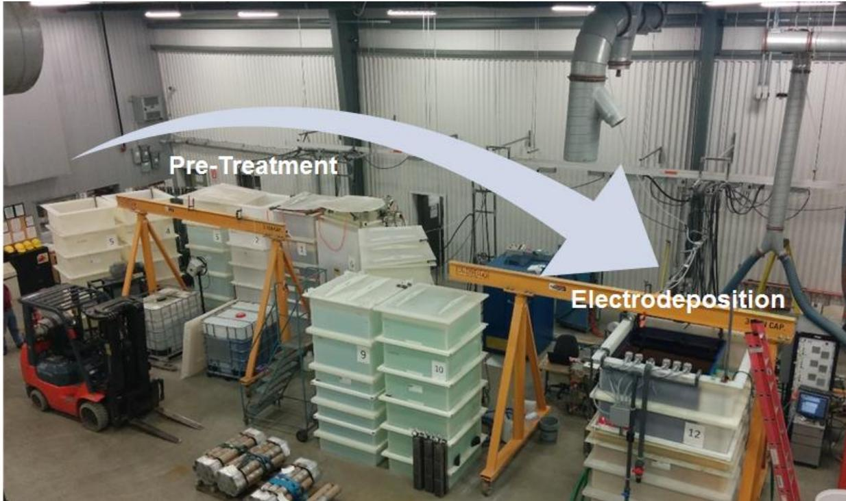
**Figure 3-8: Proof-of-concept Line Consisting of Pre-treatment and Electrodeposition Process Tanks**
