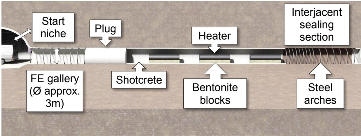
Figure 4-22: Visualization of Final Arrangement of FE Experiment at Mont Terri Rock Laboratory (Vogt, 2013)
