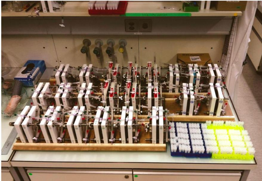
**Figure 4-1: a) Schematic of Confining Cell for Saturation Component of the Benchmarking Experiment; Fluid of Known Composition is Injected at the Inlet. b) Experimental Set-up – Edges of the Core Discs are Sealed in Resin, in Addition to the Presence of Sealing Rings – Maintains Closed-system Conditions during Saturation**
