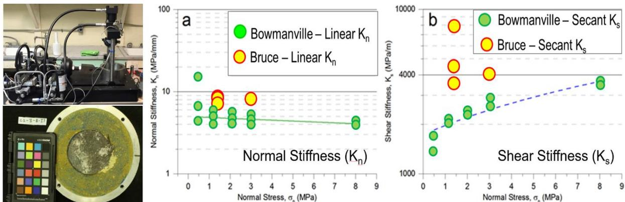
**Figure 4-14: Servo Controlled Direct Shear Apparatus at Queen's University; (a) Normal and (b) Shear Stiffness Measurements from Two Different Limestones**
