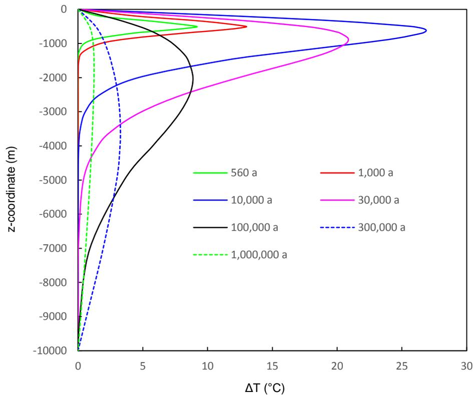
**Figure 5-5: Temperature Difference Profiles along Vertical Line through Panel Centre between the Simplified Near-Field Model and the Far-field Model**
