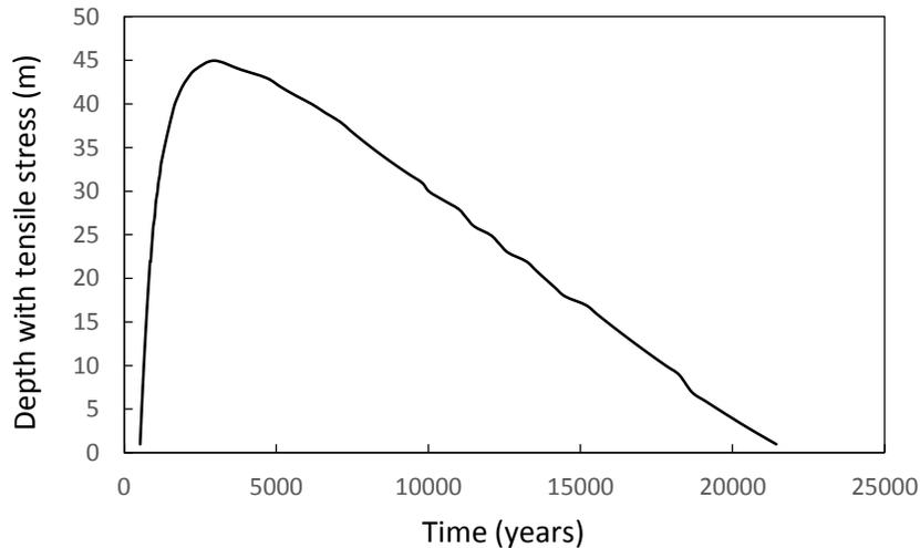
**Figure 5-11: Tensile Stress Depth in Rock for the Case with the 150 m Top Layer of Rock Fractured**
