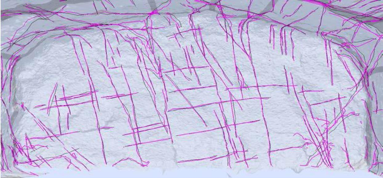
**Figure 4-17: Comparison of Field (grey) and Generated Fracture (pink) Traces for Tunnel Wall**
