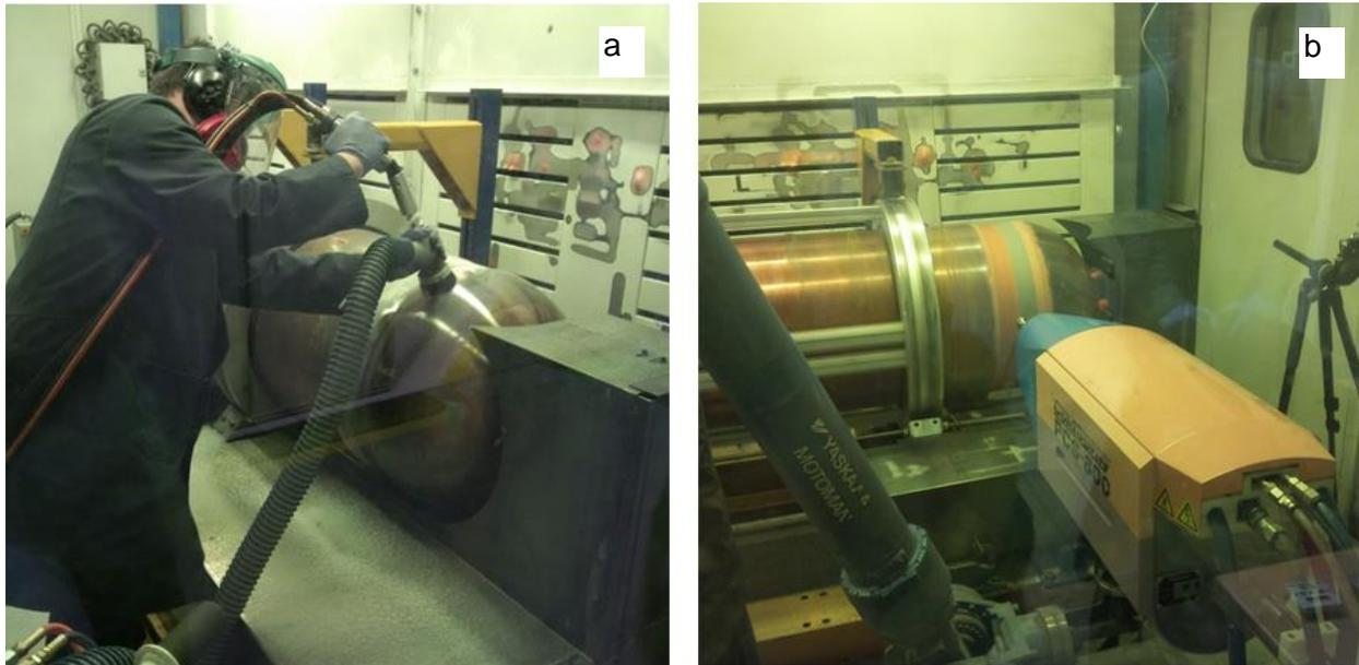
**Figure 3-12: Cold Spray of the UFC's – Grit Blasting to Remove Scale (a) and the Application of Cold Spray Copper to the Closure Weld Zone (b)**
