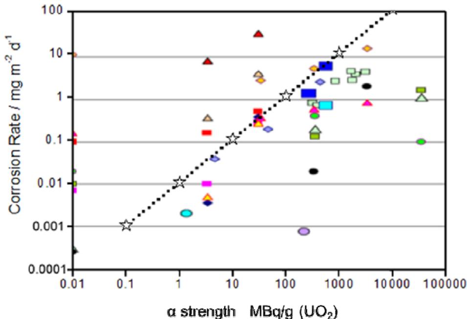
**Figure 5-1: Comparison of Experimental Corrosion Rates from Poinssot et al. (2005) with Model Simulation Results (stars)**
