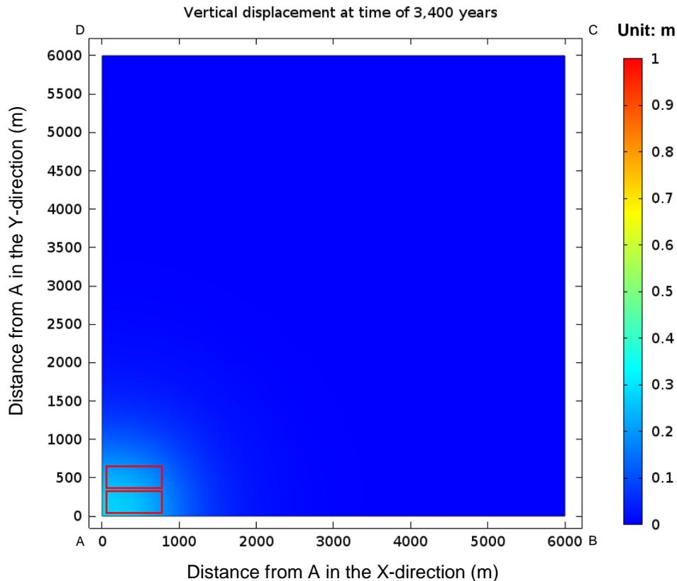
**Figure 5-9: Vertical Displacement of the Ground Surface after 3,400 Years**
