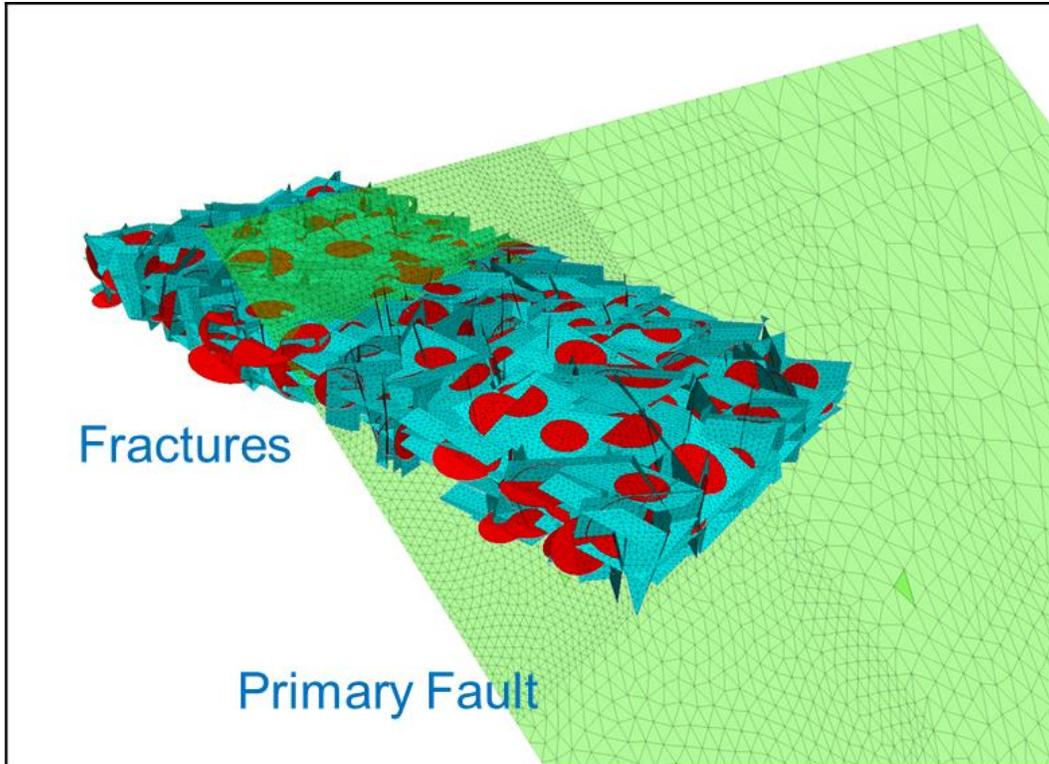
**Figure 4-32: Fault Rupturing Model Showing a 40° Dipping Primary Fault and Discrete Fracture Network Along Repository Horizon**
