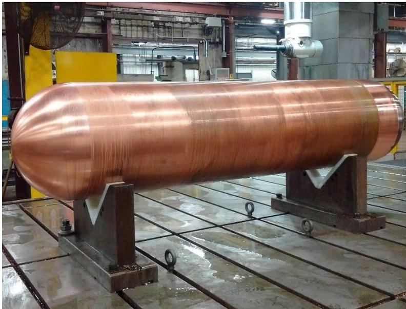
**Figure 3-6: Prototype Used Fuel Container after Final Machining**
