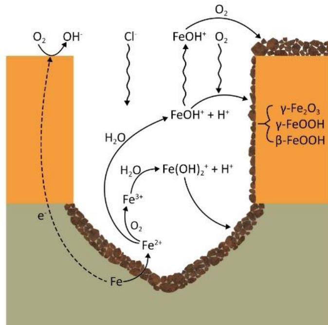
**Figure 3-18: Schematic Illustration of the Chemistry Inside a Coating Defect during Corrosion in an  $O_2$ -purged  $3 \text{ mol L}^{-1} \text{ NaCl}$  Solution**
