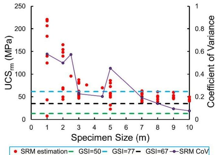
**Figure 4-13: Compressive Strength Obtained from SRM Simulations and Hoek-Brown Criterion for Different Specimen Sizes [Note: Input GSI parameter in the Hoek-Brown criterion was estimated based on the average block volume, mean joint spacing and RQD measured in the Brockville site (Farahmand 2017)]**
