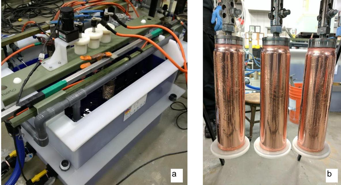
**Figure 3-11: Small-scale Tank for Tolerance Studies (a) and Coupons to be Used for Testing (b)**
