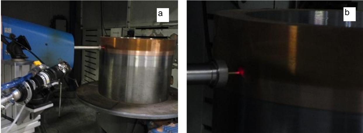
**Figure 3-15: Implementation of the Robot-assisted Laser for Pre-heat or Surface Conditioning (a) and Close-up of Laser Spot on the Surface (b)**
