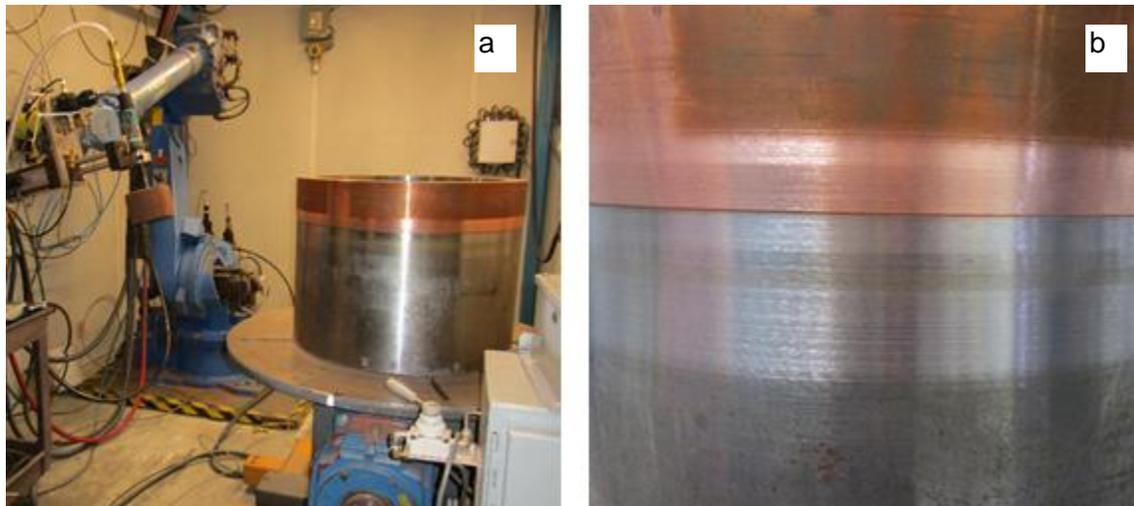
**Figure 3-14: Implementation of the Robot-assisted Mechanical Abrasion Tool (a) and Resulting Surface after Removing Scale (b)**
