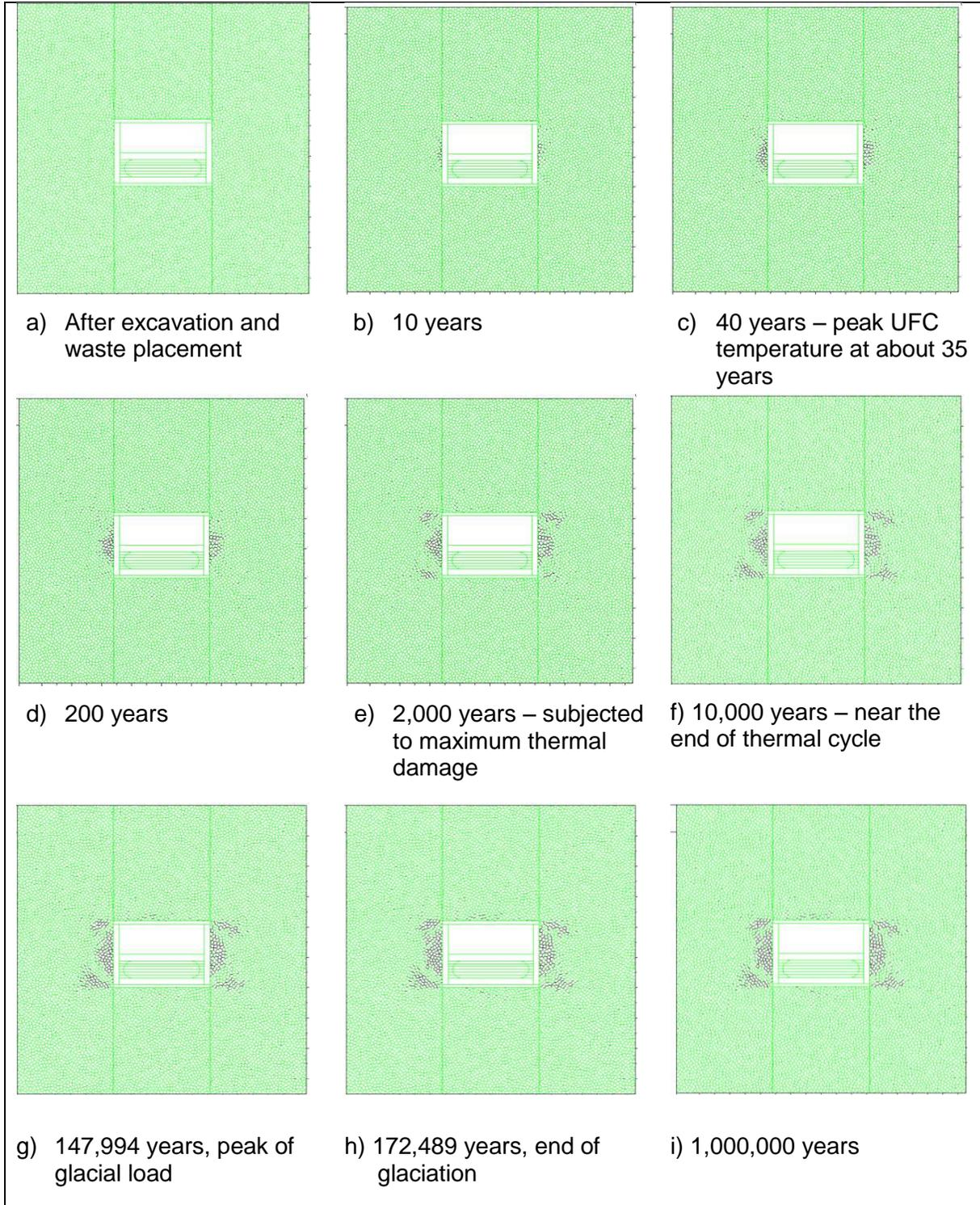
**Note:** (1) Black markings indicate microcrack/damage and (2) Placement room dimension: 3.2 m (W) x 2.2 m (H)
