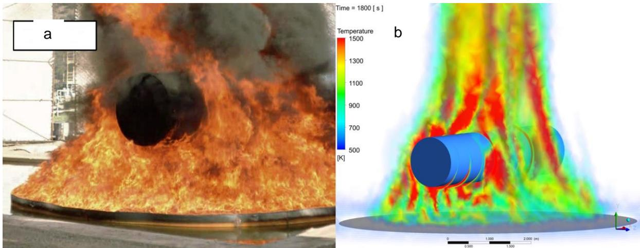
**Figure 3-4: Simulating (a) Real-world Fire Test with (b) CFD Combustion Simulation**
