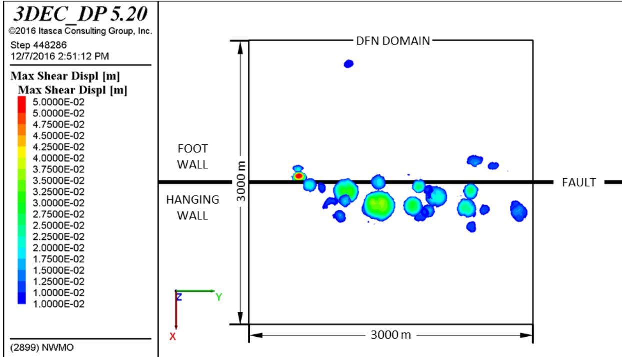
**Figure 4-33: Fracture Shear Displacements in DFN 001. This Image Depicts a M6.1 Earthquake, with a 40° Dipping Fault. The Maximum Fracture Shear Displacement is 4.8 cm (fractures with shear displacement less than 1 cm are not shown)**
