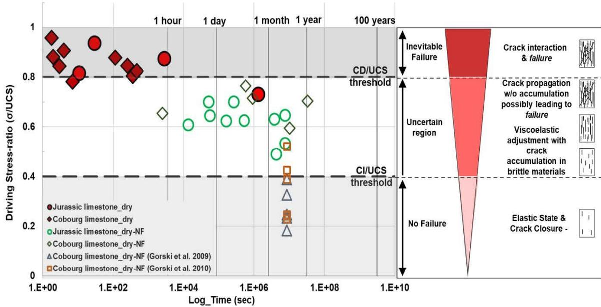
Figure 4-15: Static Load Creep Test of Jurassic and Cobourg Limestone Performed in Dry Conditions (The 'NF' in the legend indicates samples or tests did not fail)
