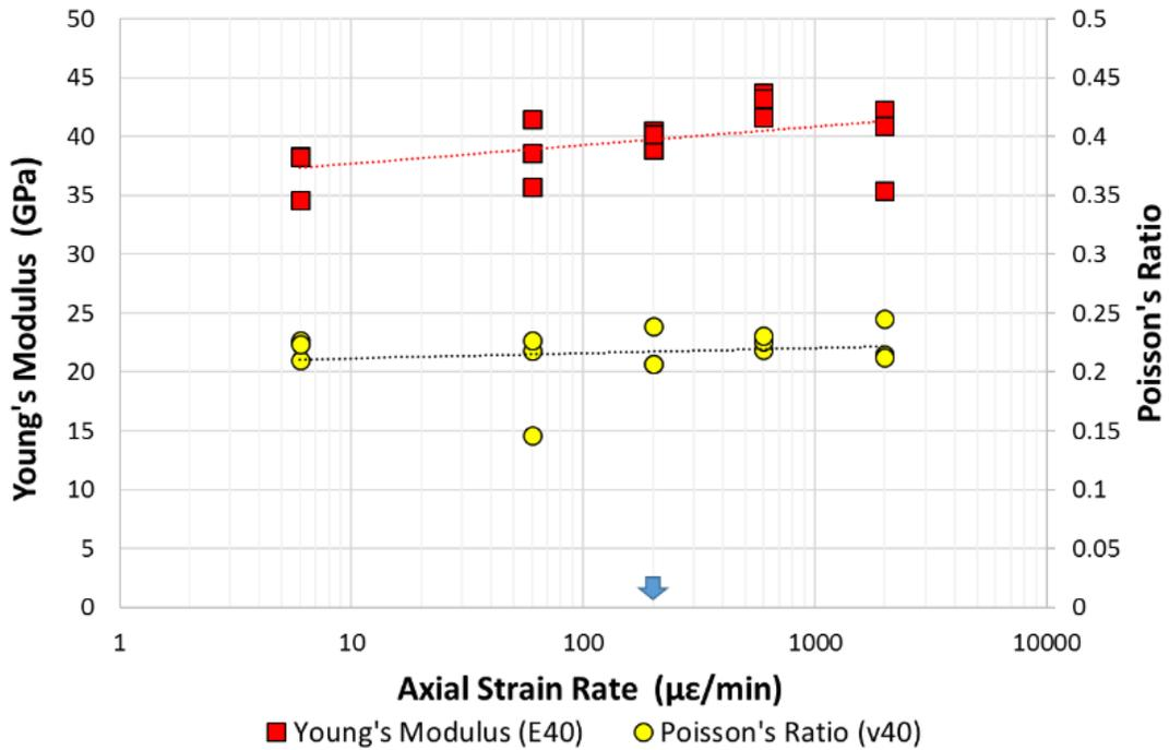
Figure 4-20: Poisson's Ratio and Young's Modulus Versus Axial Strain Rate for RRH. Blue Arrow Represents Standard Axial Strain Rate Used in Saturation and Scaling Studies
