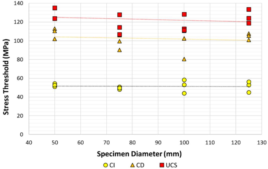
Figure 4-19: Comparison of CI, CD, and UCS Stress Thresholds with Respect to Specimen Diameter
