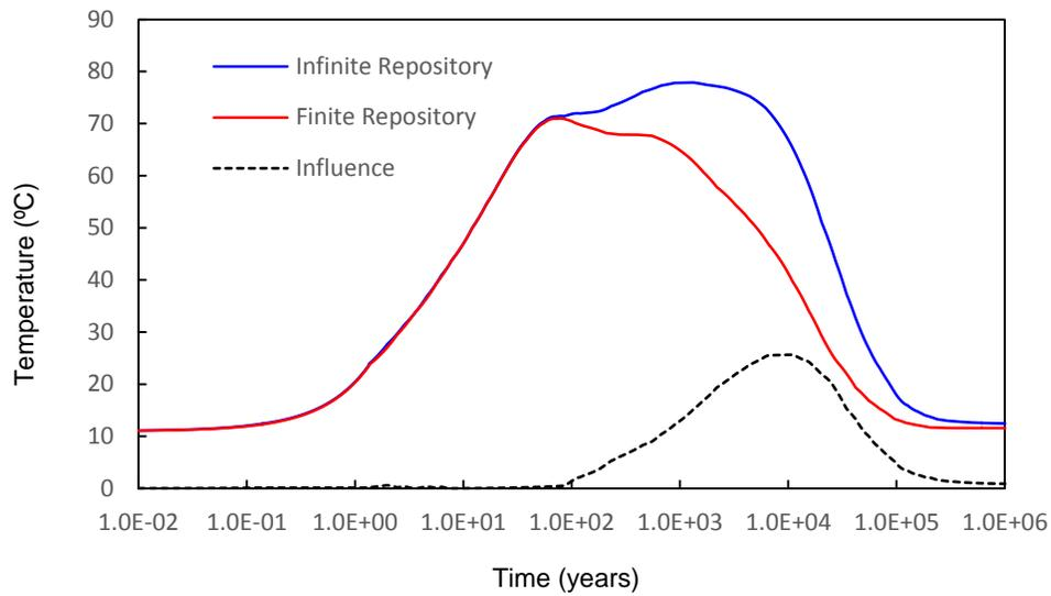
**Figure 5-4: Temperature at Panel Centre from the Far-field Model with Horizontally Finite-Dimensional Repository and Temperature at Repository Depth from the Simplified Near-Field Model and their Differences**
