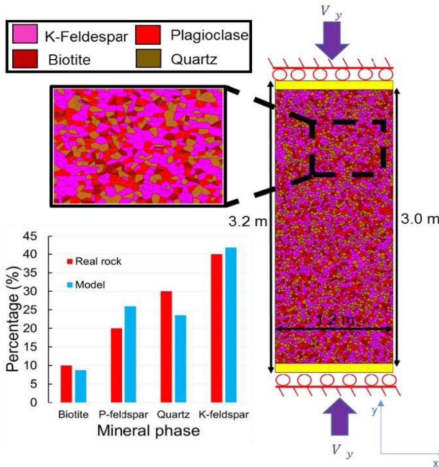
**Figure 4-11: SRM Model for an Unconfined Compression (UCS) Test Sample. Grains with Purple, Light Red, Light Brown, and Dark Red Represent K-feldspar, Plagioclase, Feldspar, Quartz and Biotite Minerals, Respectively; Histogram Shows the Abundance of Different Mineral Phases (Farahmand 2017)**
