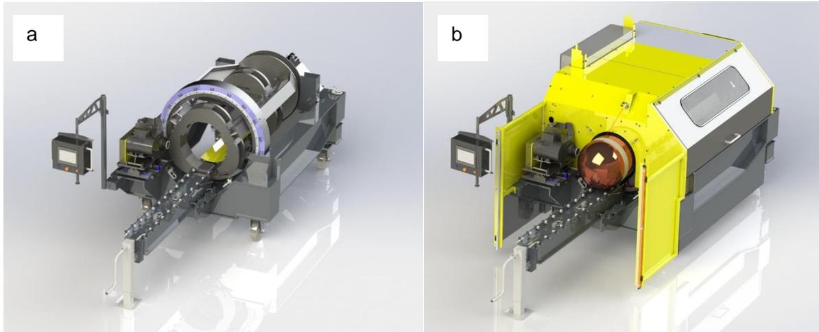
**Figure 3-7(a, b): Illustration of Second Generation Ancillary Equipment (ROTEQ 2.0) Used to Rotate UFC during Closure Welding**
