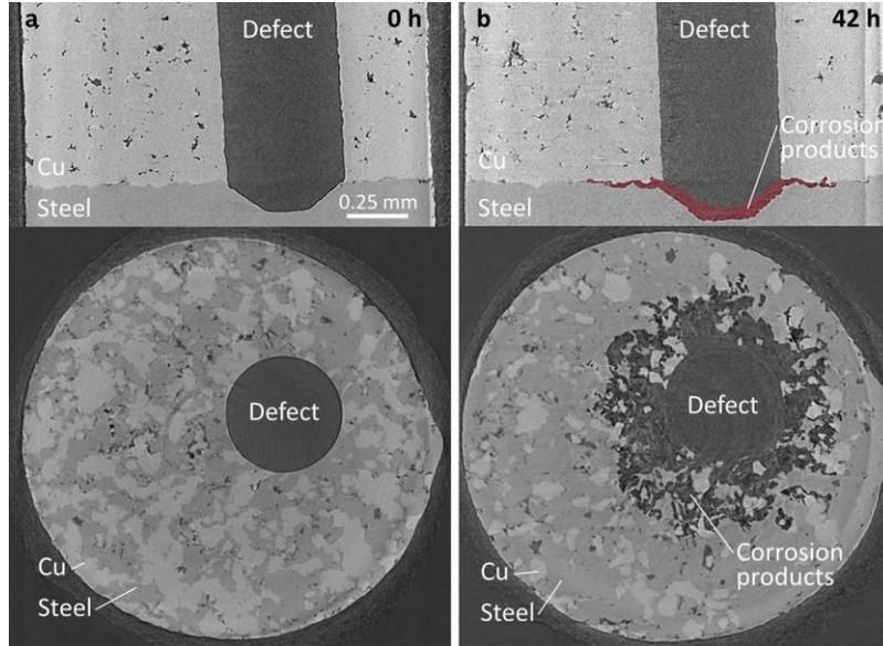
**Figure 3-19: Synchrotron Micro-CT Vertical and Horizontal Image Slices of the Cold Spray Cu/steel Interface after Exposure to O<sub>2</sub>-sparged 3 mol L<sup>-1</sup> NaCl Solution for 0 Hours (a) and 42 Hours (b). The Accumulated Corrosion Products are Highlighted in the 42 Hours Vertical Image Slice**
