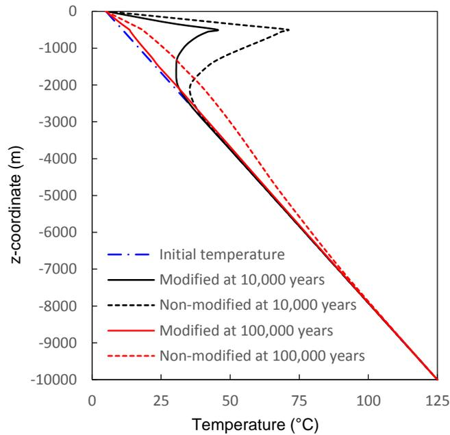
**Figure 5-8: Comparison of Modified and Non-modified Temperature after 10,000 Years and 100,000 Years from Near-field Model with Initial Temperature**
