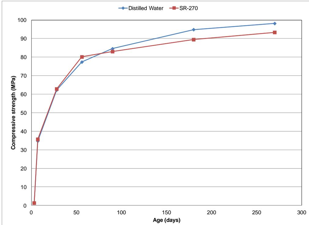
**Figure 5-3: Unconfined Compressive Strength Results for LHHPC**
