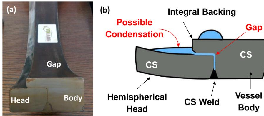
**Figure 3-17: (a) Photograph and (b) Schematic of the Cross-section of the Hemispherical Head and Vessel Body Weld Region of the Canadian UFC**
