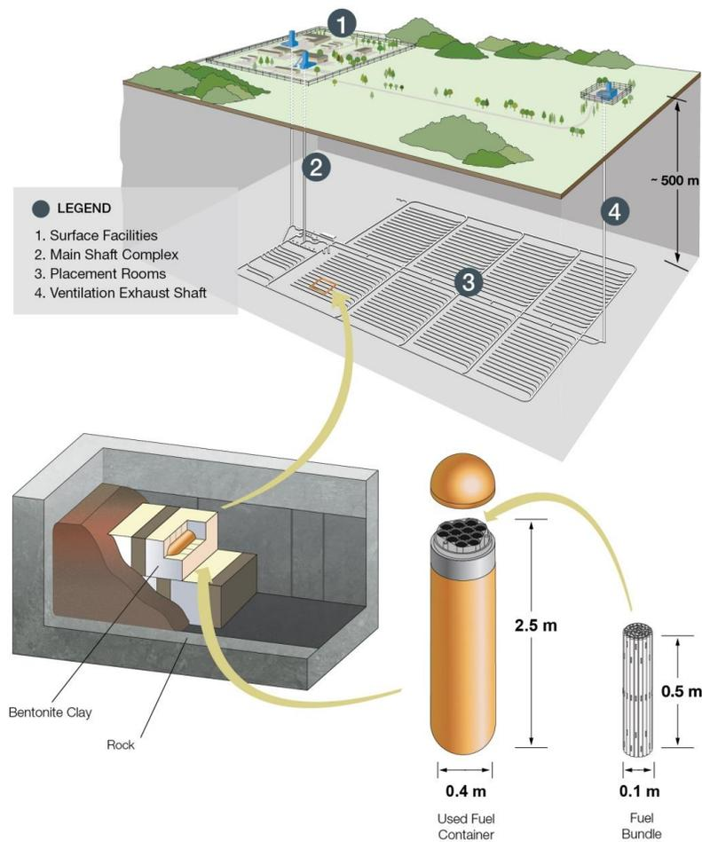
**Figure 1-1: Illustration of a Deep Geological Repository Reference Design**
