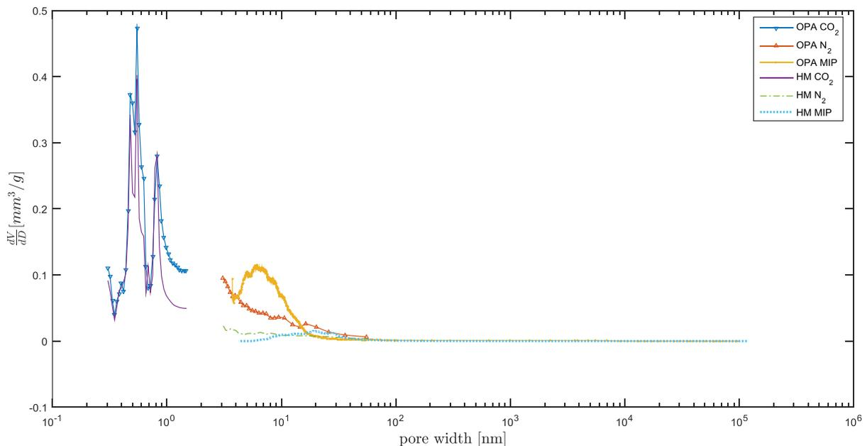
**Figure 4-5: Pore Size Distributions of Opalinus Clay and Helvetic Marl Measured by CO<sub>2</sub>- and N<sub>2</sub>-adsorption and MIP**
