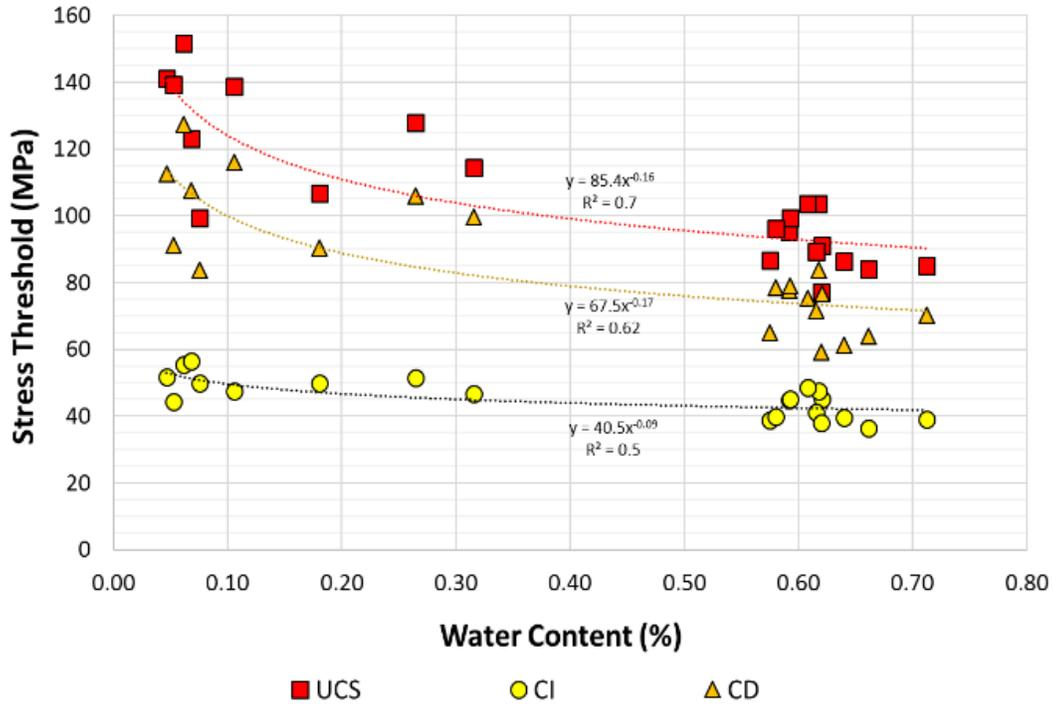
**Figure 4-18: Comparison of CI, CD, and UCS Stress Thresholds with Respect to Specimen Water Content**
