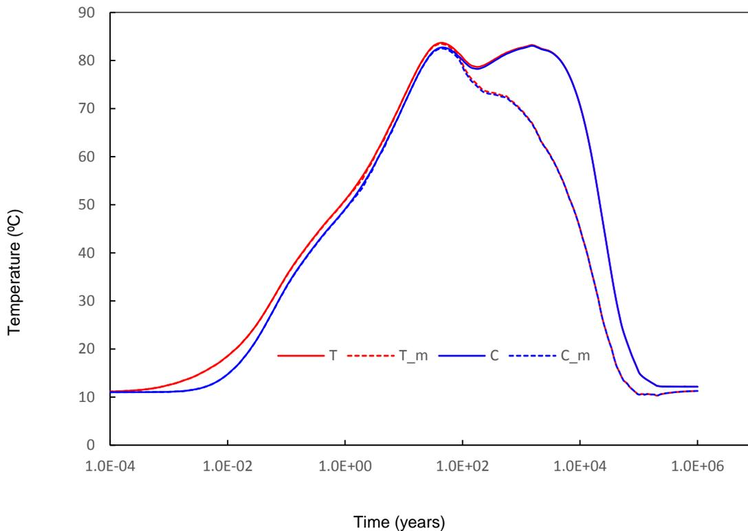
**Figure 5-6: Comparison of the Temperature as a Function of Time at Point T (container surface) and Point C (centre of tunnel) between Near-Field Modelling Results and Modified Results**
