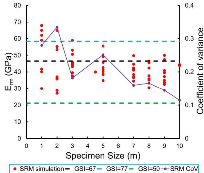
**Figure 4-12: Elastic Modulus Obtained from SRM Simulations and Empirical Hoek-Diederichs Equation (Hoek and Diederichs 2006) for Different Specimen Sizes (Farahmand 2017)**
