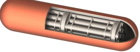
Figure 4-3: Copper Coated Used Fuel Container
