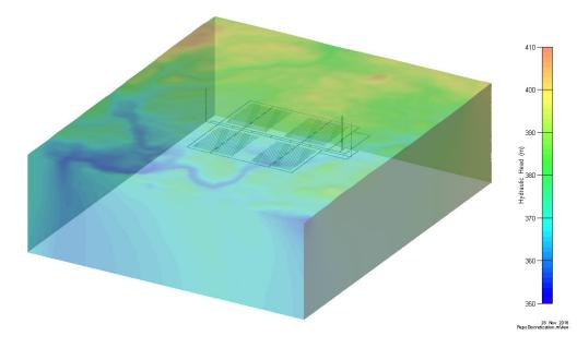
Figure 7-30: Full Repository-Scale Model: Base Case Head Boundaries
