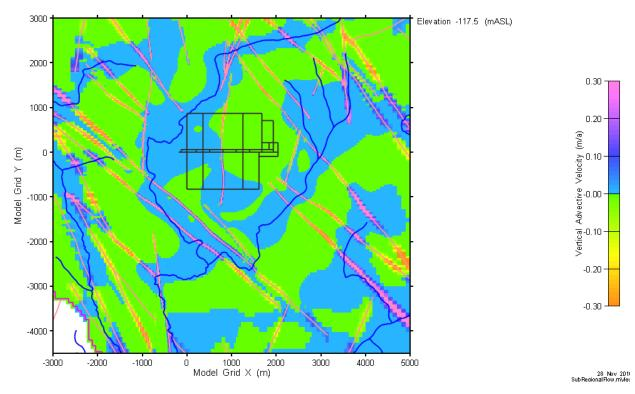
Figure 7-39: Subregional-Scale Model: Base Case (No Well) - Vertical Advective Velocity at Repository Elevation
