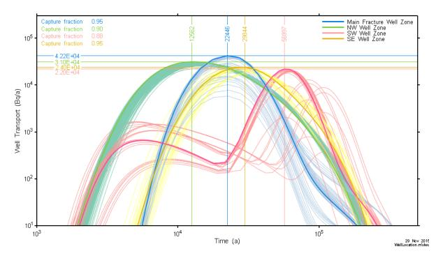
Figure 7-72: Rooms-Only Repository-Scale Model: Well / Source Transport Simulations
