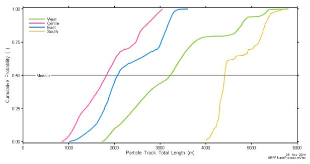
Figure 7-47: Subregional-Scale Model: Base Case (No Well) - Pathway Travel Length Cumulative Distribution Function
