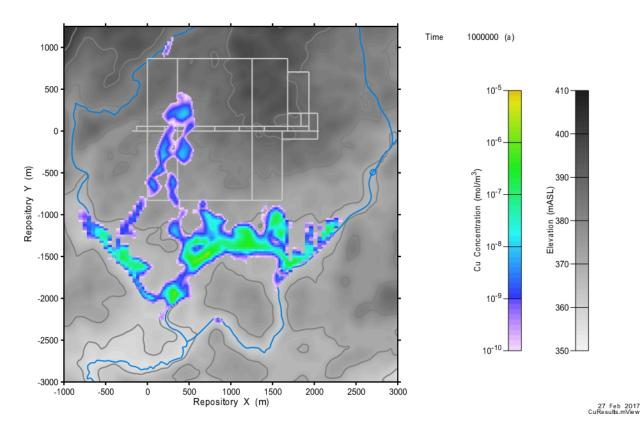
Figure 7-201: Rooms-Only Repository-Scale Model: Copper Concentration across the Repository Site (with well)
