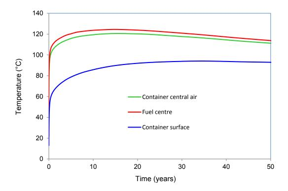
Figure 5-9: Temperature inside Container after Placement in Crystalline Rock [Guo 2015]
