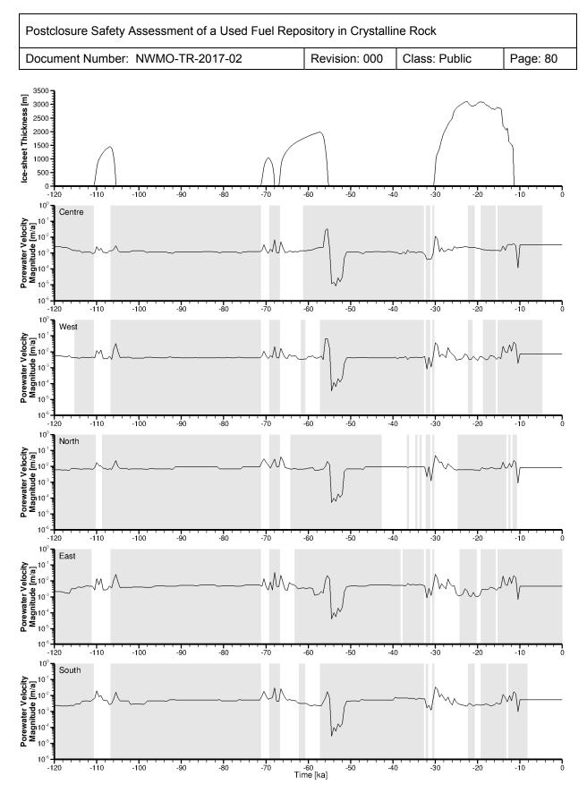
Figure 2-39: Velocity Magnitude versus Time for nn2008 Paleoclimate Boundary Conditions and a Loading Efficiency of 1 (fr-base-paleo-le1)
