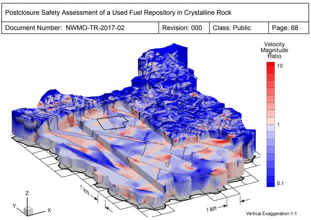
Figure 2-23: Ratio of Velocity Magnitudes for a Recharge Surface Boundary Condition Relative to the Reference Case
