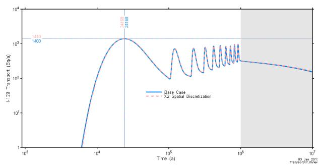
Figure 7-111: Rooms-Only Repository-Scale Model: Spatial Convergence Sensitivity – I-129 Transport to the Well
