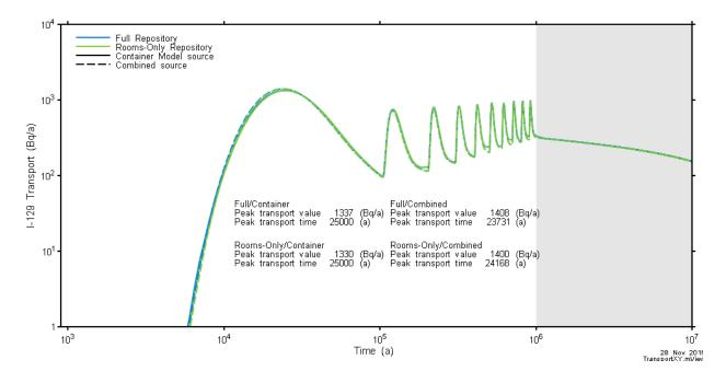
Figure 7-64: Repository-Scale Models: Comparison of Full Model and Rooms-Only Model for the Container Source Term and the Combined Source Term for I-129 Transport to the Main Well
