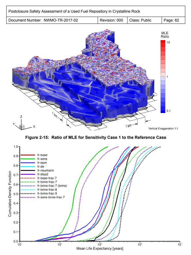
Figure 2-16: Cumulative Density Function of Mean Life Expectancy within Repository Outline at Repository Depth for Temperate Sensitivity Cases
