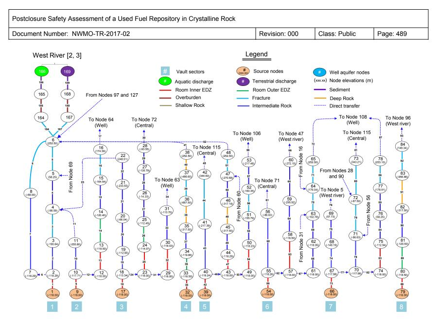
Figure 7-145: System Model, Full Geosphere Submodel: Transport Network Connectivity – Part I
