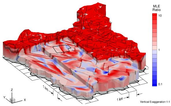
Figure 2-24: Ratio of MLE for a Recharge Surface Boundary Condition Relative to the Reference Case
