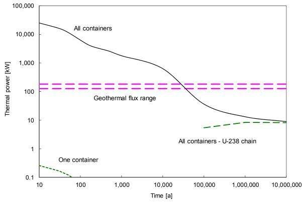
Notes: The power is similar to the natural geothermal flow (Perry et al. 2010) through the repository area after about 30,000 years. After about 1 million years, the residual power is due to radioactive decay of the decay products of uranium.
