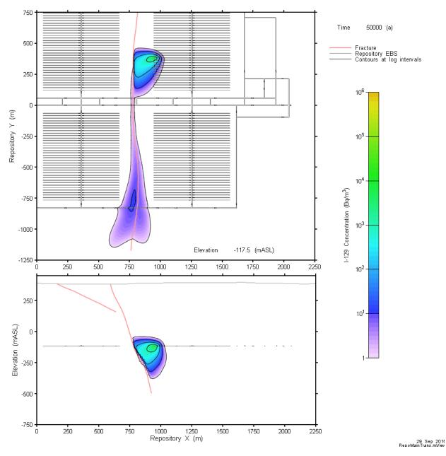
Figure 7-79: Full Repository-Scale Model: Base Case I-129 Concentration at 50 k Years
