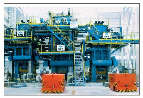
Figure 4-12: Example of a Closed-Die Forging Press (Uniaxial Compaction)
