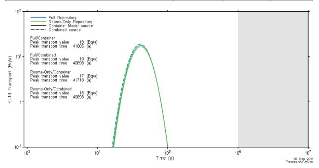
Figure 7-65: Repository Model – Comparison of Model (Full and Rooms-Only) and Source Term (Container model or Combined) C-14 Transport to Main Well
