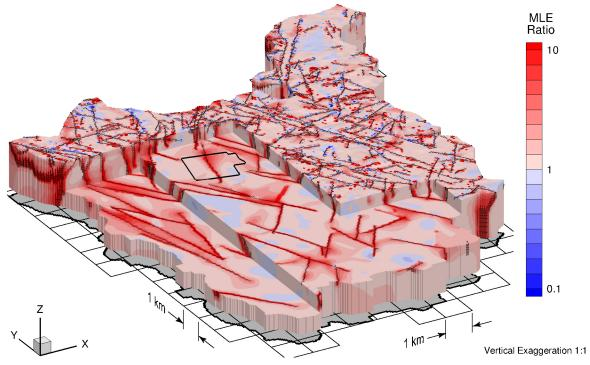
Figure 2-26: MLE Ratio of Uniform Fracture Zone Hydraulic Conductivity of 10<sup>-7</sup> m/s Relative to Reference Case Simulation
