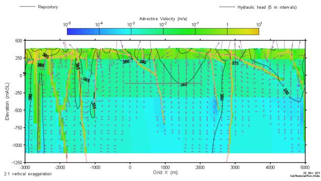
Figure 7-41: Subregional-Scale Model: Base Case (No Well) - Advective Velocity and Hydraulic Head on a Vertical Slice through the Grid Origin
