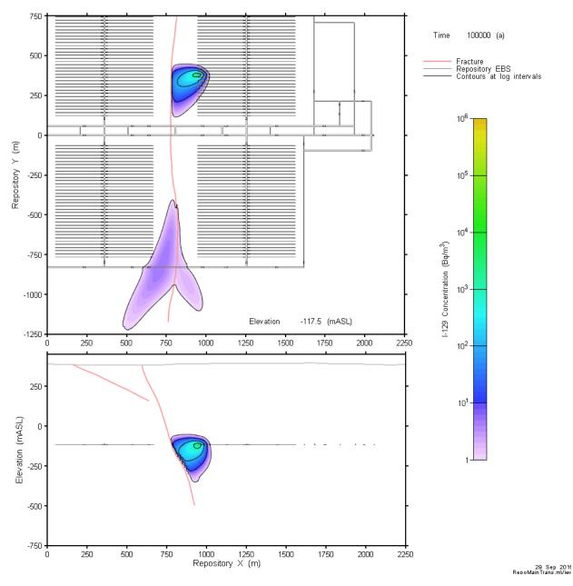
Figure 7-80: Full Repository-Scale Model: Base Case I-129 Concentration at 100 k Years
