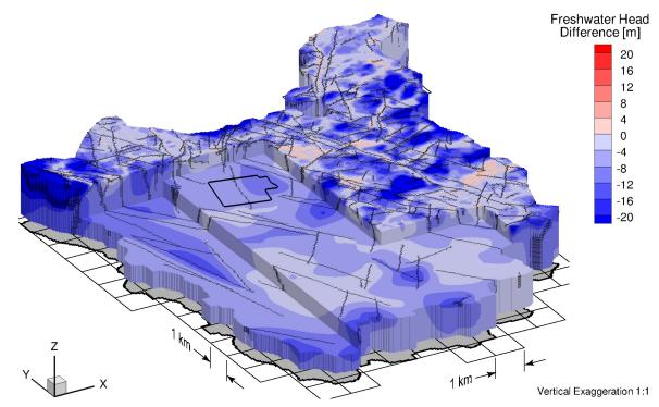
Figure 2-22: Difference in Freshwater Heads for a Recharge Surface Boundary Condition Relative to the Reference Case
