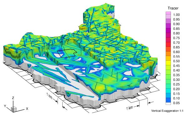
Figure 2-35: Tracer Migration at 120,000 Years for nn2008 Paleoclimate Boundary Conditions Loading Efficiency of 1 and a 0% of Ice-Sheet Thickness Equivalent Freshwater Head for the Surface Hydraulic Boundary Condition (fr-base-paleo-0-le1)
