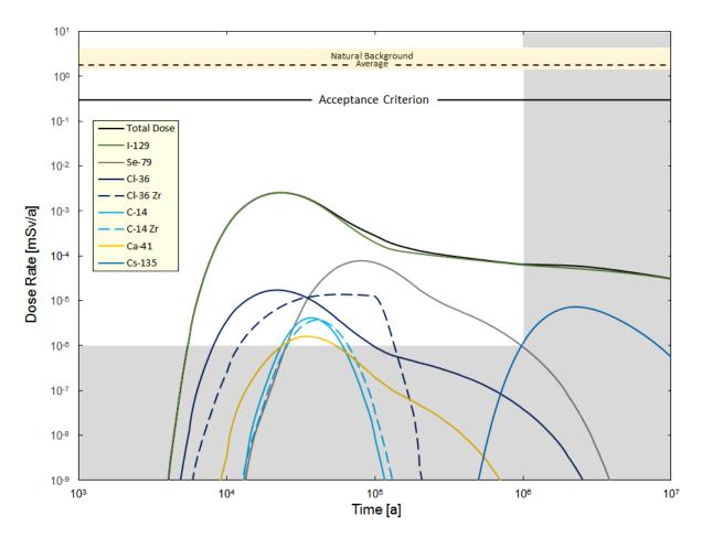
Figure 7-159: System Model: Sensitivity to All 10 Containers Fail at 1000 years
