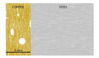
Figure 5-14: Hypothetical Defects in the Copper Coating
