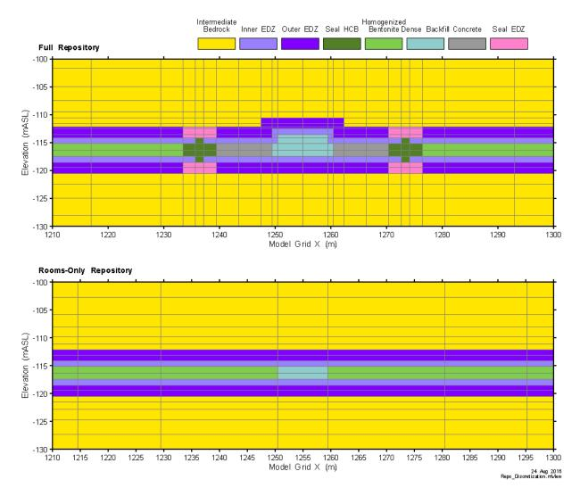
Figure 7-24: Repository-Scale Models: Detailed Vertical Discretization
