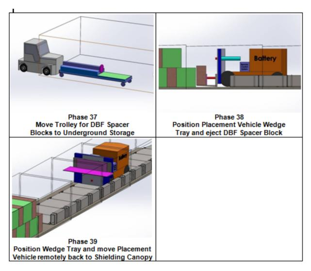
Figure 4-22: Container/Buffer Box Placement (concluded)
