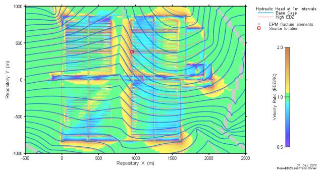
Figure 7-97: Full Repository-Scale Model: EDZ Hydraulic Conductivity Sensitivity - Plan View Velocity Ratio and Hydraulic Head Contours
