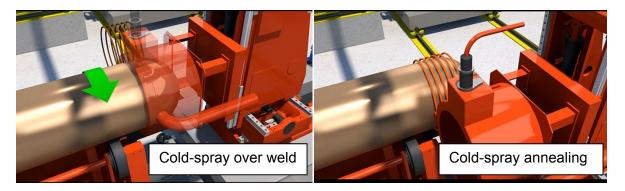
Figure 4-11: Copper Cold Spray and Copper Annealing Worktable
