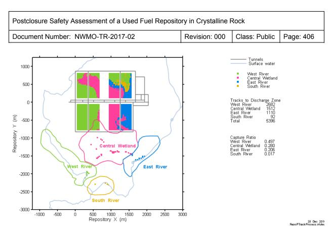
Figure 7-54: Rooms-Only Repository-Scale Model: Base Case No-Well Transport Pathway Discharge Zones
