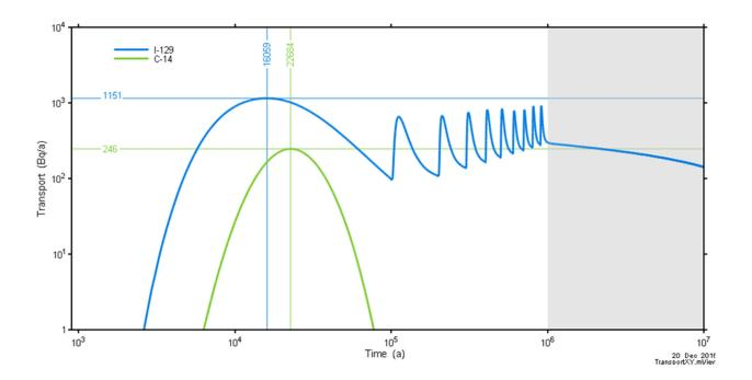
Figure 7-75: Rooms-Only Repository-Scale Model: I-129 and C-14 Well Transport for the NW Zone
