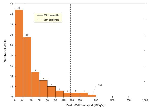
Figure 7-68: Rooms-Only Repository-Scale Model: Histogram of Peak Well Transport for All Tested Well Locations for the Tracer Source Term
