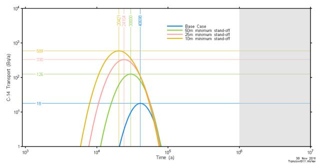
Figure 7-102: Rooms-Only Repository-Scale Model: Fracture Location Sensitivity – C-14 Transport
