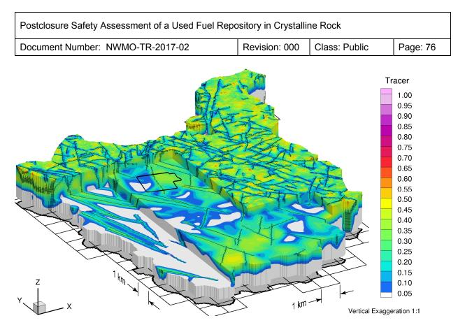
Figure 2-34: Tracer Migration at 120,000 Years for nn2008 Paleoclimate Boundary Conditions and a Loading Efficiency of 0 (fr-base-paleo-le0)
