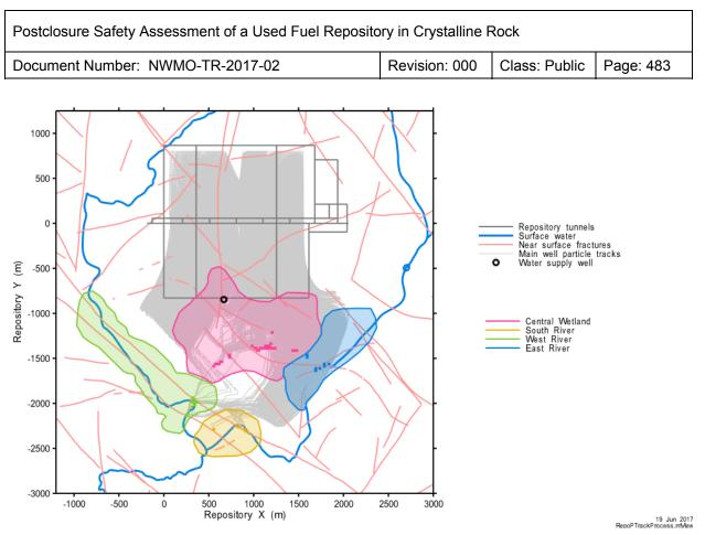
Figure 7-141: Repository-Scale Model: Surface Discharge Zones
