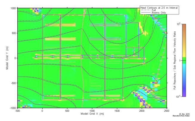
Figure 7-51: Repository Scale Models: Comparison of Hydraulic Heads and Advective Velocities at Repository Elevation
