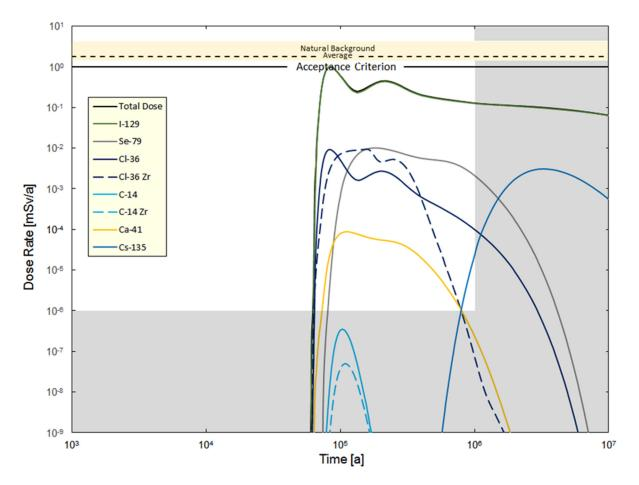
Figure 7-187: Full System Model: All Containers Fail at 60,000 Years: Contributing Radionuclides
