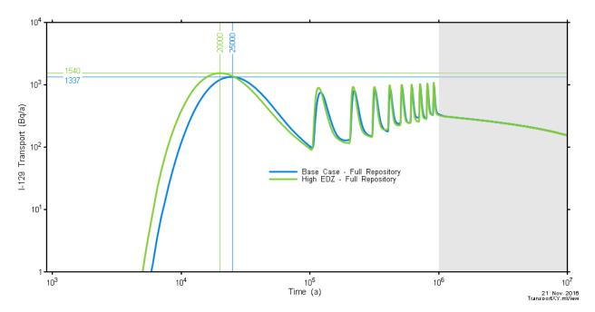
Figure 7-96: Repository-Scale Models: EDZ Hydraulic Conductivity Sensitivity - I-129 Transport to the Well
