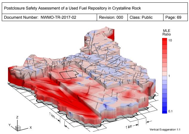
Figure 2-25: Ratio of MLE for a Density-Dependent Groundwater Flow Case to a Steady-State Case for Uniform Fracture Zone Hydraulic Conductivity of 10<sup>-7</sup> m/s
