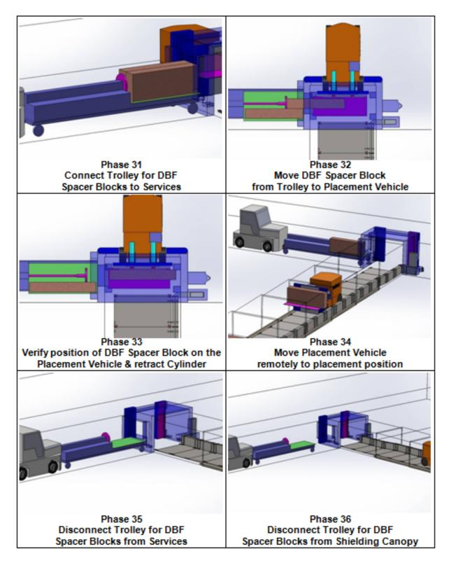
Figure 4-22: Container/Buffer Box Placement (continued)
