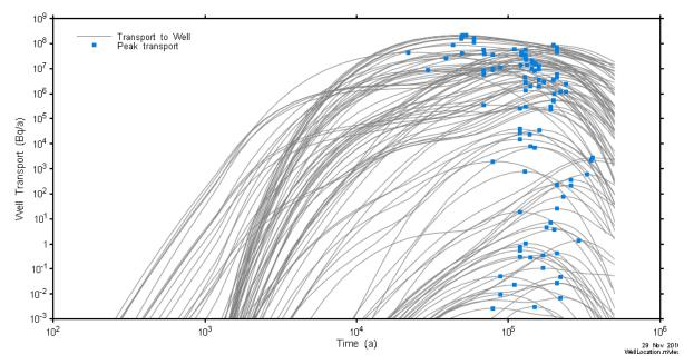
Figure 7-67: Rooms-Only Repository-Scale Model: Well Transport for All Tested Well Locations for the Tracer Source Term
