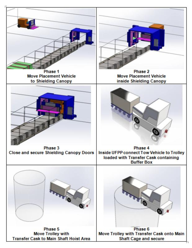
Figure 4-22: Container/Buffer Box Placement
