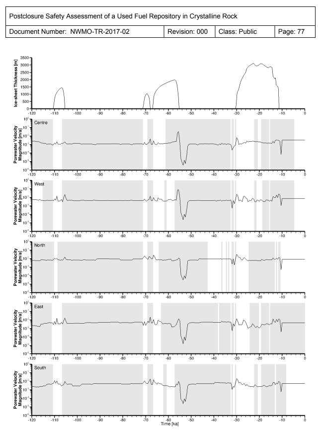
Figure 2-36: Velocity Magnitude versus Time for the nn2008 Reference Case Paleohydrogeological Scenario (fr-base-paleo)
