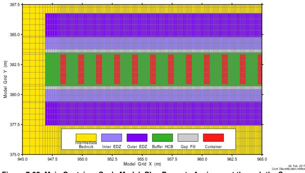
Figure 7-32: Main Container-Scale Model: Plan Property Assignment through the Source Placement Room
