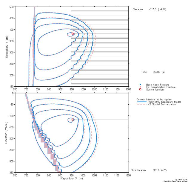
Figure 7-109: Rooms-Only Repository-Scale Model: Spatial Convergence Sensitivity – I-129 Transport
