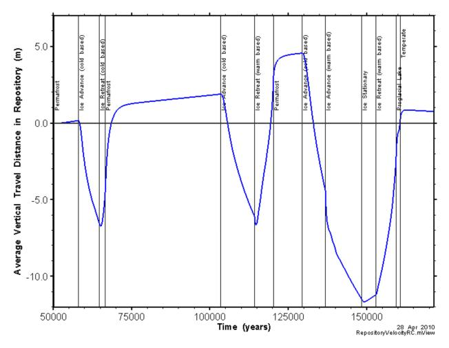
Figure 7-169: Cumulative Average Vertical Advective Flow Distance
