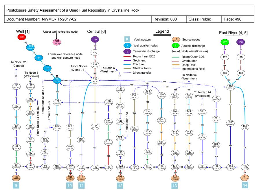
Figure 7-146: System Model, Full Geosphere Submodel: Transport Network Connectivity – Part II
