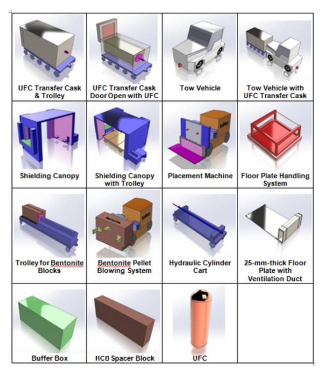
Figure 4-20: Legend for Container Placement Equipment
