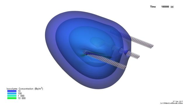
Figure 7-133: Main Container-Scale Model: Three-Dimensional Visualization of Cs-135 Concentration at 100 ka
