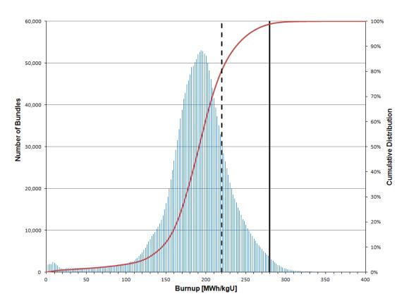
Note: The vertical dashed and solid black lines correspond to burnup values of 220 MWh/kgU and 280 MWh/kgU, while the red line represents the cumulative distribution. The figure is based on data in Wilk (2013).
