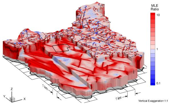
Figure 2-28: MLE Ratio of Uniform Fracture Zone Hydraulic Conductivity of 10<sup>-9</sup> m/s Relative to Reference Case Simulation
