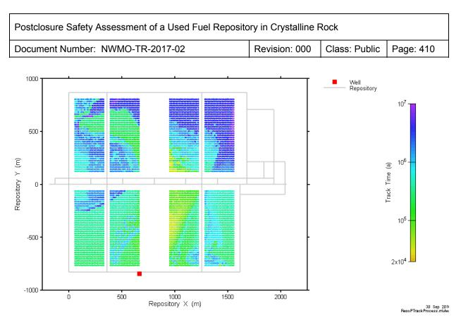
Figure 7-61: Rooms-Only Repository-Scale Model: Main Well Transport Pathway Travel Time to Discharge
