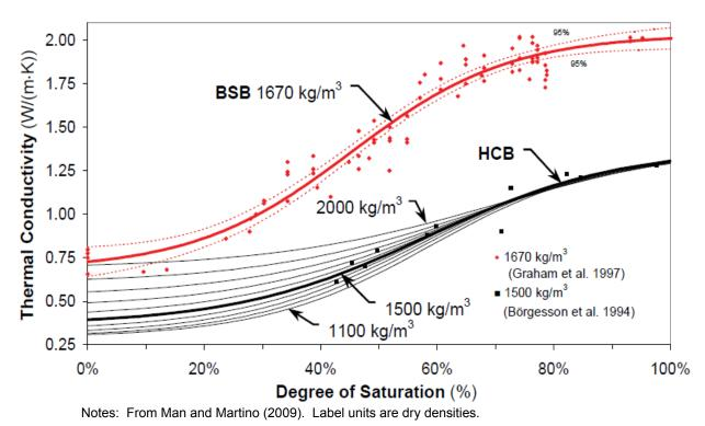
Figure 5-23: Thermal Conductivity of 50:50 wt% Bentonite-Sand Buffer (BSB) and of 100 wt% MX-80 Bentonite
