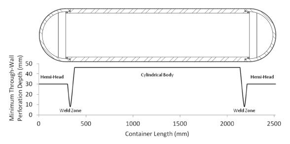
Figure 5-16: Minimum Corrosion Depth for Through-Wall Perforation of Steel Container
