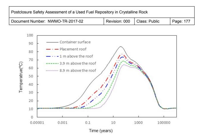
Figure 5-3: Illustrative Example of the Range of Temperature Variation over Time in a Placement Room
