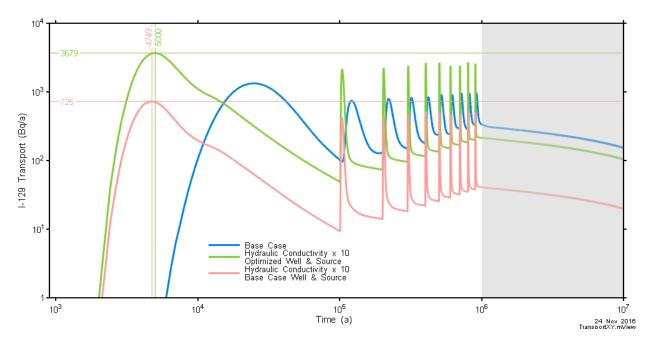
Figure 7-94: Rooms-Only Repository-Scale Model: Base Case Geosphere Hydraulic Conductivity x 10 with Repositioned Well – I-129 Transport to the Well
