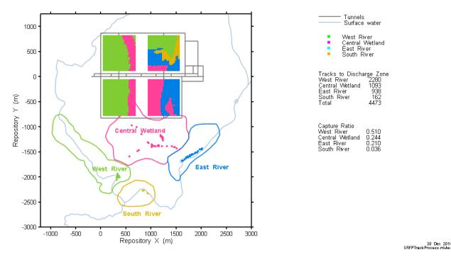
Figure 7-44: Subregional-Scale Model: Base Case (No Well) - Discharge Zones
