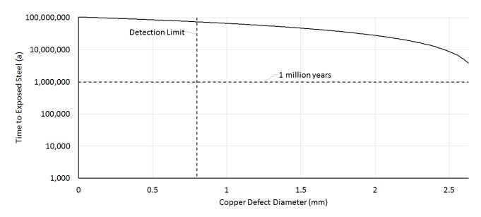
Figure 5-15: Time to Exposed Steel beneath Defects in a Nominal 3 mm Copper Coating
