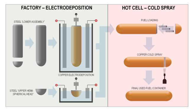
Note: This figure shows the two processes used for copper-coating the container: 1) the lower assembly and the upper hemispherical head are electroplated in a factory environment; and 2) the final steel zone is welded after the used fuel is loaded in the hot cell and then cold-sprayed with copper.
