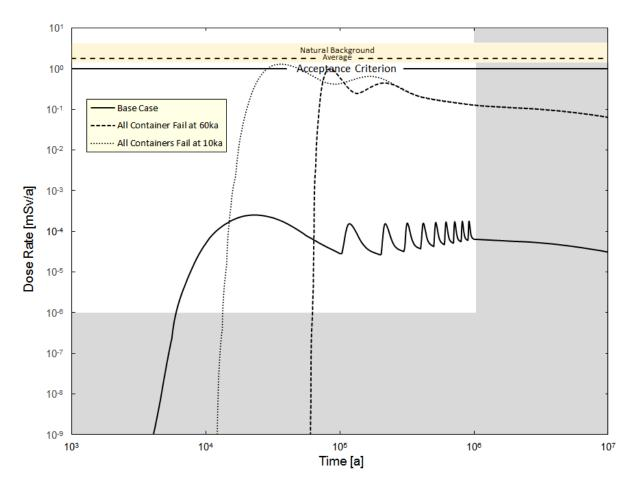
Figure 7-188: All Containers Fail at 10,000 Years: Sensitivity Case Dose Rate
