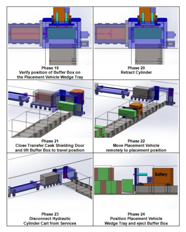
Figure 4-22: Container/Buffer Box Placement (continued)
