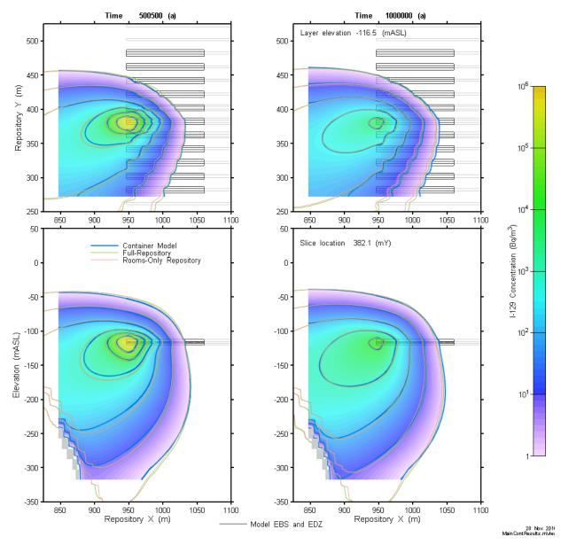
Figure 7-123: Main Container-Scale Model: I-129 Concentration at 500.5 ka and 1 Ma
