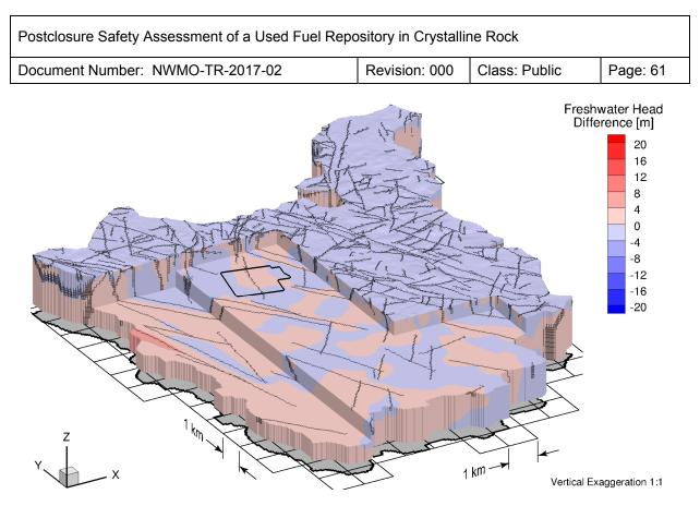
Figure 2-13: Difference in Freshwater Heads between Sensitivity Case 1 and the Reference Case
