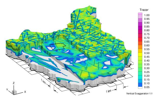
Figure 2-29: Tracer Migration after 120,000 Years for nn2008 Reference Case Paleohydrogeologic Scenario (fr-base-paleo)
