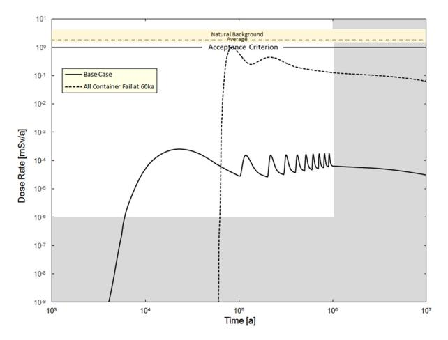
Figure 7-186: Full System Model: All Containers Fail at 60,000 Years: Dose Rate
