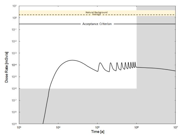
Figure 7-152: System Model: Base Case Total Dose Rate
