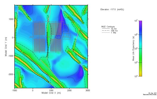
Figure 7-52: Full Repository-Scale Model: Mean Life Expectancy at Repository Elevation
