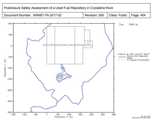
Figure 7-110: Rooms-Only Repository-Scale Model: Spatial Convergence Sensitivity – Peak I-129 Transport at Surface
