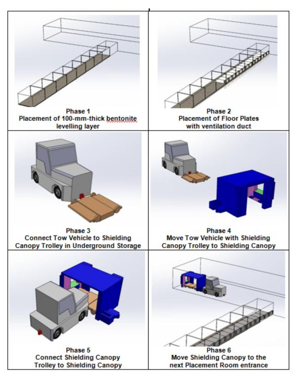
Figure 4-21: Preparation of Placement Room & Shielding Canopy
