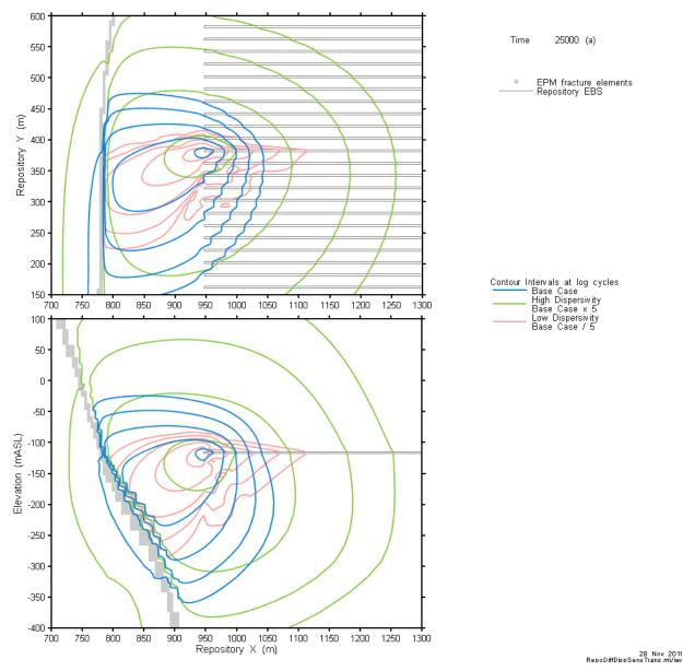
Figure 7-106: Rooms-Only Repository-Scale Model: Dispersivity Sensitivity – Contours of I-129 Concentration in the Geosphere
