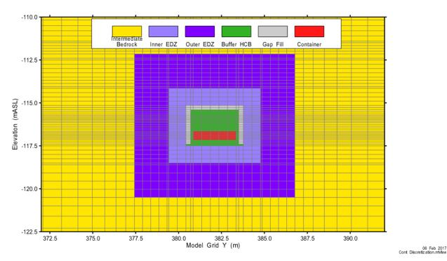
Figure 7-34: Main Container-Scale Model: Vertical Property Assignment Perpendicular to the Source Placement Room
