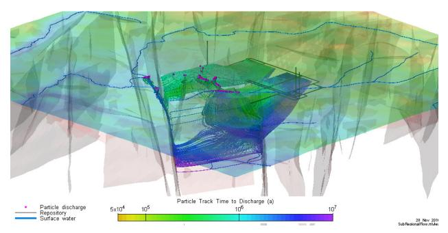
Figure 7-43: Subregional-Scale Model: Base Case (No Well) – Three Dimensional Transport Pathways from Repository to Discharge
