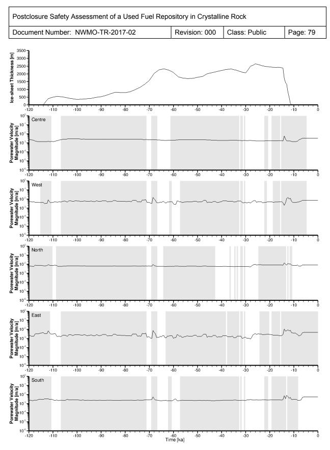
Figure 2-38: Velocity Magnitude versus Time for the "Peltier 2015" Paleoclimate Boundary Conditions (fr-base-paleo-peltier)
