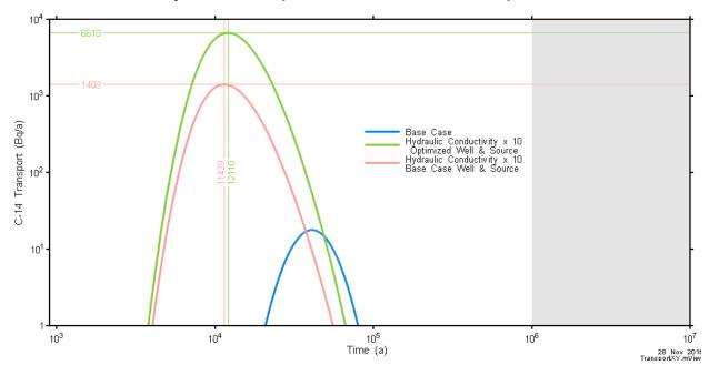
Figure 7-95: Rooms-Only Repository-Scale Model: Base Case Geosphere Hydraulic Conductivity x 10 with Repositioned Well – C-14 Transport to the Well
