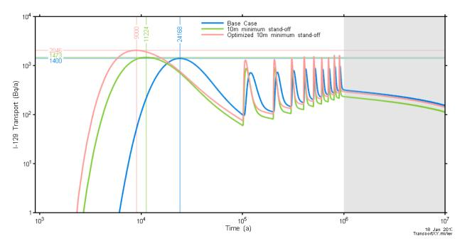
Figure 7-104: Rooms-Only Repository Scale Model: Fracture Location Sensitivity – I-129 Transport to the Well for Alternate Well Location
