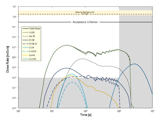
Figure 7-155: System Model: Sensitivity to a Factor of 10 Increase in Fuel Dissolution Rate
