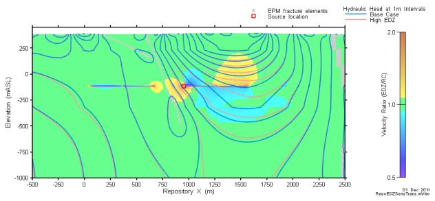
Figure 7-98: Full Repository-Scale Model: EDZ Hydraulic Conductivity Sensitivity Case – Vertical Section View Velocity Ratio and Hydraulic Head Contours
