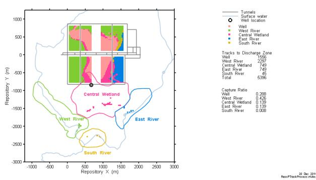
Figure 7-60: Rooms-Only Repository-Scale Model: Main Well Transport Pathway Discharge Zones
