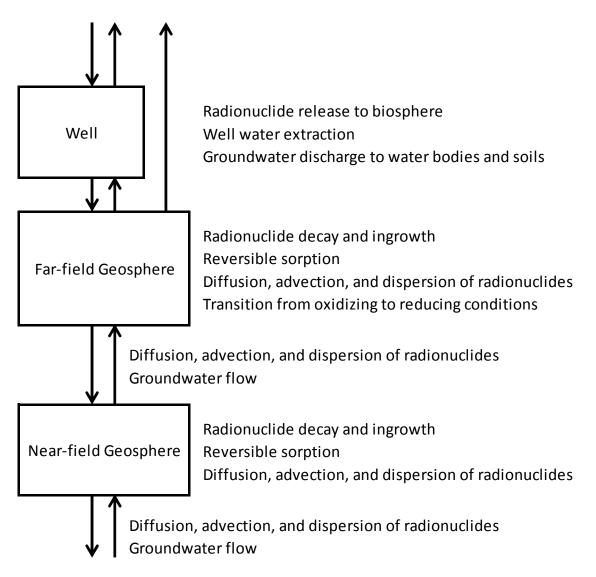
Figure 7-5: Conceptual Model for the Geosphere
