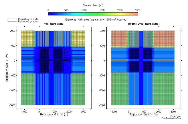
Figure 7-22: Repository-Scale Models: Plan Discretization
