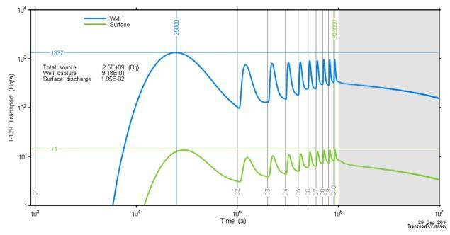
Figure 7-76: Full Repository-Scale Model: I-129 Transport for the Main Fracture Zone
