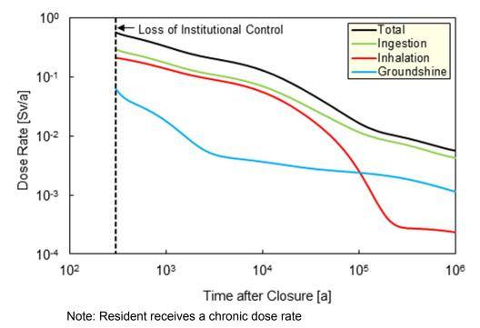
Figure 7-183: Inadvertent Human Intrusion: Exposure Pathways for the Resident – Hazard Not Identified and Site Vacated after 14 Days
