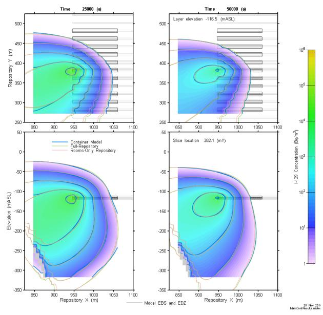
Figure 7-121: Main Container-Scale Model: I-129 Concentration at 25 ka and 50 ka
