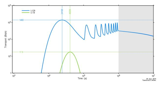
Figure 7-74: Rooms-Only Repository-Scale Model: I-129 and C-14 Well Transport for the Main Fracture Zone
