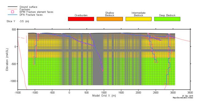
Figure 7-23: Full Repository-Scale Model: Vertical Discretization
