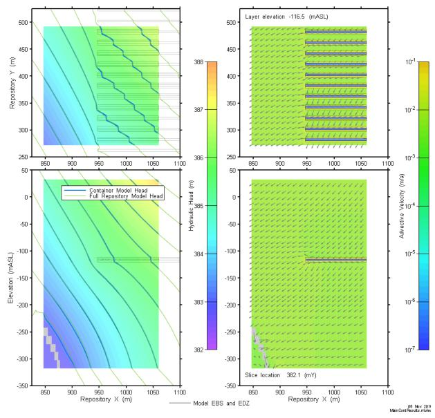
Figure 7-115: Main Container-Scale Model: Hydraulic Head and Advective Velocity on Horizontal Plane through Repository (top) and Vertical Plane through Source Room (bottom)
