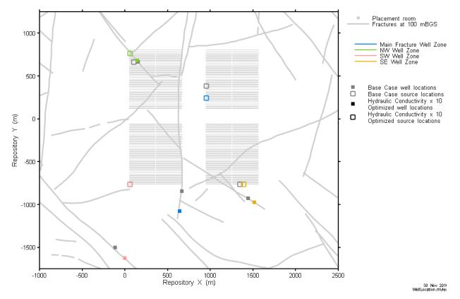
Figure 7-93: Rooms-Only Repository-Scale Model: Base Case Geosphere Hydraulic Conductivity x 10 – Updated Well and Defective Container Locations
