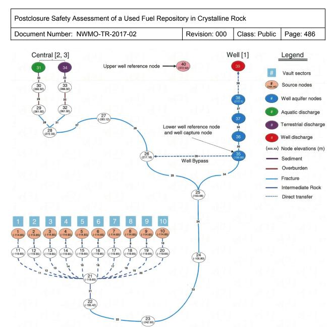
Notes: Only nodes (ellipses) with a particular function are colour coded. The line segments, representing the 1D transport pathways, are colour coded (see legend) to indicate the geosphere zone through which they pass.
