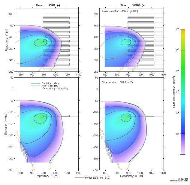
Figure 7-122: Main Container-Scale Model: I-129 Concentration at 75 ka and 100 ka
