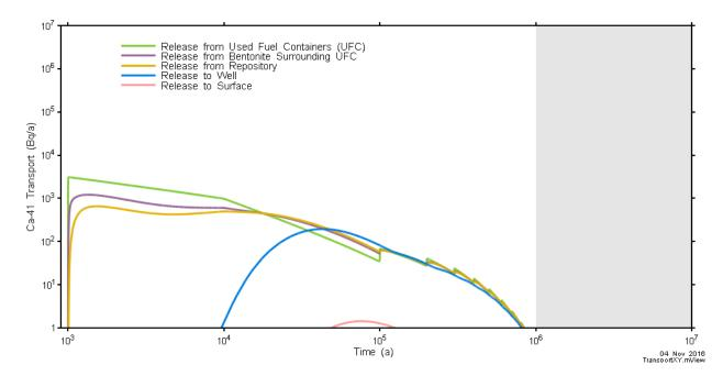
Figure 7-137: Full Repository and Main Container-Scale Models: Ca-41 Transport through Barriers
