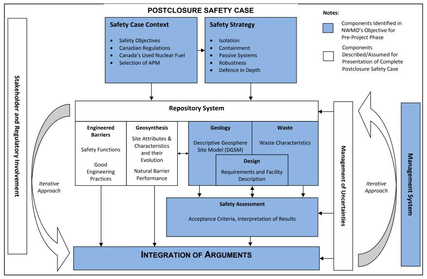
Figure 1-4: Components of the Safety Case
