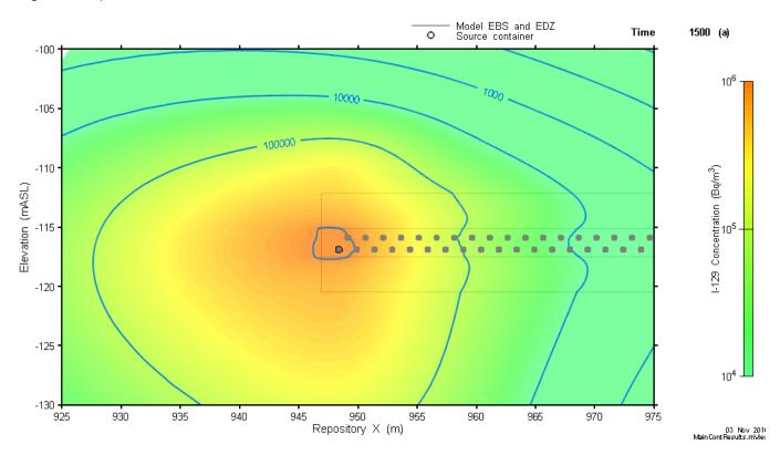
Figure 7-117: Main Container-Scale Model: Detail of I-129 Concentration 500 Years after Failure of the First Container (at 1500 a)
