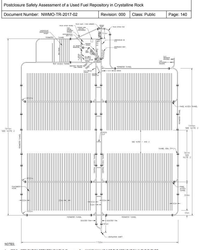
1. 252.8m SEPARATION BETWEEN PANELS IS BASED ON A HYPOTHETICAL FRACTURE ZONE WITH 100m STANDOFF 2. NWMO MAY ADJUST THE SEPARATION IN THE FUTURE BASED ON SITE SPECIFIC SAFETY ANALYSES.
