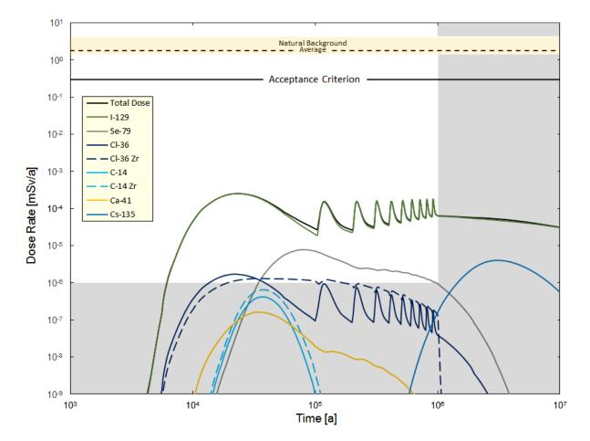
Figure 7-158: System Model: Sensitivity to Zircaloy Instant Release Fractions Set to 10%
