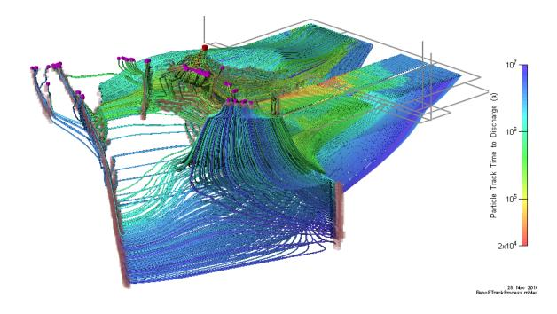
Figure 7-59: Rooms-Only Repository-Scale Model: Main Well Advective Transport Pathways
