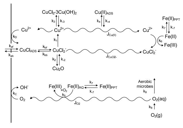
Notes: From King and Kolář (2000) and King et al. (2008, 2010, 2011a). The k's denote rate constants for the various interfacial electrochemical and homogeneous reactions and the J's denote diffusive fluxes.
