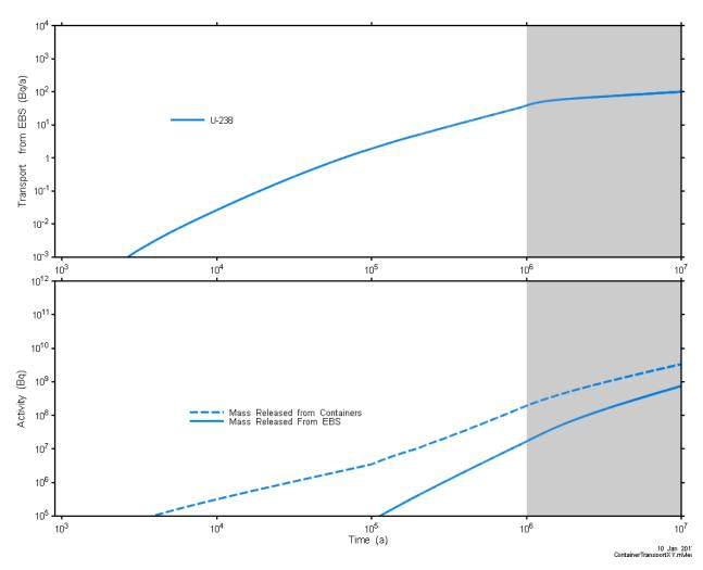
Figure 7-135: Main Container-Scale Model: Transport Rates and Cumulative Release for U-238
