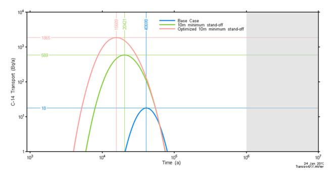
Figure 7-105: Rooms-Only Repository-Scale Model: Fracture Location Sensitivity – C-14 Transport to the Well for Alternate Well Location
