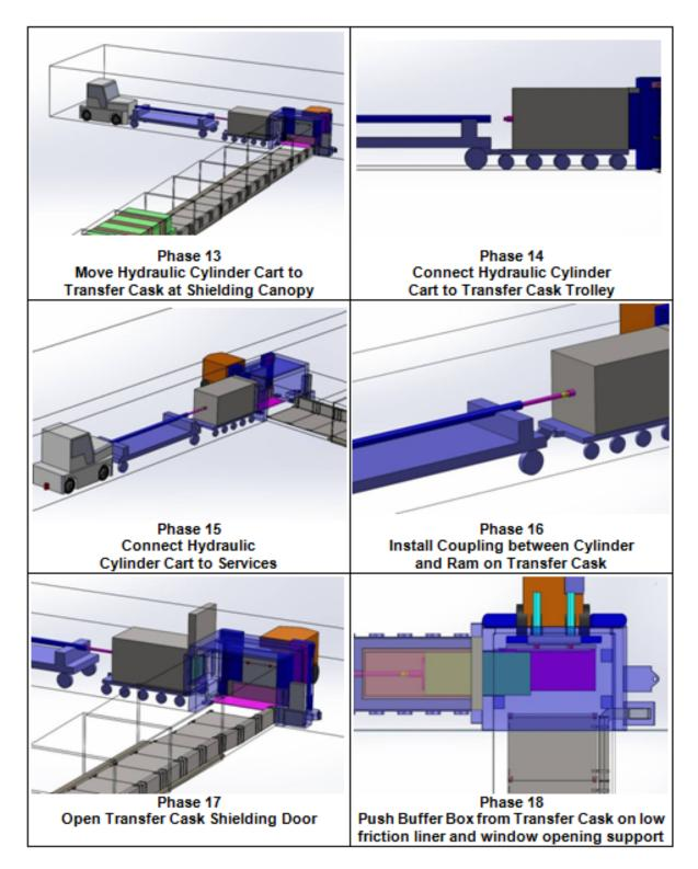
Figure 4-22: Container/Buffer Box Placement (continued)
