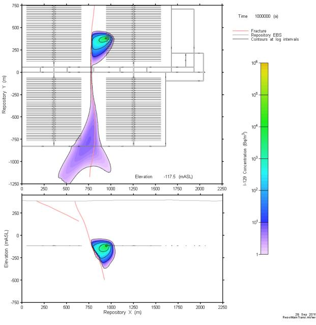
Figure 7-82: Full Repository-Scale Model: Base Case I-129 Concentration at One Million Years
