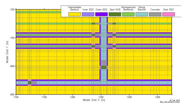
Figure 7-26: Full Repository-Scale Model: Detailed Plan Discretization Showing Seal Implementation
