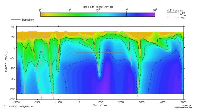
Figure 7-42: Subregional-Scale Model: Base Case (No Well) - Mean Life Expectancy on a Vertical Slice through the Grid Origin
