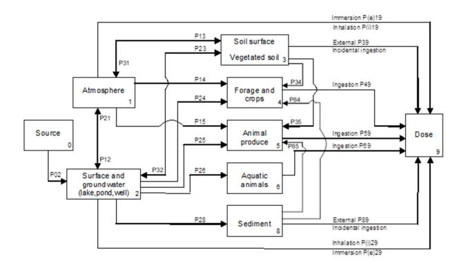
Notes: The nomenclature is from CSA (2014) and the Pij represent transfer parameters from compartment i to compartment j. The biosphere model includes all these environmental transfers and exposure pathways. The building material exposure pathway is not shown here since it is not included in the CSA (2014) dose model.
