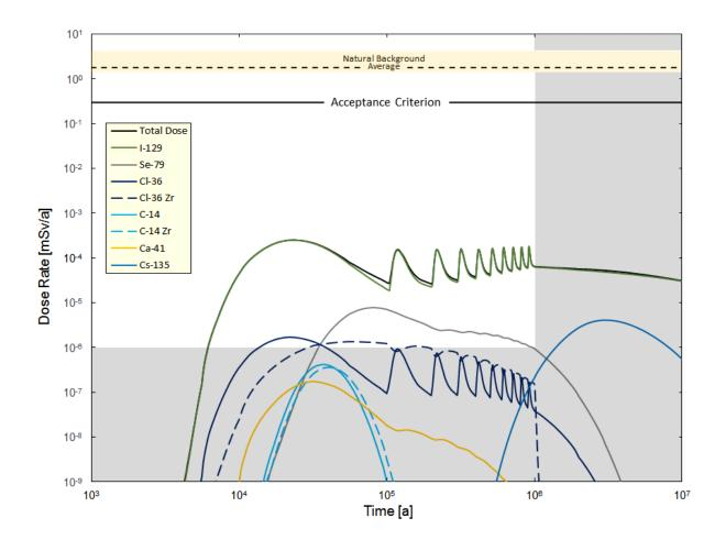
Figure 7-160: System Model: Sensitivity to Low Sorption in the EBS with Coincident High Solubility Limits in the Container
