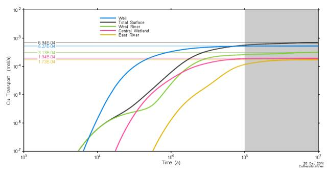
Figure 7-202 shows the transport of copper to the surface as a function of time.
