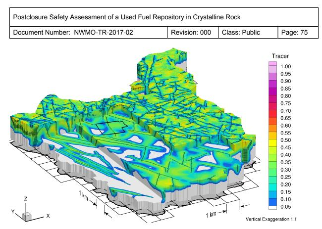
Figure 2-32: Tracer Migration at 120,000 Years for the "Peltier 2015" Paleoclimate Boundary Conditions (fr-base-paleo-peltier)
