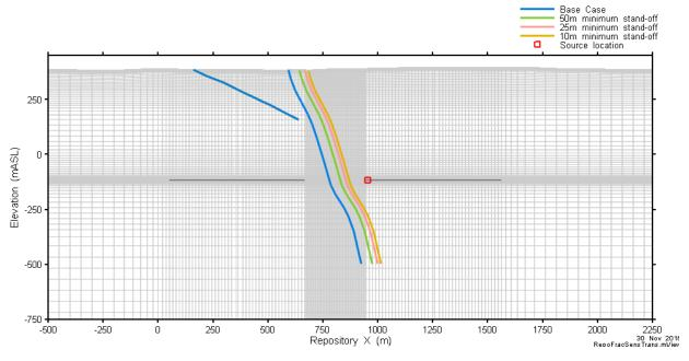
Figure 7-100: Rooms-Only Repository-Scale Model: Fracture Location Sensitivity -Vertical Cross-Section View
