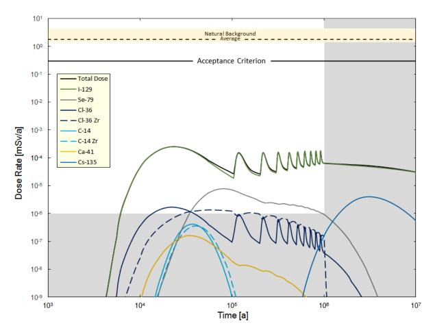
Figure 7-161: System Model: Sensitivity to No Solubility Limits
