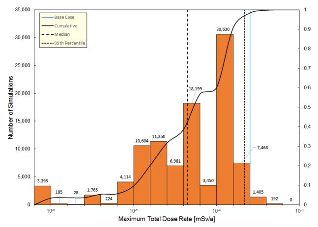
Note: The leftmost bin at 10<sup>-6</sup> mSv/a includes all simulations (3395) that resulted in a dose less than 10<sup>-6</sup> mSv/a
