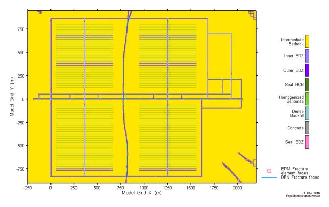
Figure 7-25: Full Repository-Scale Model: Plan View of Repository Property Assignment
