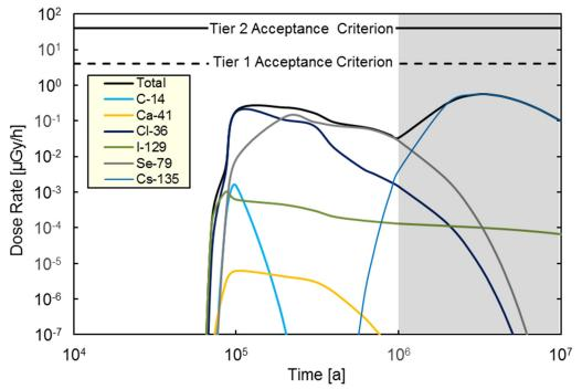
Note: C-14 and CI-36 dose rates result from the sum of releases originating from both the fuel and the fuel sheath.
