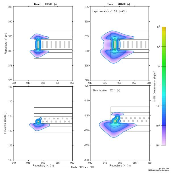
Figure 7-128: Main Container-Scale Model: U-238 Concentration at 100.5 and 200.5 ka
