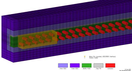
Figure 7-35: Main Container-Scale Model: 3D View of EBS and EDZ near Source Containers
