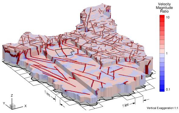
Figure 2-18: Ratio of Velocity Magnitudes for the EPM Case to the Reference Case
