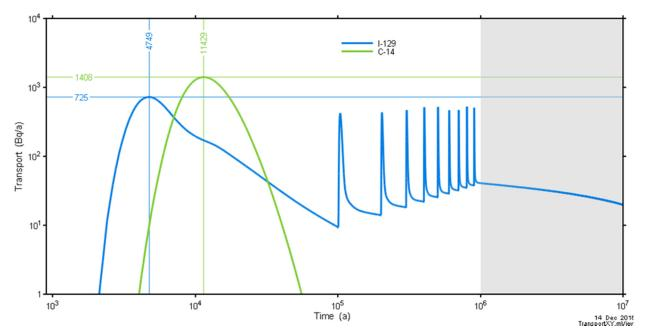
Figure 7-92: Rooms-Only Repository-Scale Model: Base Case Geosphere Hydraulic Conductivity x 10 - I-129 and C-14 Transport to the Well
