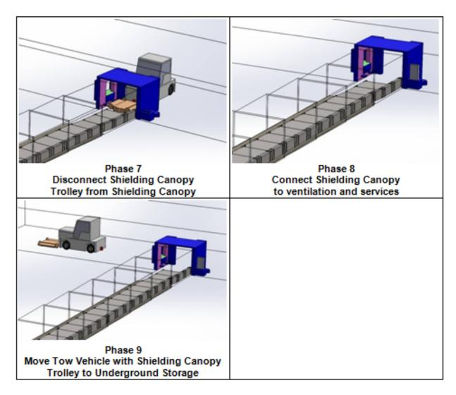
Figure 4-21: Preparation of Placement Room & Shielding Canopy (concluded)
