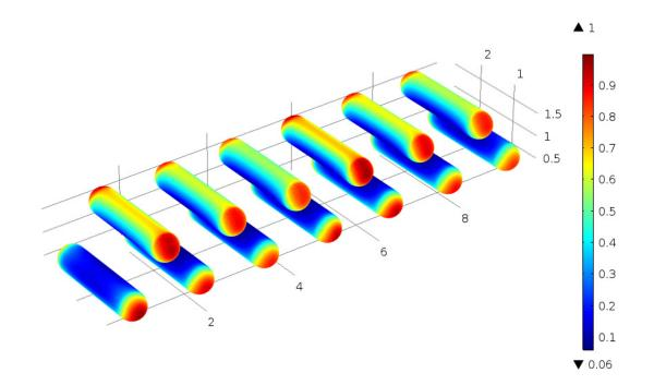
Figure 5-12: Normalized Diffusive Sulphide Flux Ratio for UFCs in Placement Room for a Uniform Background Concentration of Sulphide in the Host Rock
