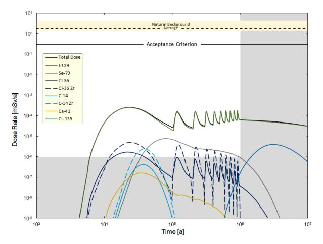
Figure 7-157: System Model: Sensitivity to a Factor of 10 Increase in Zircaloy Corrosion Rate
