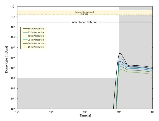
Figure 7-177: Probabilistic Assessment: Time Dependence of Percentile Values with Container Assumptions Varying
