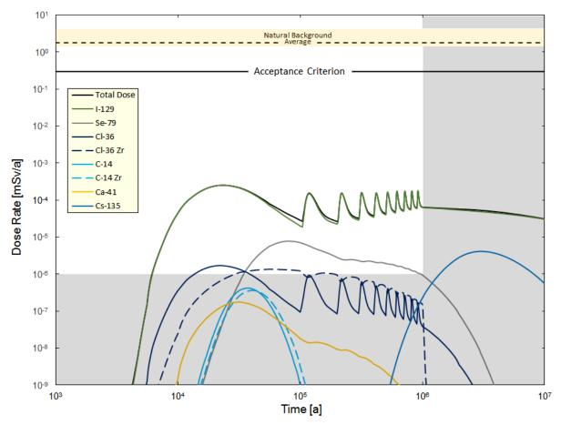
Figure 7-162: System Model: Sensitivity to No Sorption in the Near Field
