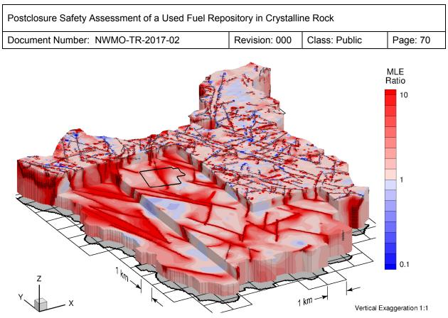
Figure 2-27: MLE Ratio of Uniform Fracture Zone Hydraulic Conductivity of 10<sup>-8</sup> m/s Relative to Reference Case Simulation
