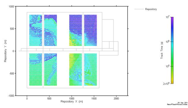
Figure 7-55: Rooms-Only Repository-Scale Model: Base Case No-Well Transport Pathway Travel Time to Discharge
