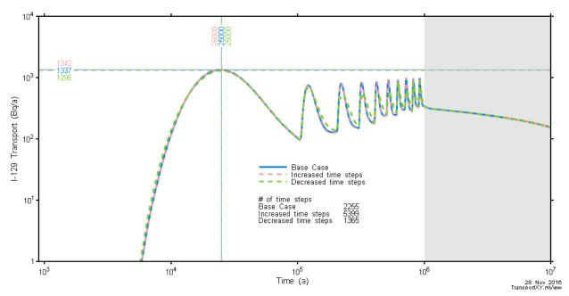
Figure 7-113: Full Repository Scale-Model: Time Step Convergence Sensitivity with Container Source Term – I-129 Transport to the Well
