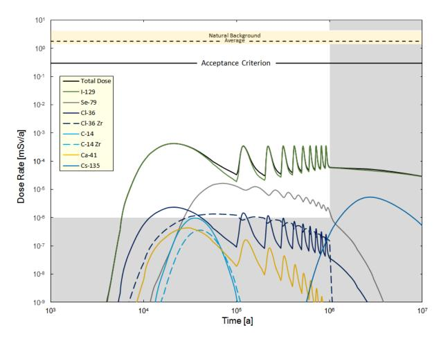
Figure 7-156: System Model: Sensitivity to Fuel Instant Release Fractions Set to 10%
