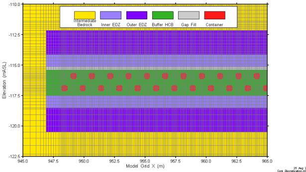
Figure 7-33: Main Container-Scale Model: Vertical Property Assignment Parallel to the Source Placement Room
