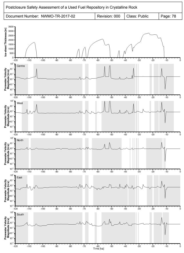
Figure 2-37: Velocity Magnitude versus Time for the nn2778 Paleoclimate Boundary Conditions (fr-base-paleo-nn2778)
