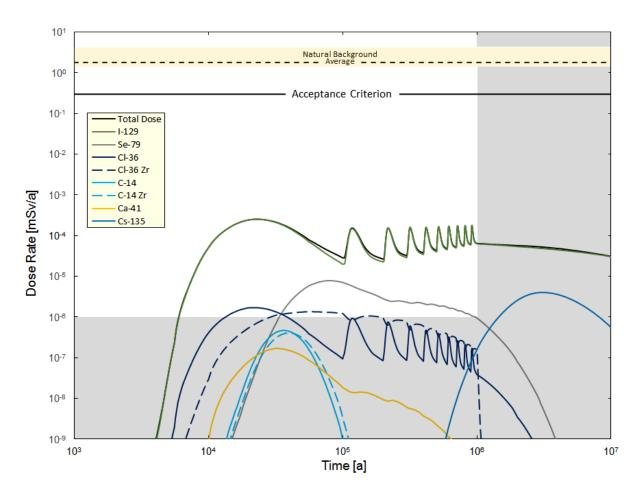
Figure 7-153: System Model: Base Case Individual Radionuclide Dose Rates
