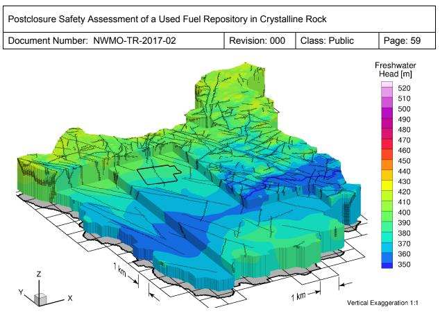
Note: Block-cuts occur at 500 mBGS and 1000 mBGS. The black outline in the centre of the figure delineates the repository location.
