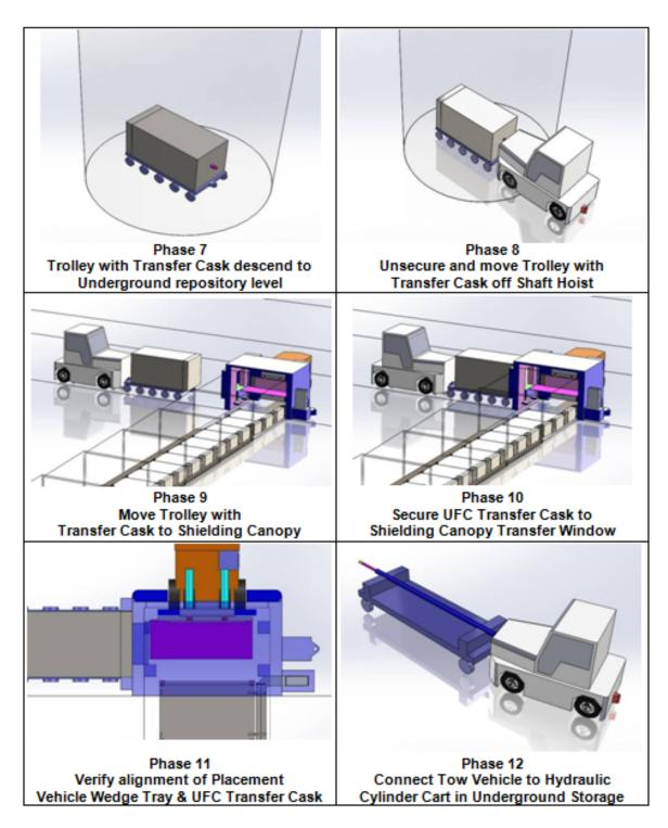
Figure 4-22: Container/Buffer Box Placement (continued)
