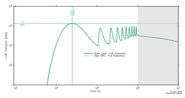
Figure 7-90: Full Repository-Scale Model: EBS Hydraulic Conductivity Sensitivity - I-129 Transport to the Well
