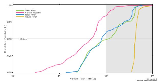
Figure 7-56: Rooms-Only Repository-Scale Model: Base Case No-Well Transport Pathway Travel Time Cumulative Distribution Function
