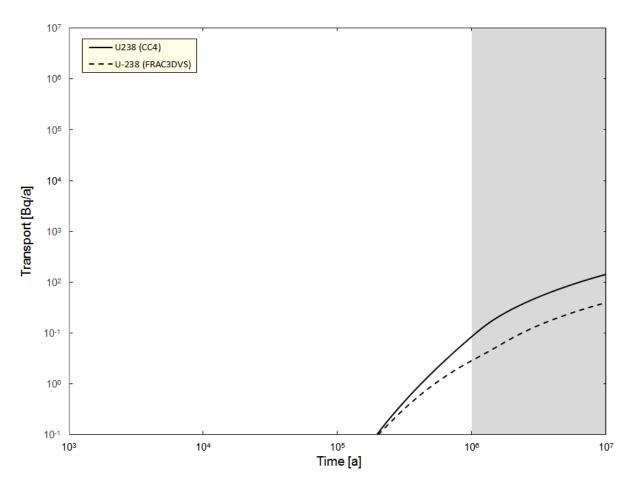
Figure 7-148: System Model, Simple Geosphere Submodel: Comparison U-238 Transport to the Geosphere
