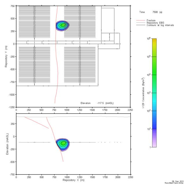
Figure 7-77: Full Repository-Scale Model: Base Case I-129 Concentration at 7,500 Years
