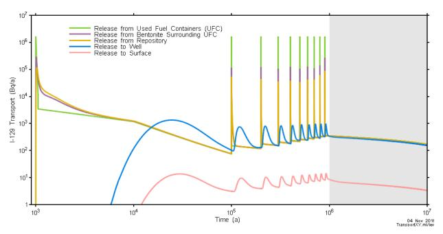
Figure 7-136: Full Repository and Main Container-Scale Models: I-129 Transport through Barriers
