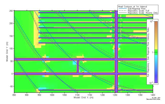
Figure 7-50: Repository-Scale Models: Comparison of Hydraulic Heads and Advective Velocities with Subregional-Scale Model at Repository Elevation
