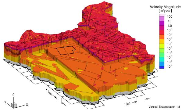
Figure 2-11: Reference Case Porewater Velocity Magnitudes
