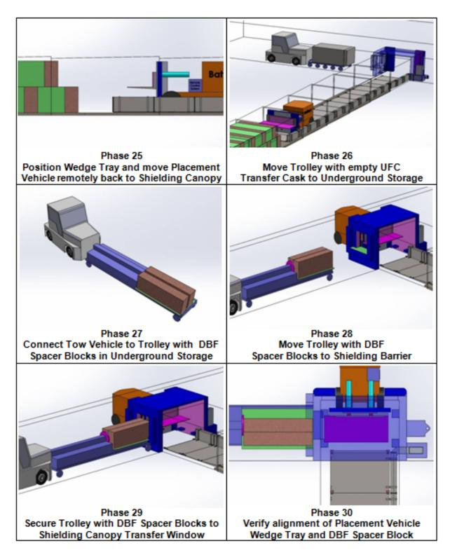
Figure 4-22: Container/Buffer Box Placement (continued)
