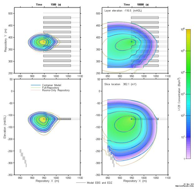
Figure 7-120: Main Container-Scale Model: I-129 Concentration at 1500 a and 10 ka
