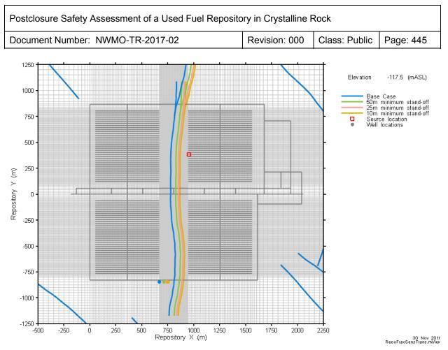
Figure 7-99: Rooms-Only Repository-Scale Model: Fracture Location Sensitivity - Plan View
