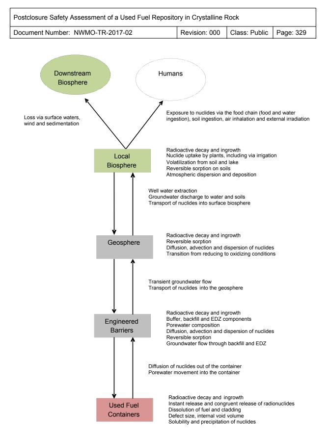
Figure 7-2: General Conceptual Model for Defective Containers
