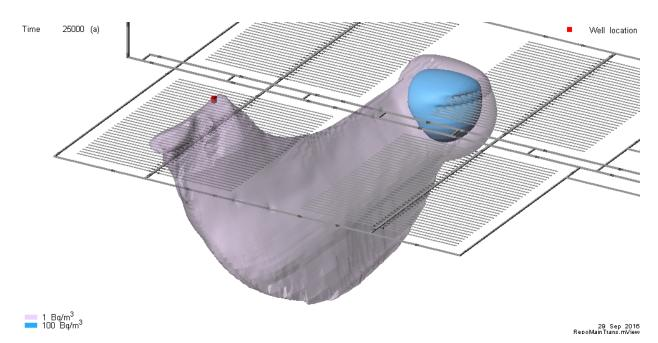
Figure 7-83: Full Repository-Scale Model: Base Case I-129 Concentration in 3D at Time of Peak Well Transport (25 ka)
