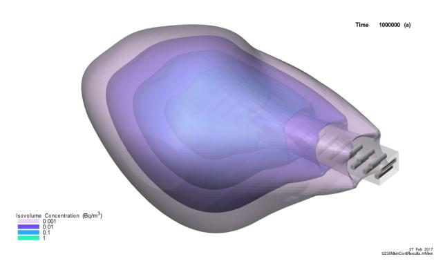
Figure 7-131: Main Container-Scale Model: Three-Dimensional Visualization of U-238 Concentration at 1 Ma
