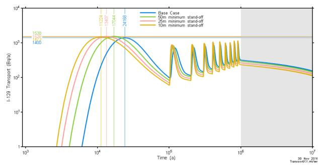
Figure 7-101: Rooms-Only Repository Scale Model: Fracture Location Sensitivity – I-129 Transport to the Well
