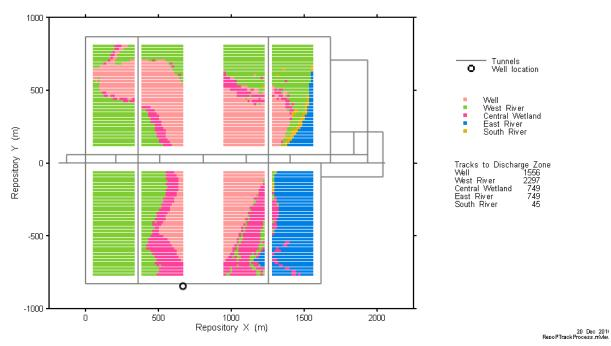
Figure 7-142: Repository-Scale Model: Origin and Discharge Locations of Advective Transport Pathways for a Well Demand of 911 m<sup>3</sup>/a
