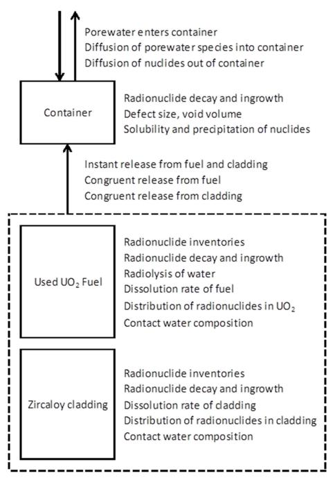
Figure 7-3: Conceptual Model for the Waste Form and Container
