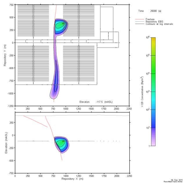
Figure 7-78: Full Repository-Scale Model: Base Case I-129 Concentration at 25 k Years
