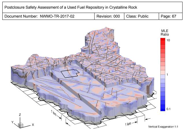
Figure 2-21: Ratio of MLE for a Doubling of Dispersivity Relative to the Reference Case
