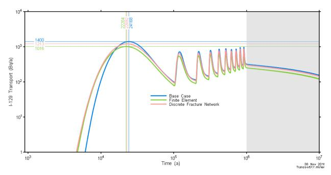
Figure 7-114: Rooms-Only Repository Scale Model: DFN Sensitivity – I-129 Transport to the Well
