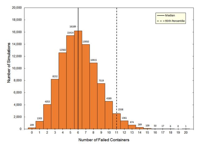
Figure 7-175: Probabilistic Assessment: Distribution of Container Failures with Container Assumptions Varying
