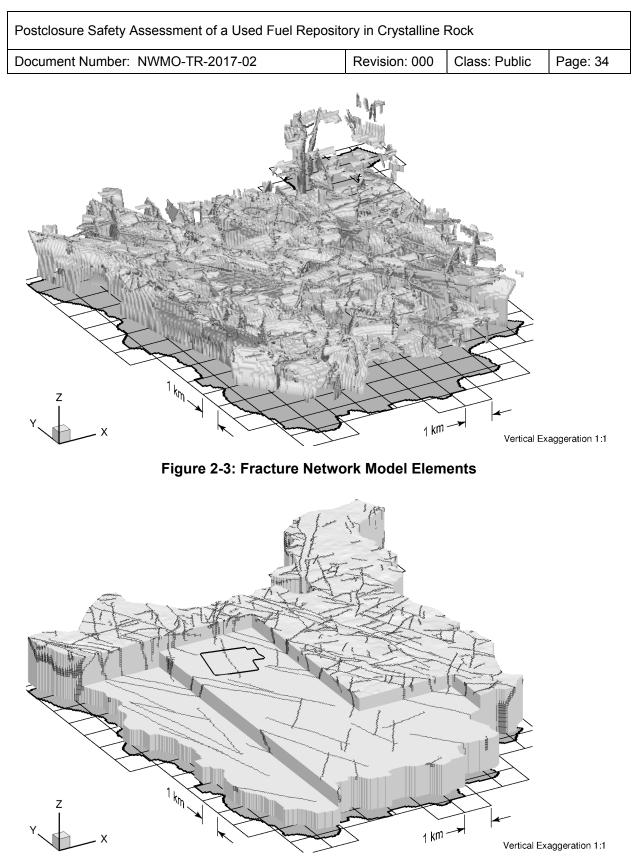
Note: Cut away sections are at 500 metres below ground surface (mBGS) and 1000 mBGS.
