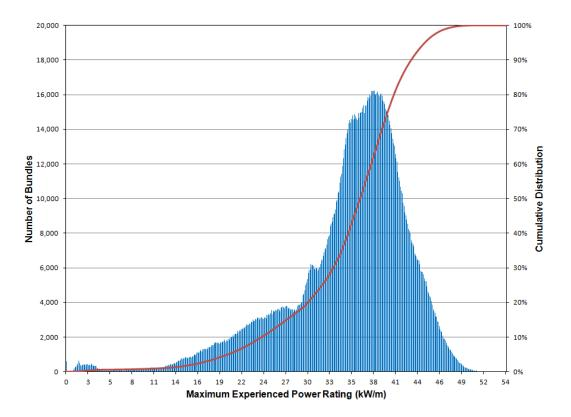
Note: The standard deviation of the distribution is approximately 7.4 kW/m or 140 kW/bundle. The figure is based on data in Wilk (2013).
