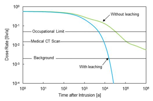
Figure 7-184: Inadvertent Human Intrusion: Effect of Leaching on Exposure to the Resident – Hazard Not Identified and Site Vacated after 14 Days
