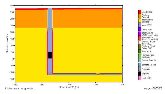
Figure 7-28: Full Repository-Scale Model: Vertical Visualization Showing Shaft and Seals
