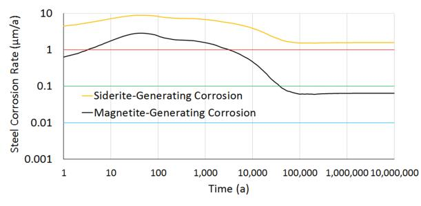
Figure 5-17: Evolution of Steel Corrosion Rates
