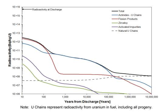
Figure 5-7: Radioactivity of Used CANDU Fuel (220 MWh/kgU burnup)
