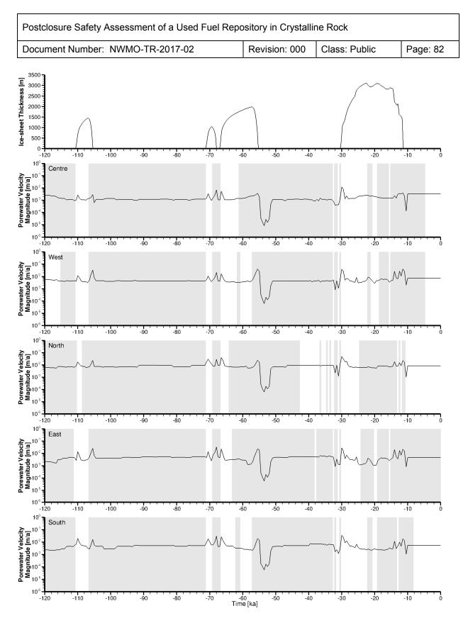
Figure 2-41: Velocity Magnitude versus Time for nn2008 Paleoclimate Boundary Conditions a loading efficiency of 1 and a 0% of ice-sheet thickness equivalent freshwater head for the surface hydraulic boundary condition (fr-base-paleo-0-le1)
