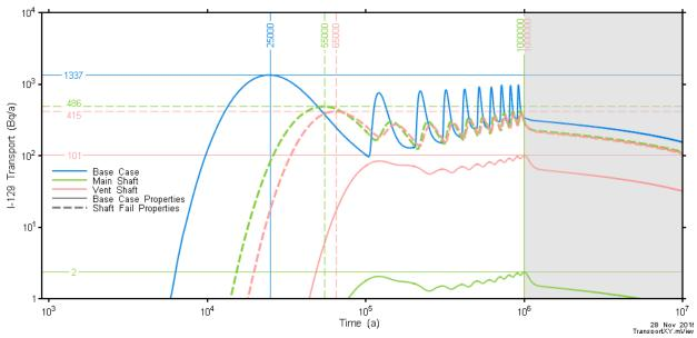
Figure 7-190: Full Repository Scale-Mode: Container Source Term – Main Shaft and Vent Shaft Fail Disruptive Event Scenarios - I-129 Transport to the Well
