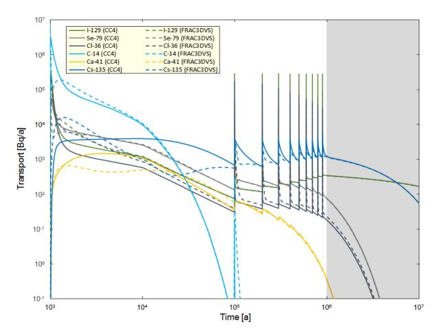
Figure 7-147: System Model, Simple Geosphere Submodel: Comparison of I-129, C-14, Ca-41, CI-36, Cs-135 and Se-79 Transport to the Geosphere
