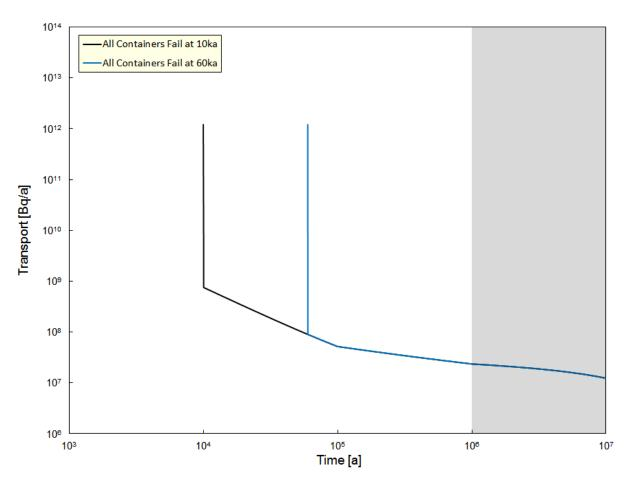
Figure 7-18: I-129 Source Term for the All Containers Fail Cases
