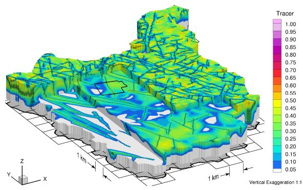
Figure 2-33: Tracer Migration at 120,000 Years for nn2008 Paleoclimate Boundary Conditions and a Loading Efficiency of 1 (fr-base-paleo-le1)
