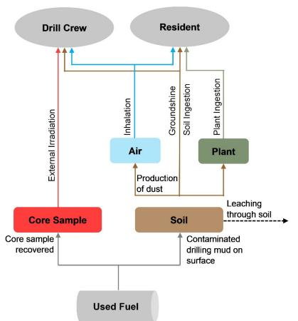
Figure 7-179: Inadvertent Human Intrusion - General Conceptual Model
