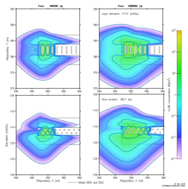
Figure 7-129: Main Container-Scale Model: U-238 Concentration at 500.5 and 1 Ma
