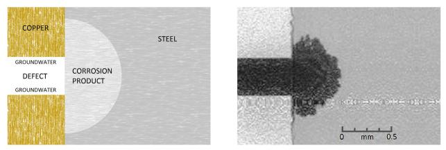
Note: The left panel represents a conceptual illustration and the right micrograph shows early results from laboratory experiments that have been accelerated by utilizing a free-flowing solution, purged with oxygen.
