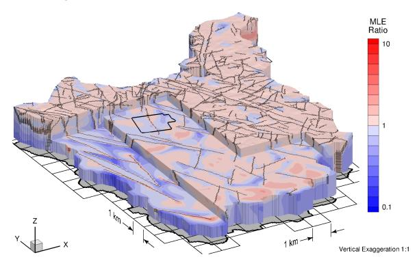
Figure 2-20: Ratio of MLE for an Order-of-Magnitude Increase in the Diffusion Coefficient Relative to the Reference Case
