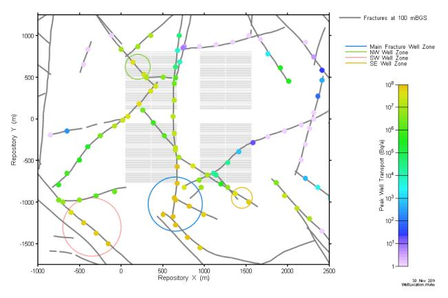
Figure 7-69: Rooms Only Repository-Scale Model: Peak Well Transport at Test Well Locations and Spatial Zone Identification
