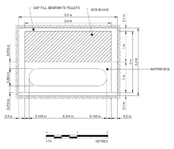
Figure 4-16: Placement Room Geometry (Vertical Section)
