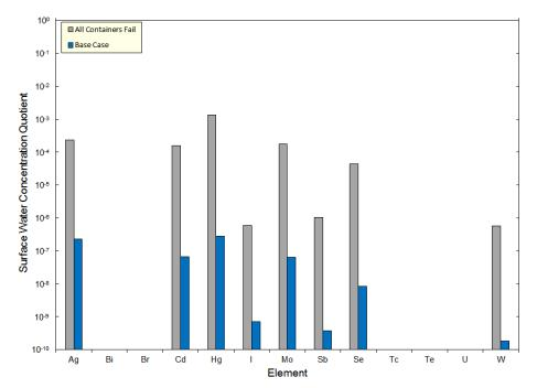
Figure 7-196: Non-Radiological Hazard: Groundwater Results
