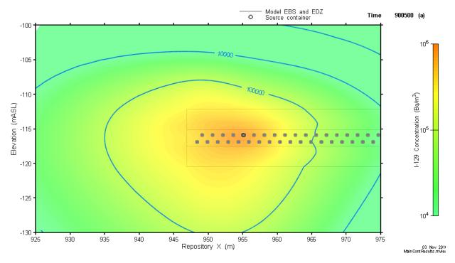
Figure 7-119: Main Source Container-Scale Model: Detail of I-129 Concentration 500 Years after the Failure of the Tenth Container (at 900,500 a)
