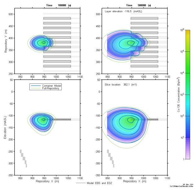
Figure 7-132: Main Container-Scale Model: Cs-135 Concentration at 100 and 500 ka
