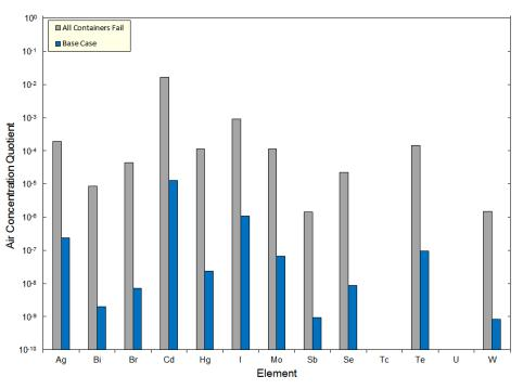
Note: Tc does not have an acceptance criterion in Air, U results are off scale low
