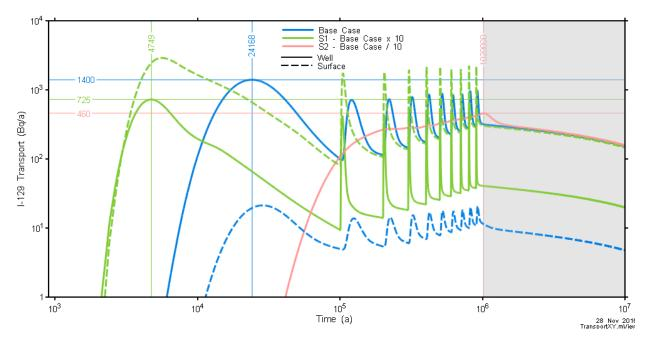
Figure 7-91: Rooms-Only Repository-Scale Model: I-129 Transport for Geosphere Hydraulic Conductivity Sensitivity Cases
