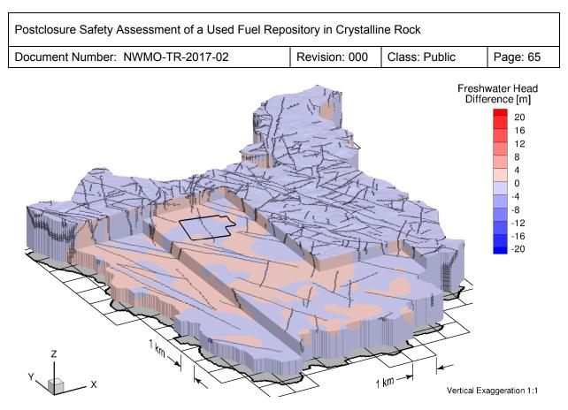
Figure 2-17: Difference in Freshwater Heads between the EPM Case and the Reference Case
