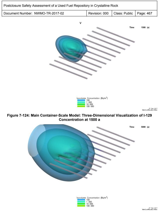
Figure 7-125: Main Container-Scale Model: Three-Dimensional Visualization of I-129 Concentration at 5000 a
