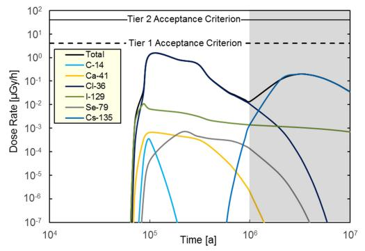
Note: C-14 and CI-36 dose rates result from the sum of releases originating from both the fuel and the fuel sheath.
