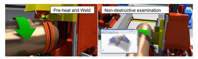
Figure 4-10: Weld Worktable and Non-Destructive Examination Worktable
