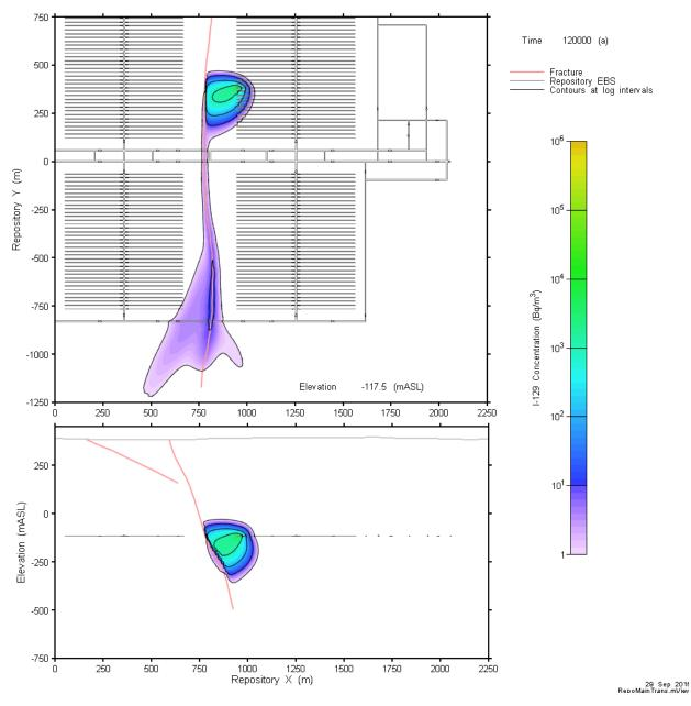
Figure 7-81: Full Repository-Scale Model: Base Case I-129 Concentration at 120,000 Years
