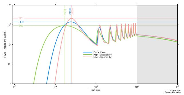
Figure 7-107: Rooms-Only Repository-Scale Model: Dispersivity Sensitivity – I-129 Transport to the Well
