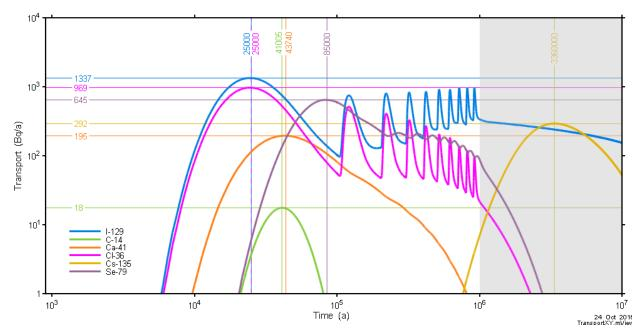
Figure 7-86: Full Repository-Scale Model: Base Case Transport to the Well for all Radionuclides
