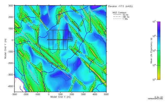
Figure 7-40: Subregional-Scale Model: Base Case (No Well) - Mean Life Expectancy (a) at Repository Elevation
