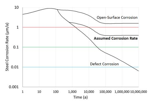
Note: This figure illustrates siderite-generating corrosion.
