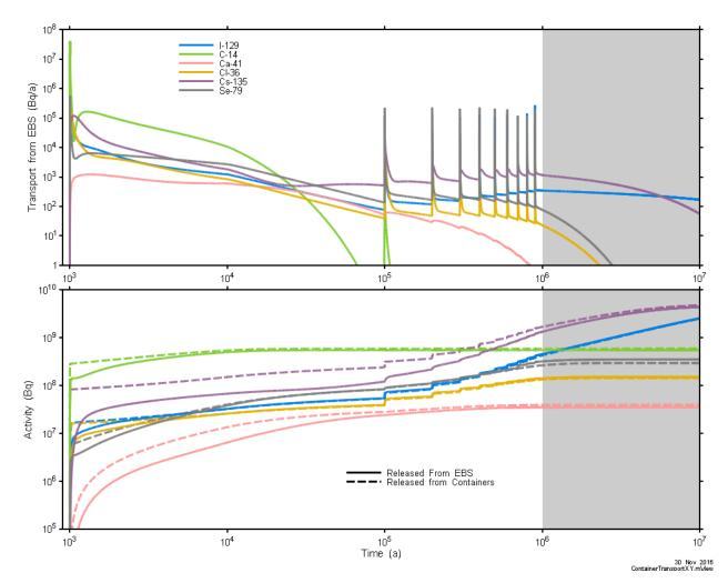
Figure 7-134: Main Container-Scale Model: Transport Rates and Cumulative Release for I-129, C-14, CI-36, Ca-41, Se-79, and Cs-135
