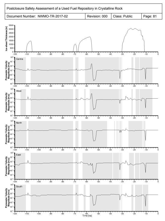
Figure 2-40: Velocity Magnitude versus Time for nn2008 Paleoclimate Boundary Conditions and a Loading Efficiency of 0 (fr-base-paleo-le0)
