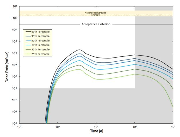
Figure 7-174: Probabilistic Assessment: Time Dependence of Percentile Values with Container Assumptions Fixed
