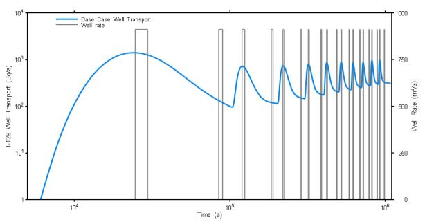
Figure 7-87: Rooms-Only Repository-Scale Model: Intermittent Well Sensitivity - Schedule
