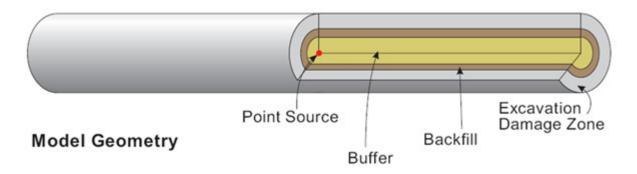
Note: the backfill thickness is 0 cm in the repository model used in this study.
