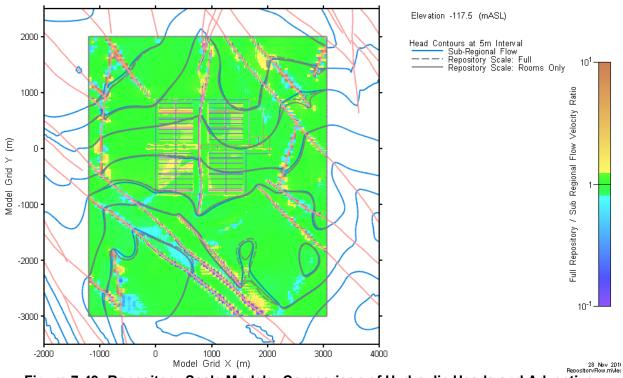
Figure 7-49: Repository-Scale Models: Comparison of Hydraulic Heads and Advective Velocities with Subregional-Scale Model at Repository Elevation
