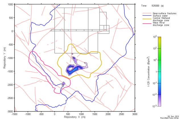
Figure 7-85: Full Repository-Scale Model: Base Case Surface Discharge Concentration at Time of Peak I-129 Transport (925 ka)
