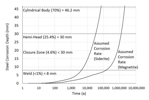
Figure 5-20: Evolution of Steel Corrosion Depth
