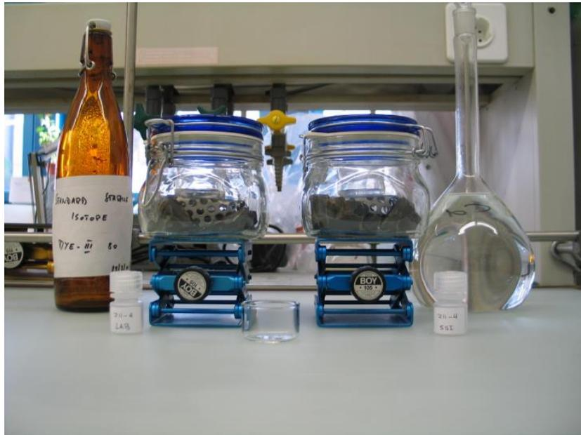
**Figure B-5: Isotope Diffusive Exchange Set-up Showing Rock Cores Enclosed in Sealed Containers and Equilibrating with Known Solutions Over the Vapour Phase**
