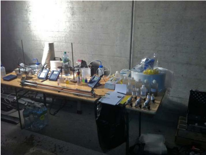
Picture 8: Field measurements devices and collected water samples; copper tubes are for noble gas measurements (Sa, 14.12.2013).
