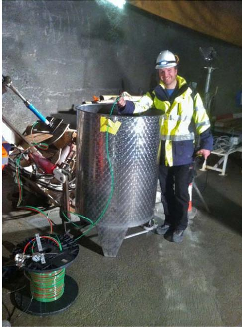
Picture 5: Collection of artesian outflow in 580 L barrel (Sa, 14.12.2013).
