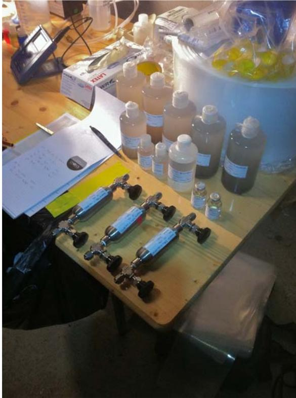
Picture 8: Collected water samples; note difference between samples filtered on-site (glass bottles for  $\delta^{13}\text{C}$  and 2 HDPE bottles in the middle) and unfiltered samples; steel cylinders are for  $^{14}\text{C}$  measurement (Sa, 14.12.2013).
