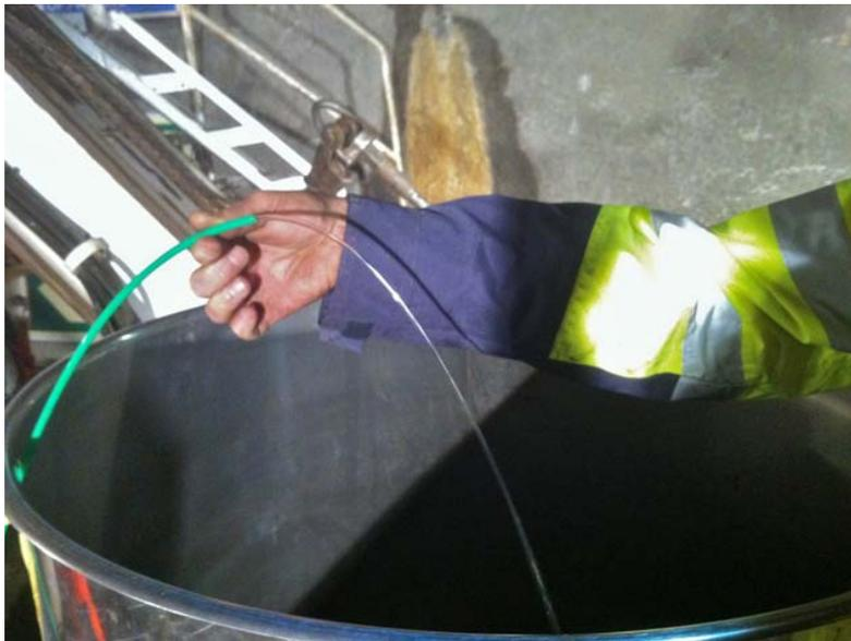
Picture 4: Artesian outflow from lower water sampling line after packer inflation (Sa, 14.12.2013).
