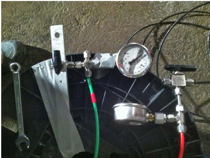
Picture 6: Manometer showing interval pressure of 7 bar after packer inflation (Sa, 14.12.2013).
