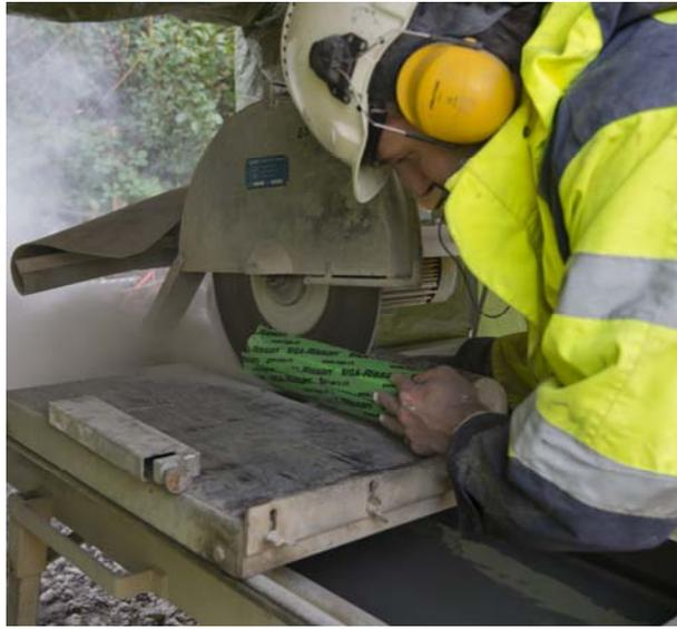
**Figure 3-3: Removal of the “Stratigraphy-slab” by Dry Cutting on Site Immediately after Core Recovery.**
