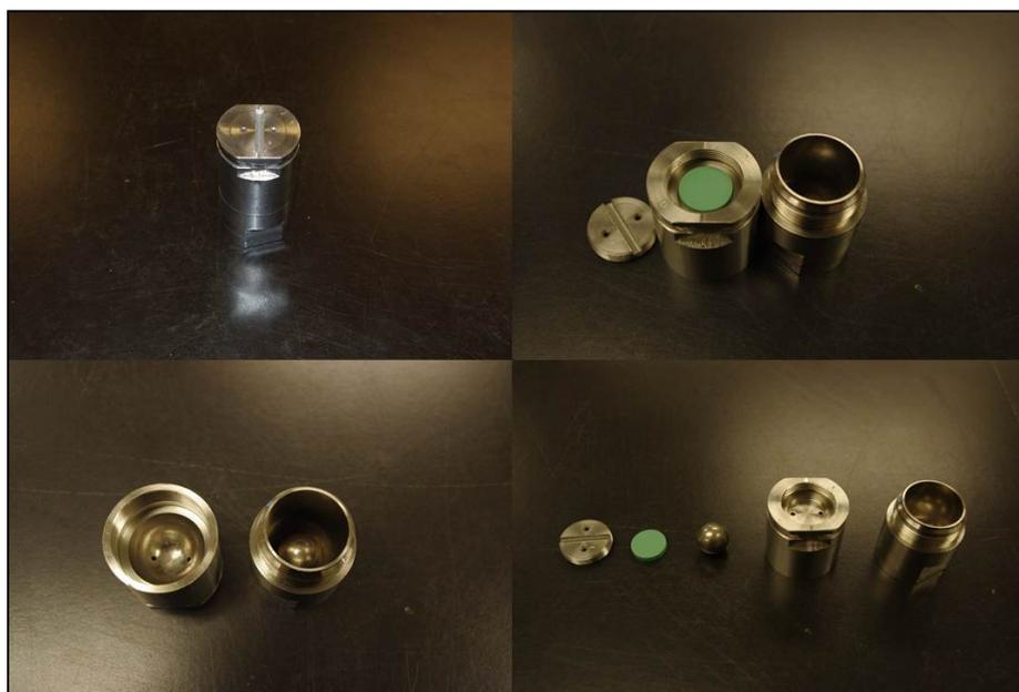
**Figure A.2. Individual Stainless Steel Sample Holder with High Temperature Septa (green) and Stainless Steel Ball; Sample Holders are ~3.5 x 6.5 cm**
