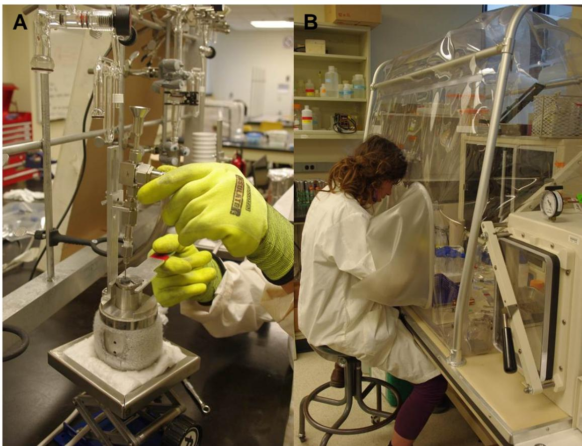
**Figure A.7. Aqueous Leaching Method: Following the Vacuum-distillation Experiment, the Needle/valve Unit and Sample Holder Containing the Dehydrated Rock is Detached From the Vacuum Line and Removed From the Heater With the Valve Closed (A). Once Cooled, the Sample Holder and Valve/needle Unit are Transferred to an Anaerobic Chamber for Aqueous Leaching (B)**
