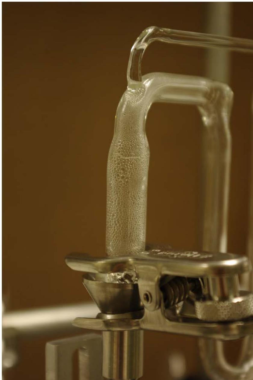
**Figure A.4. Condensation in the Vacuum Transfer Line (although rare) is Symptomatic of Loss of Vacuum, Resulting in Discarding of the Sample. This Problem is Mitigated by Performing a Dynamic Vacuum Extraction Using the U-trap**
