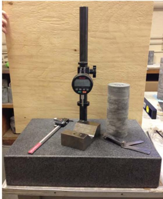
**Figure 5: Granite support surface, digital indicator, V-block, feeler gage, and the electronic caliper used for verification of the specimen dimensions**
