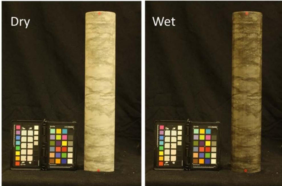
**Figure 7: Drilled cores are photographed in dry and wet (surface) conditions**
