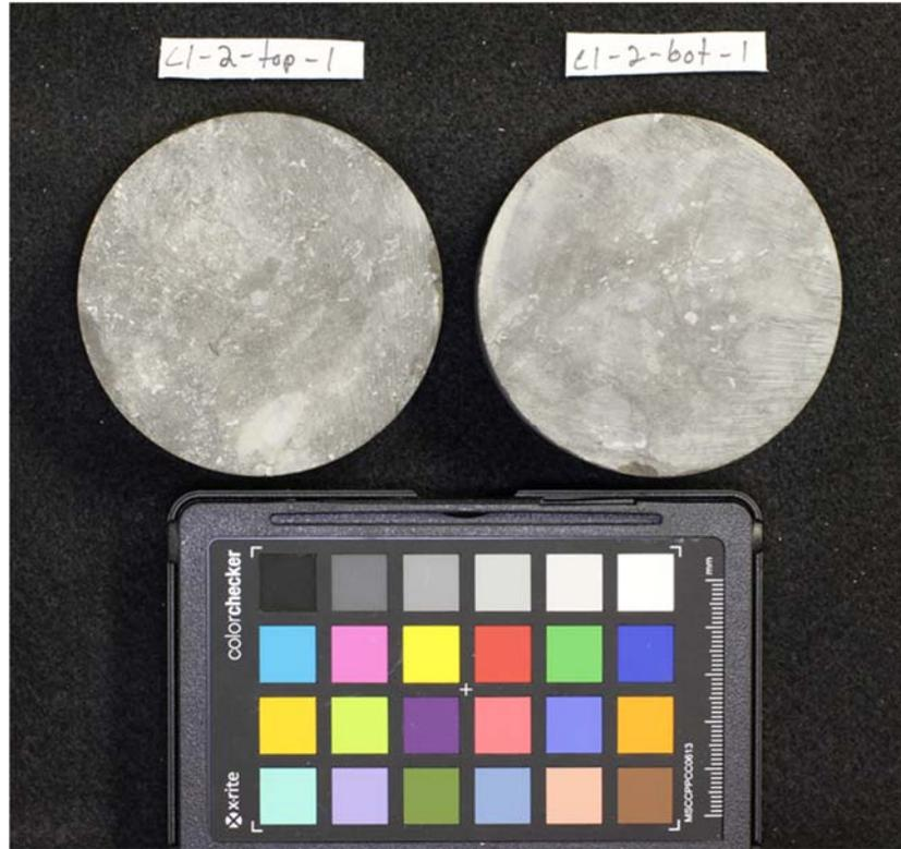
Figure 9: Photograph of the bottom of two prepared BTS specimens
