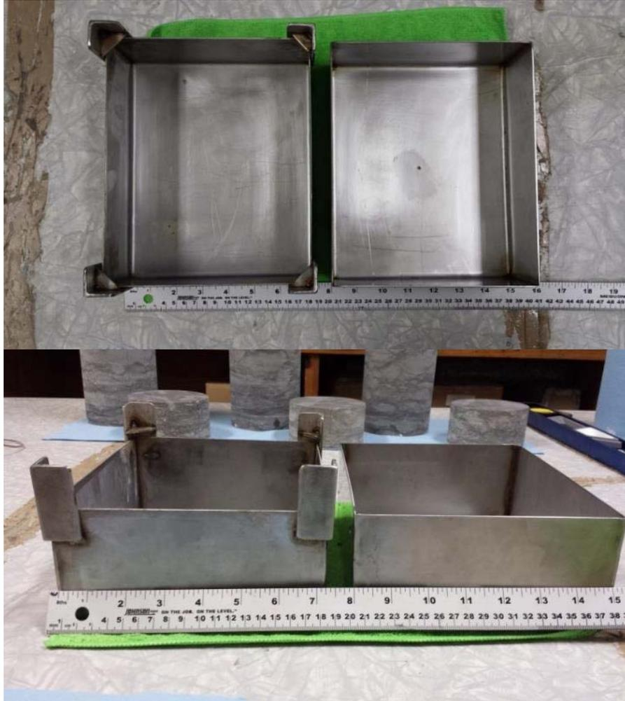
**Figure 12: Stainless steel trays used during vacuum saturation**
