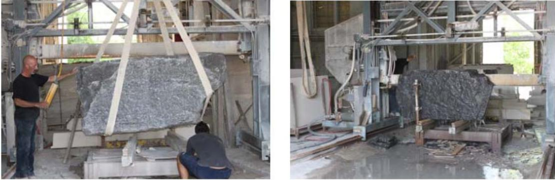
**Figure 2: Water-cooled cutting of Cobourg blocks using a flexible chain saw at Pierrexpert, Montreal**
