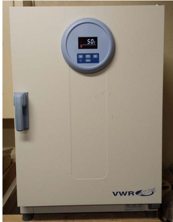
**Figure 13: VWR oven used to dry UCS and BTS specimens**
