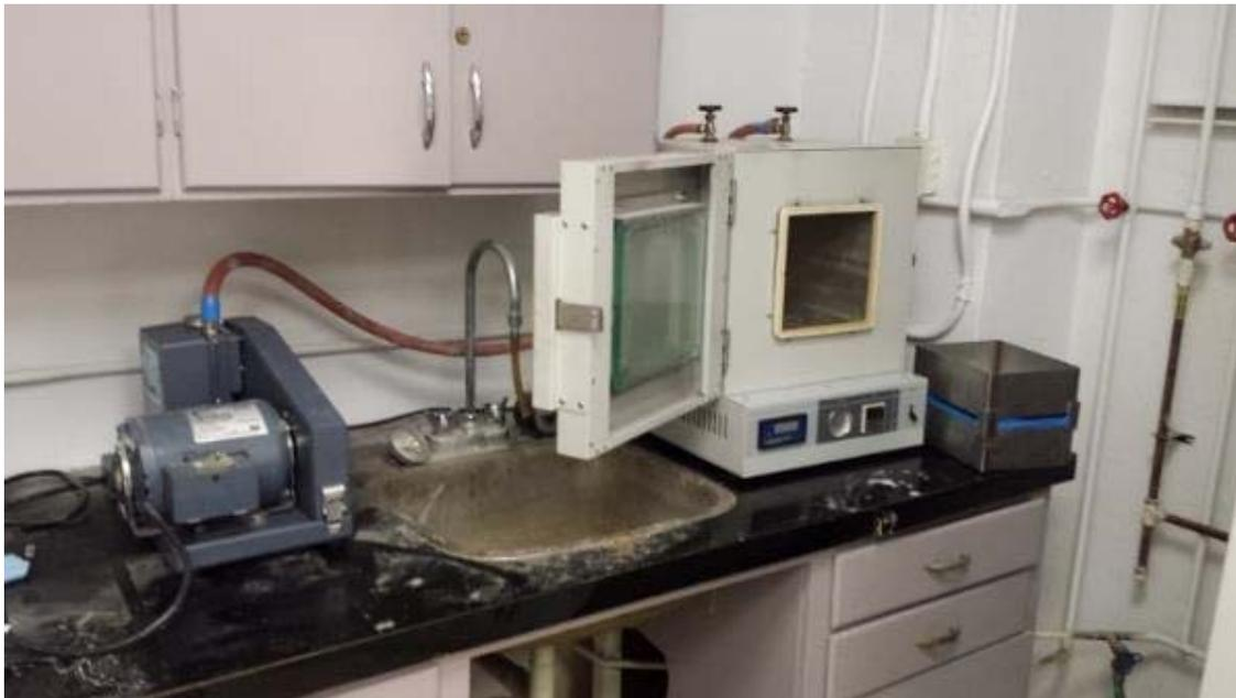
**Figure 11: Apparatus used for vacuum saturation of the specimens**
