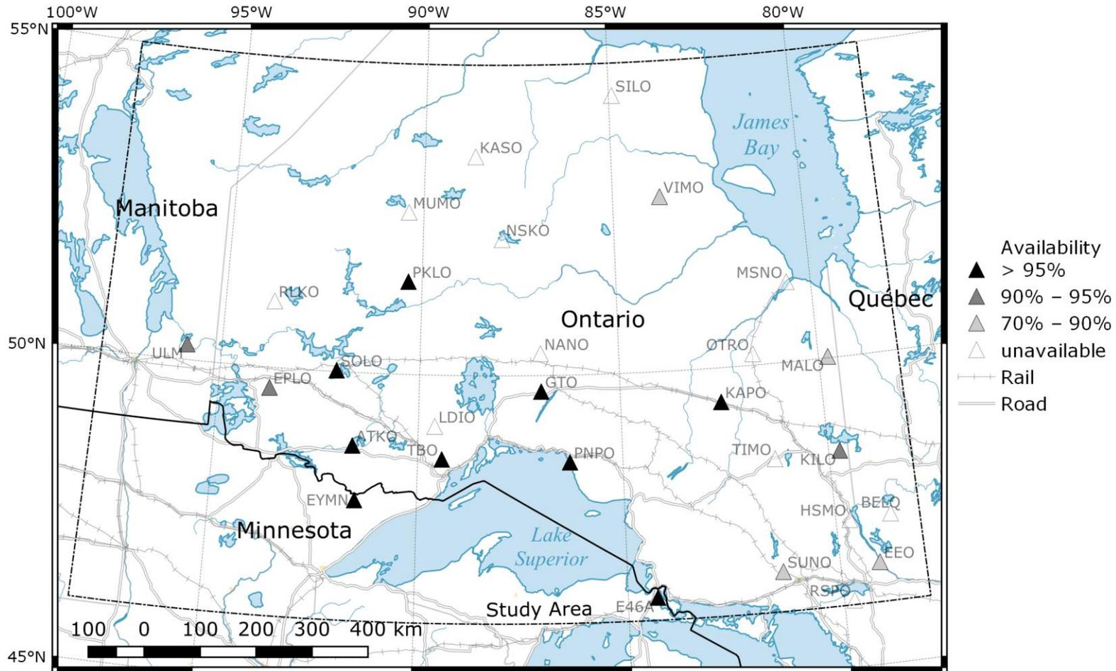
**Figure 1: Seismograph Stations in northern Ontario.** The study area is outlined with a dash-dotted line. Historical and currently active stations are shown as triangles, with the triangle filled according to data availability. Stations with no availability in northern Ontario are closed, former FedNor stations, mainly active 2006–2009. Historical analog stations are not shown.
