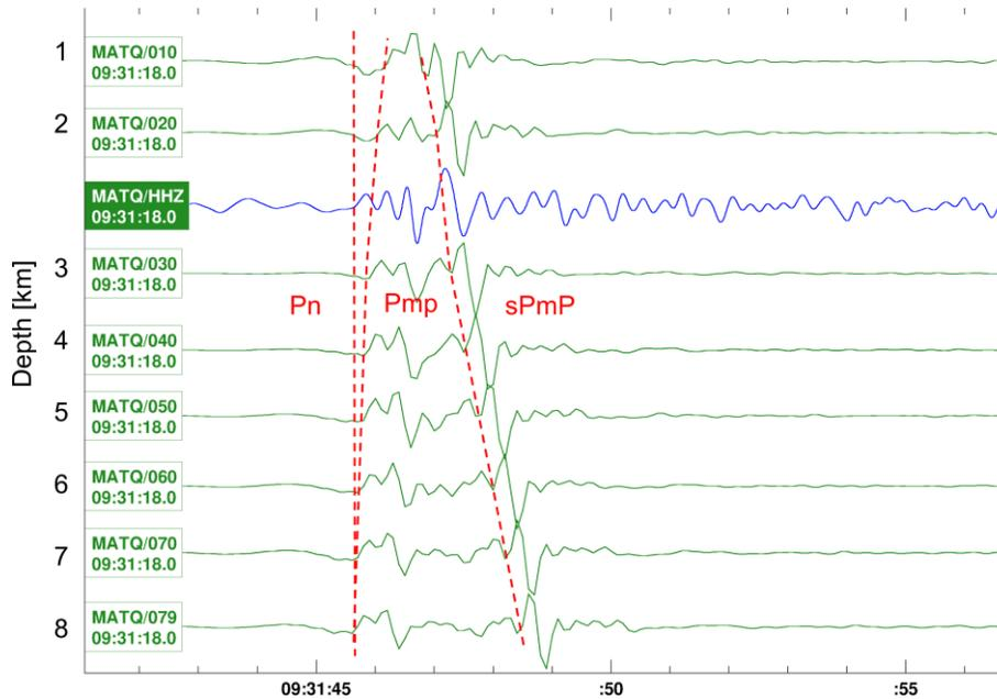
b) Waveforms at station MATQ, 178 km from epicentre, filtered using 0.7–3.5 Hz 6<sup>th</sup> order bandpass. Best fit depth 2.5 km.
