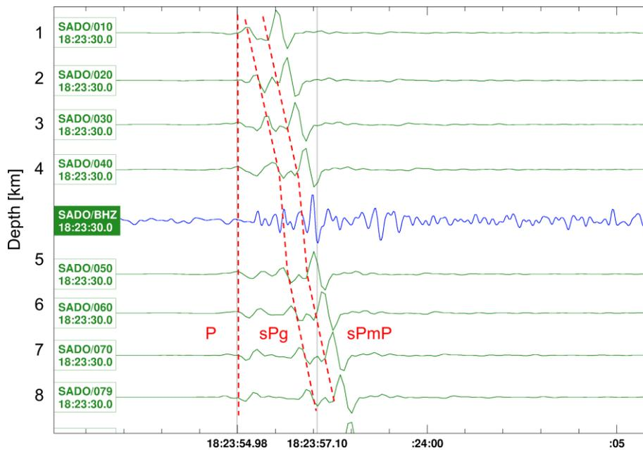
b) Waveforms at station SADO, 156 km S of epicentre, filtered using 1.2–6 Hz fifth order bandpass. Best fit depth 5.0 km. sPmP is better developed than sPg.
