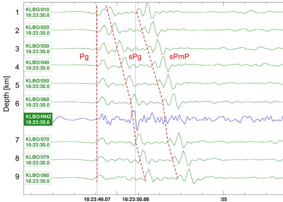
a) Waveforms at station KLBO, 121 km SW of epicentre, filtered using 1–6 Hz fifth order bandpass. Best fit depth 6.0 km. sPg is better developed than sPmp.
