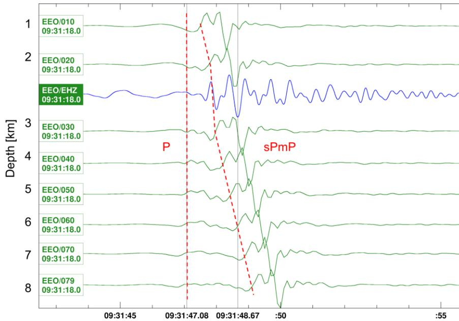
a) Waveforms at station EEO, 185 km from epicentre, filtered using 0.5–3.5 Hz 6<sup>th</sup> order bandpass. Best fit depth 2.5 km.
