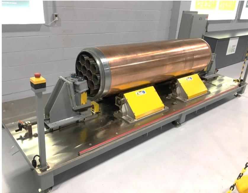
**Figure 3-5: UFC NDE Bench installed at NWMO's Engineering Test Facility**
