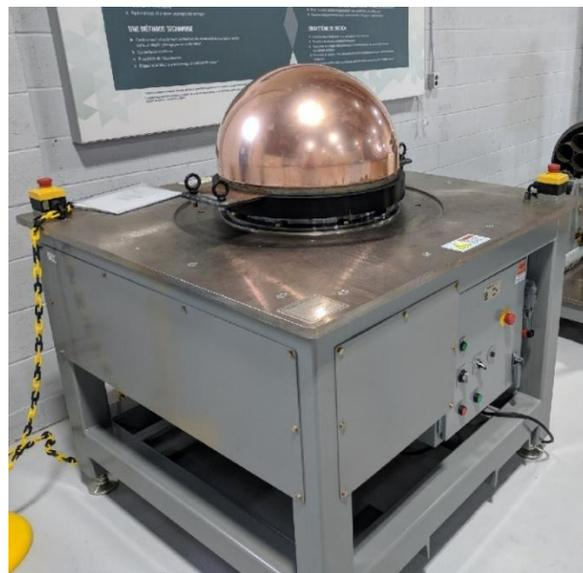
**Figure 3-6: Hemi-head NDE Bench installed at NWMO's Engineering Test Facility**
