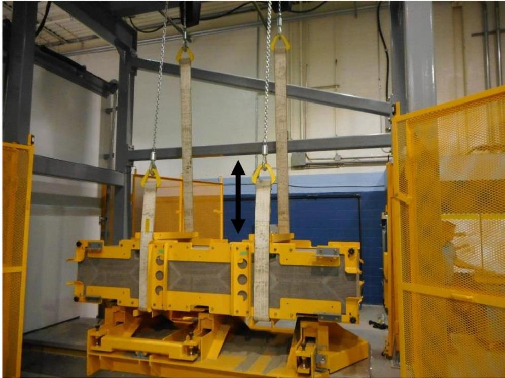
Figure 3-20: Rotation Jig for Shaping Cell
