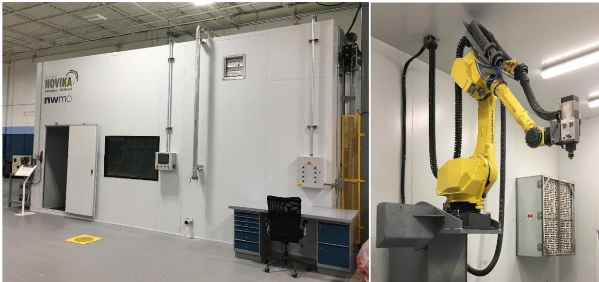
Figure 3-21: Shaping Cell and Milling Robot
