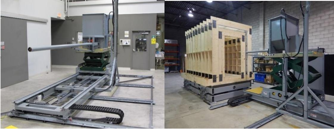
**Figure 3-17: (Left) Prototype GFM Screw Conveyor and (Right) Full scale GFM Test Frame and Prototype Screw Conveyor**
