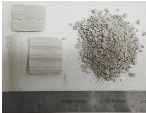
**Figure 3-16: Compacted (left) and Granulated (right) Gap Fill Material**
