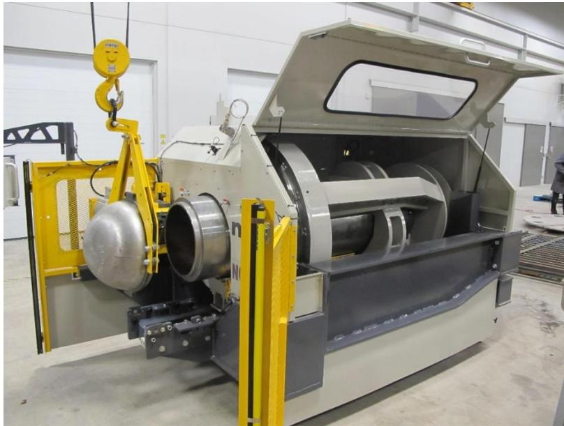
**Figure 3-4: ROTEQ 2.0 System with Viewing Panel Open (UFC Steel Hemi-Head and Shell Section Visible)**
