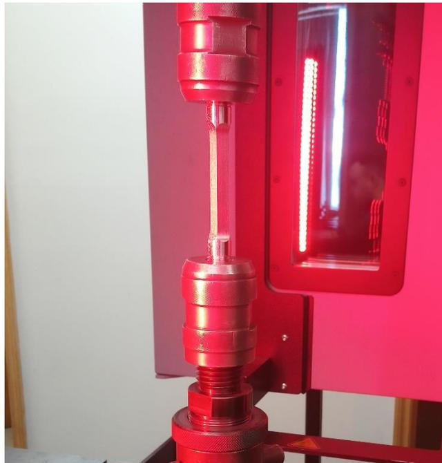
**Figure 3-1: Tensile Test Equipment to Obtain the True Stress-Strain Relationship from Initial Load to Fracture at Cambridge Materials Testing Ltd**
