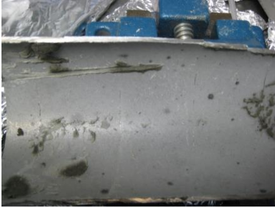
Once all sections were removed the second half of the filter was swabbed.
