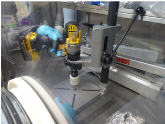
Coring device attached to electric drill inside the glovebox.
