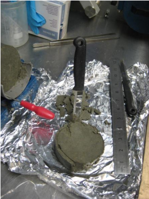
Outer layer of bentonite was removed from sections 1 to 4 and collected as a composite in one bag.
