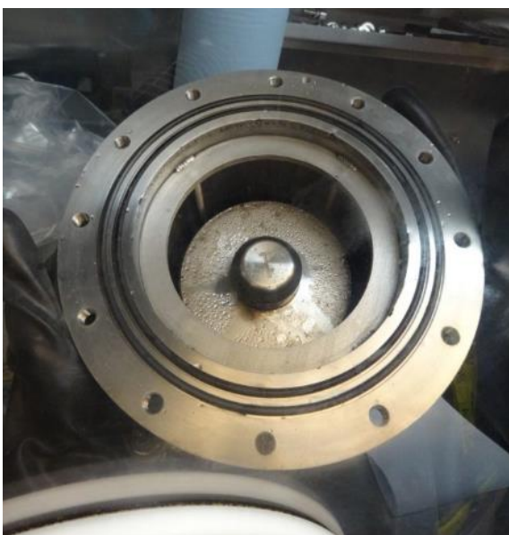
Top of module was swabbed before removing from shipping flask.
