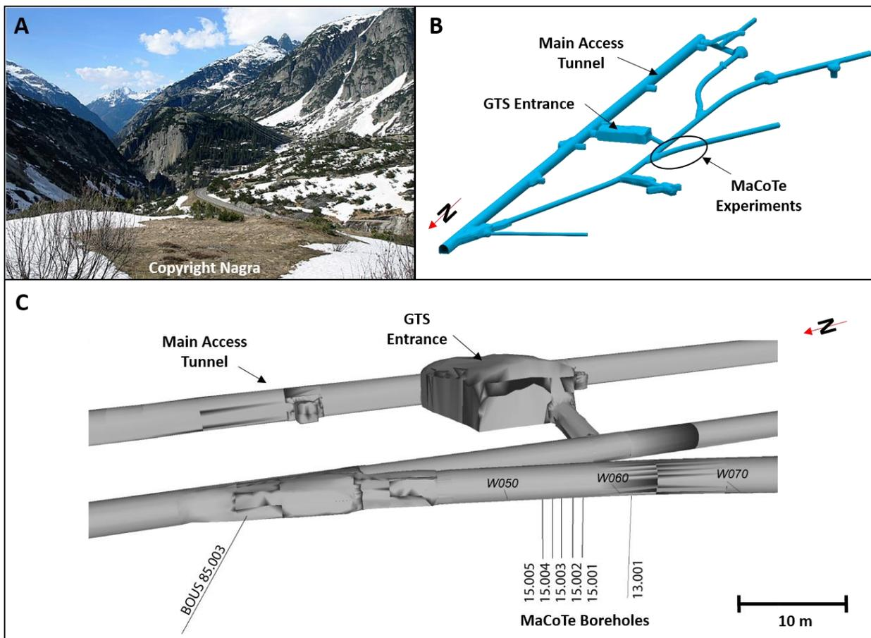
**Figure 1: A. View from the access tunnel used to enter the Grimsel Test Site showing the surrounding Swiss Alps mountains. B. Layout of the Grimsel Test Site underground research laboratory with the location of the MaCoTe project indicated (map taken from [www.grimsel.com](http://www.grimsel.com)). C. The specific locations of the MaCoTe boreholes (13.001 and 15.001 – 15.005) within the underground research laboratory. Drilling water was sourced from BOUS 85.003.**
