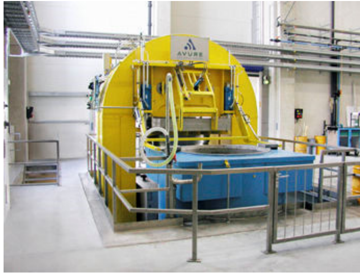
Figure 4-14: Cold Isostatic Press for Production of Highly Compacted Bentonite Blocks
