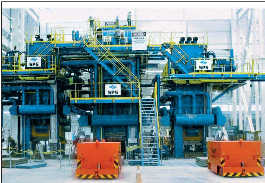
Figure 4-13: Example of a Closed-Die Forging Press (Uniaxial Compaction)
