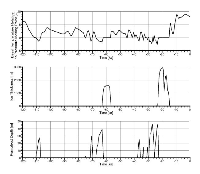
Figure 3-5: University of Toronto Glacial System Model Outputs for Simulation nn9930 at the Hypothetical Site of 7CS Repository (adapted from NWMO 2018, Section 2)
