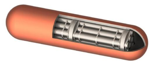
Figure 3-8: Cutaway Illustration of a Filled Mark II Container
