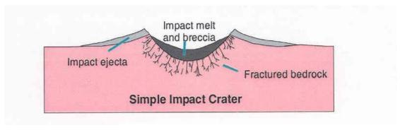
Note: In the base case of Wuschke et al. (1995), the bottom of the melt and breccia layer is approximately at repository level, i.e., 500 m below the original surface, and the rock below the repository level is fractured by the meteorite impact.
