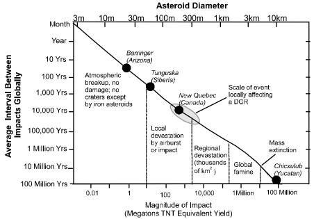
Note: Shaded region indicates the approximate magnitude of events that would produce a crater and shattered rock to a depth of 500 to 1000 m. For any given meteor impact, the chance of the impact occurring on the repository itself would be approximately 1 in 100 million, based on the size of the repository relative to the earth's surface area. Adapted from Morrison et al. (1994).
