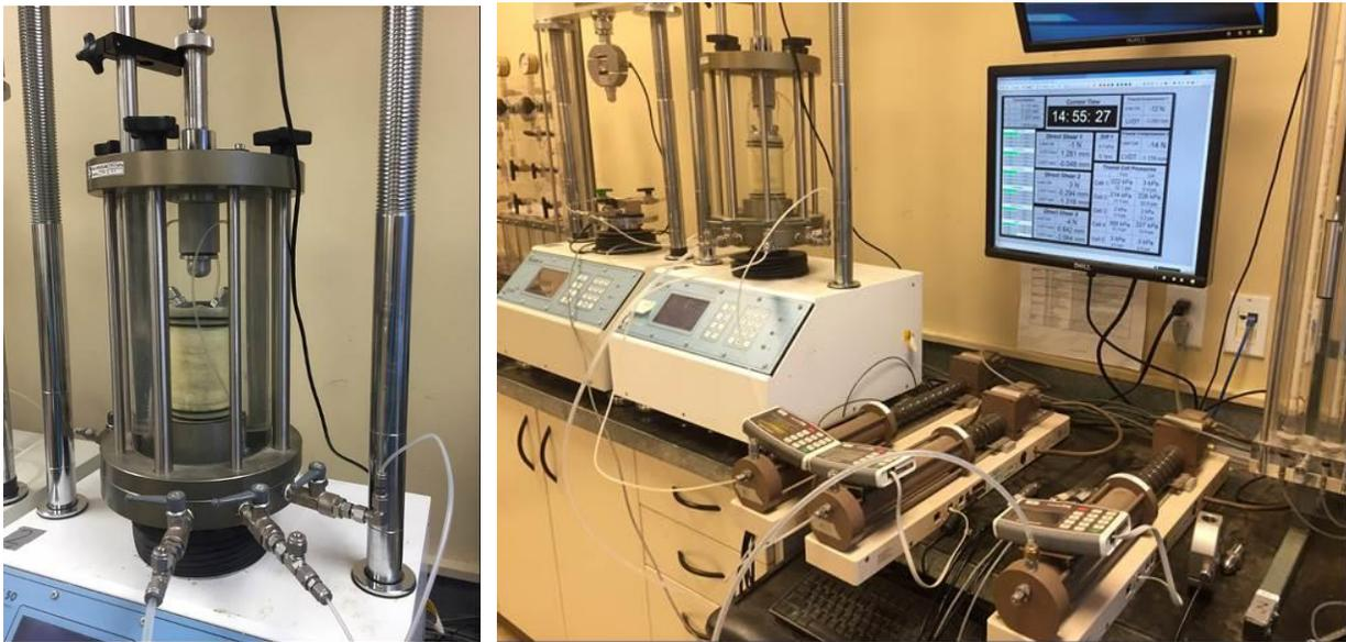
**Figure 7.13: Specimen Installed in Triaxial Cell for Air Permeability Testing and Test Apparatus in Operation**
