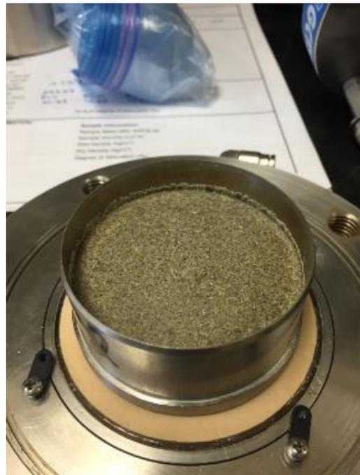
**Figure 7.6: GCTS Apparatus Used to Measure the SWCC in Low Suction Range and MX80 SWCC Specimen in Ring After Test.**
