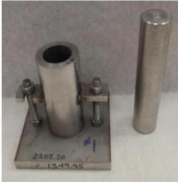
Figure 3.1 : Miniature Compaction Device (Priyanto et al. 2013)
