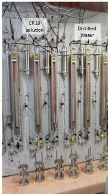
**Figure 6.1: Test Cells and Flow Gauges Used to Measure Swelling Pressure and Hydraulic Conductivity (from Priyanto et al. 2013)**
