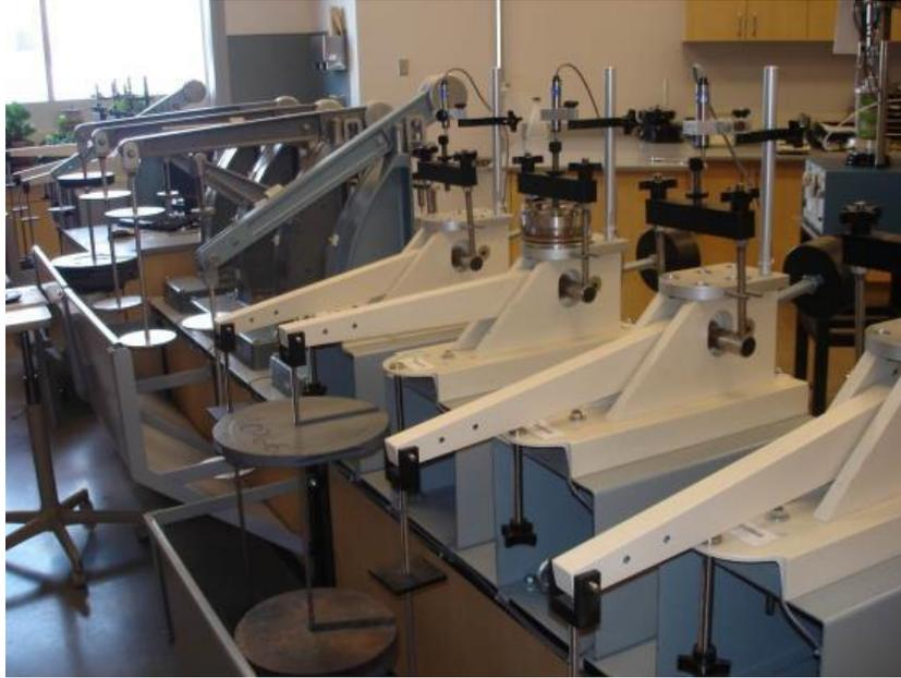
Figure 8.7: Lever-Arm Oedometers Used in 1-D Consolidation Testing.
