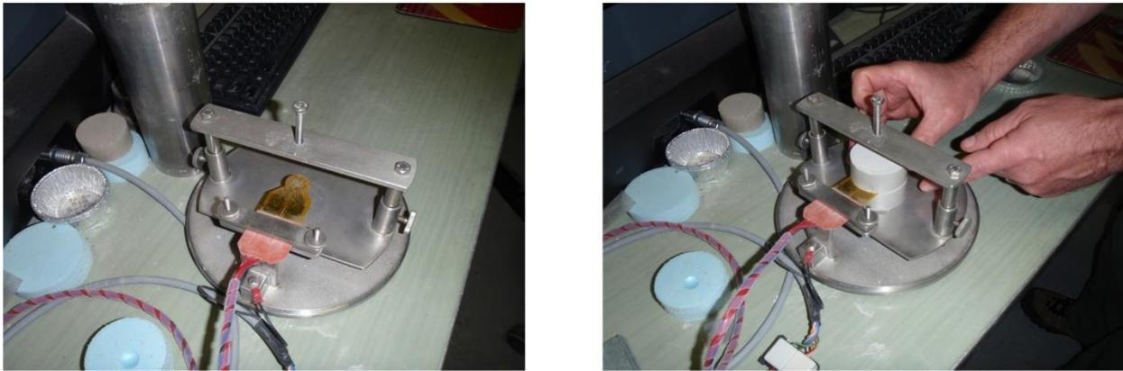
**Figure 9.2: Thermal Test Setup Showing Sensor and Specimen installation.**
