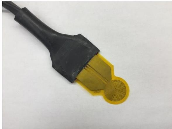
**Figure 9.1: Hot Disk Sensor Used in Current Thermal Testing**
