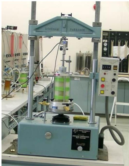
**Figure 8.1: Triaxial Test Apparatus at Golder's Mississauga Laboratory**
