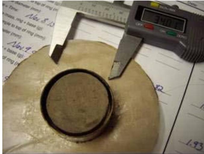
**Figure 7.1: Photograph Showing Shrinkage Specimen (Fredlund et al. 2012)**
