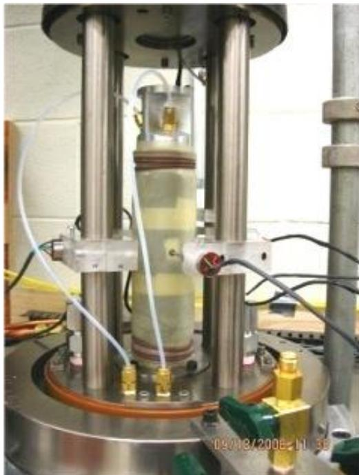
**Figure 8.3: Triaxial Test Apparatus used at RMC**
