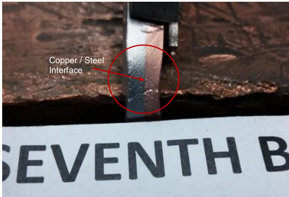
**Figure 3-11: Bend Test Sample Showing No Delamination of Electrodeposited Copper from the Steel after Several Cycles**
