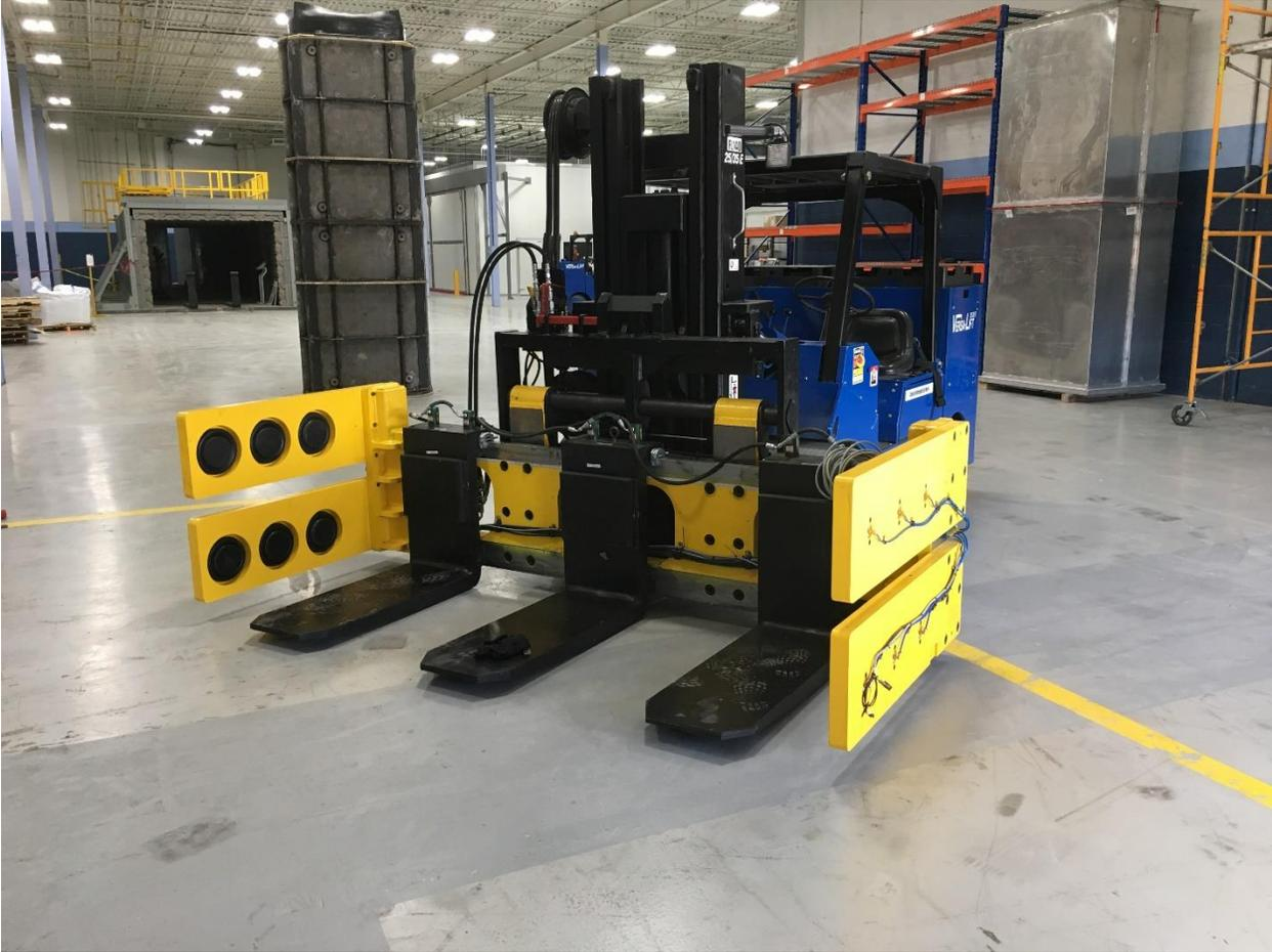
**Figure 3-18: Buffer Box Emplacement Attachment**
