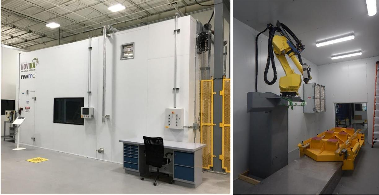
**Figure 3-20: Robotic Shaping Cell for Bentonite Blocks (Left – Enclosure, Right – Shaping Robot and Block Table)**
