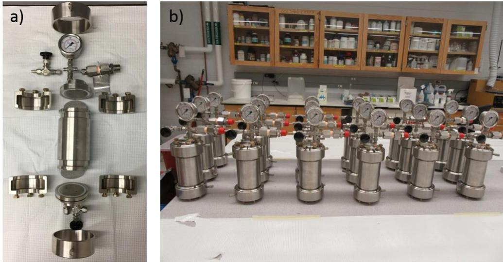
**Figure 3-23: a) Components of Pressure Vessels for Laboratory Bentonite/Microbiology Experiments at Western University. b) Set of Eighteen Pressure Vessels Used to Investigate a Variety of Physical and Chemical Parameters on Bentonite/Microbiology Properties.**
