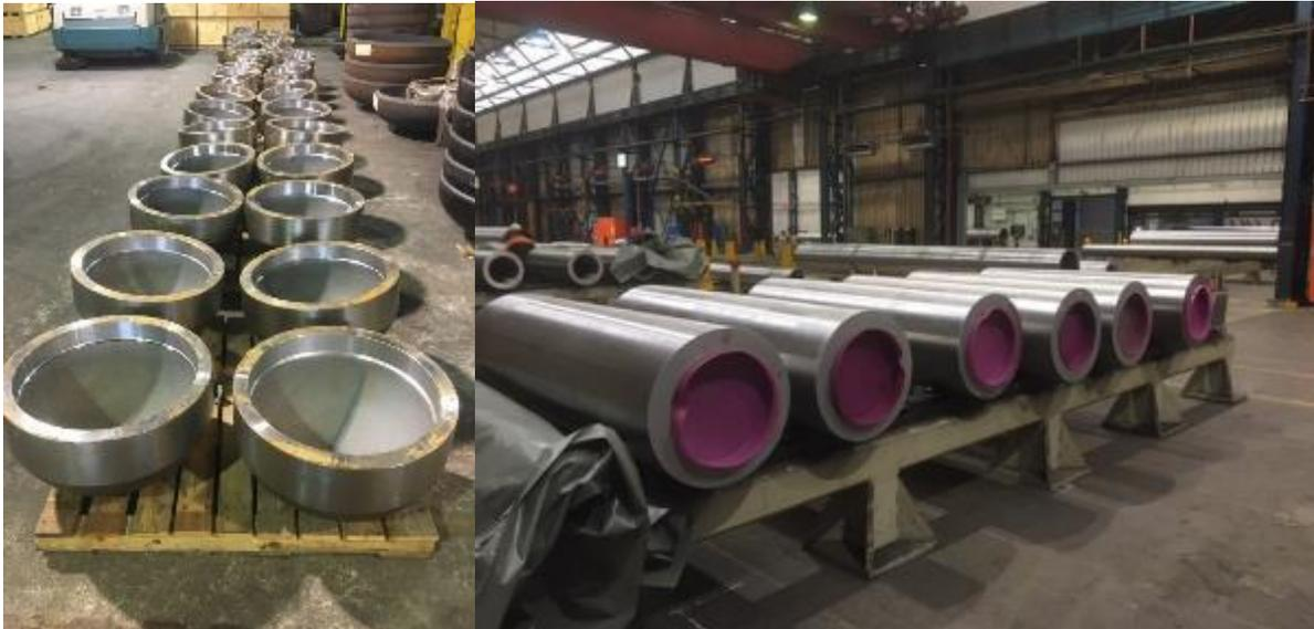
**Figure 3-6: Fabricated Hemi-Spherical Heads and Cylindrical Shells for the UFC Serial Production**
