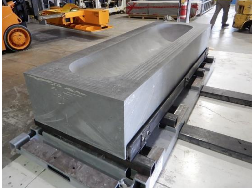
(c) HCB machined to fit UFC
