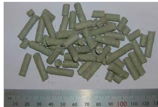
Extruded bentonite pellets of type used by SKB and Posiva (Johnsson & Sandén 2013)
