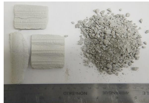
Dense bentonite chips and subsequently granulated materials considered by NWMO (Birch and Mielcarek 2017)
