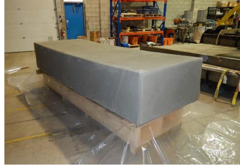
(b) HCB after machining to block size
