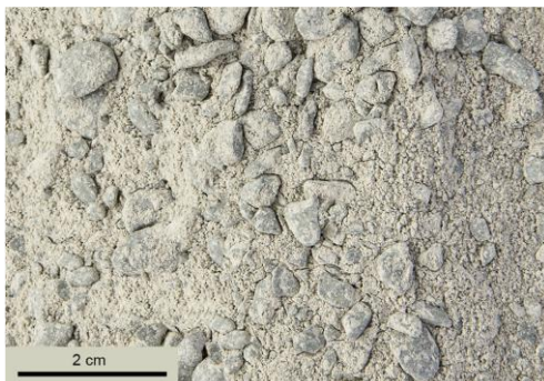
Granulated bentonite mixture considered by Nagra (Müller et al. 2017)
