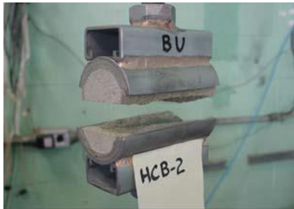
Figure 5-35: Pull-Test, Tensile Strength Measurement of HCB (Dixon et al. 2006)
