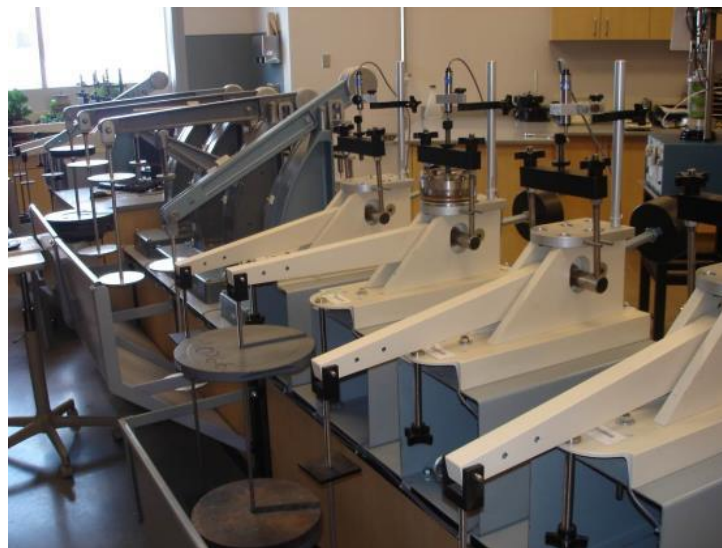
Figure 5-33: Lever-Arm Oedometers Used in 1-D Consolidation Testing (Dixon et al. 2018)
