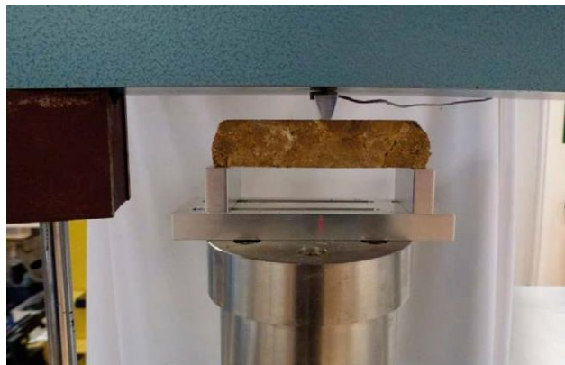
Figure 5-36: 3-Point Tensile Strength Test Setup (Eriksson 2016)
