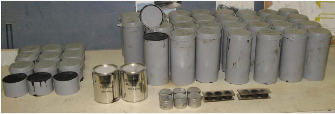
Figure 8-2: NWMO Asphalt-Based Materials Specimens for Testing
