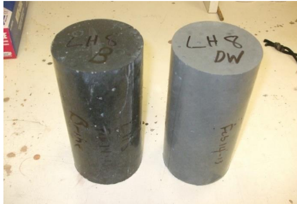
Figure 8-1: LHHPC Specimens After Curing in SR-270 (left) and Distilled (right) Waters
