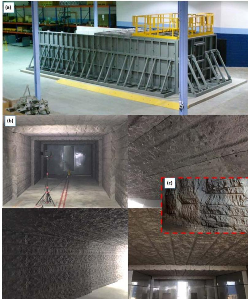
**Figure 4-6: Simulated Emplacement Room with Faux Rock Walls Simulated Drill And Blast Profile. (A) Exterior Steel Frame Approximately 3m X 3m X 15m in Size; (B) Interior With Faux Rock Walls and (C) Actual Blast Profile from Underground Research Laboratory**
