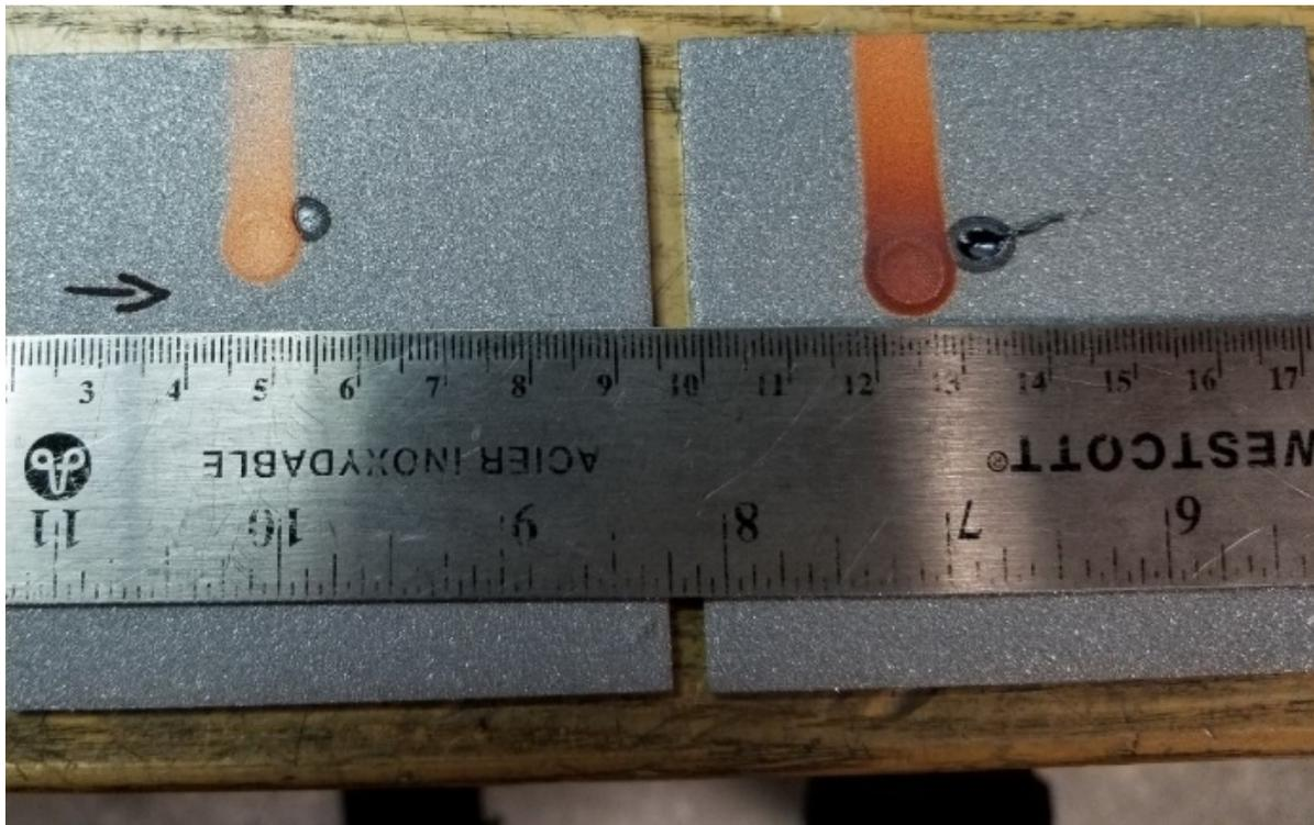
Note: The laser spot was positioned both to the right and to the top of the of the particle jet considering the dynamics of process.
