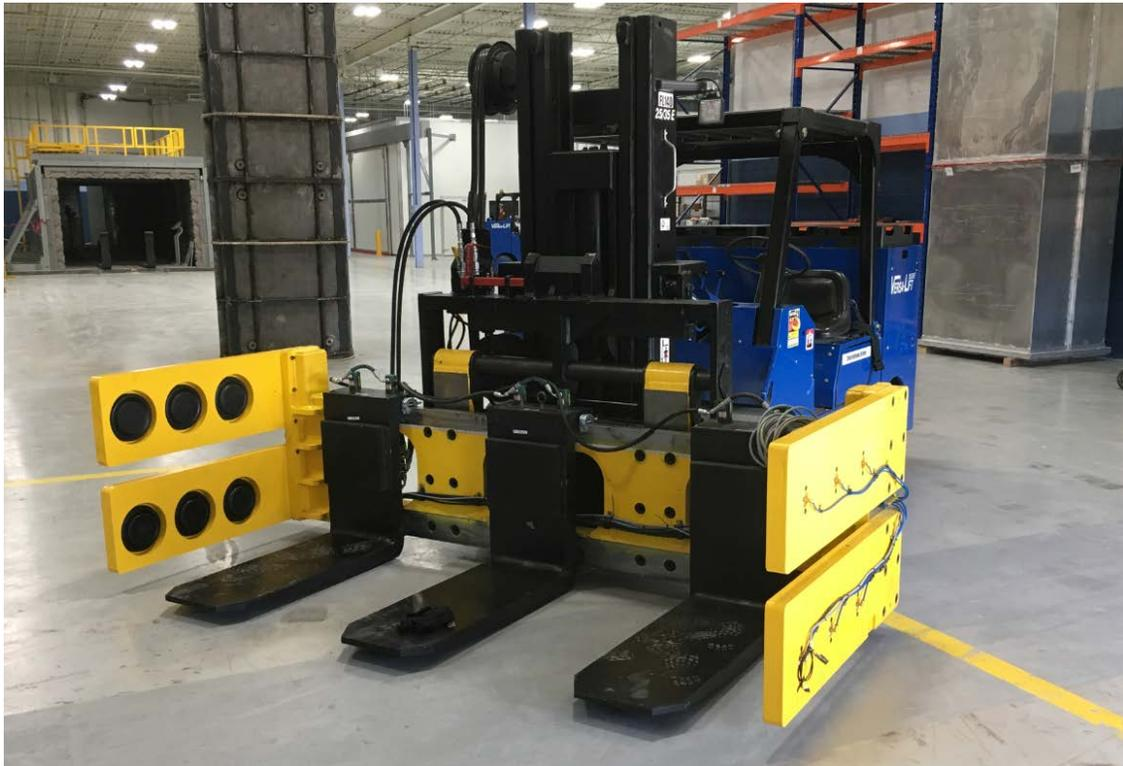
**Figure 4-7: Buffer Box Attachment installed on Versa Lift 25/35**
