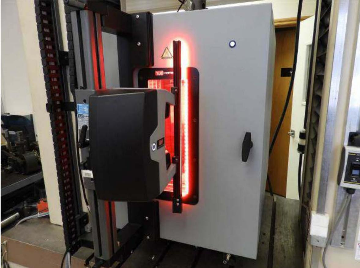
**Figure 3-16: UFC Carbon Steel Material Tensile Test Rig With Heating Chamber And Video Extensometer**
