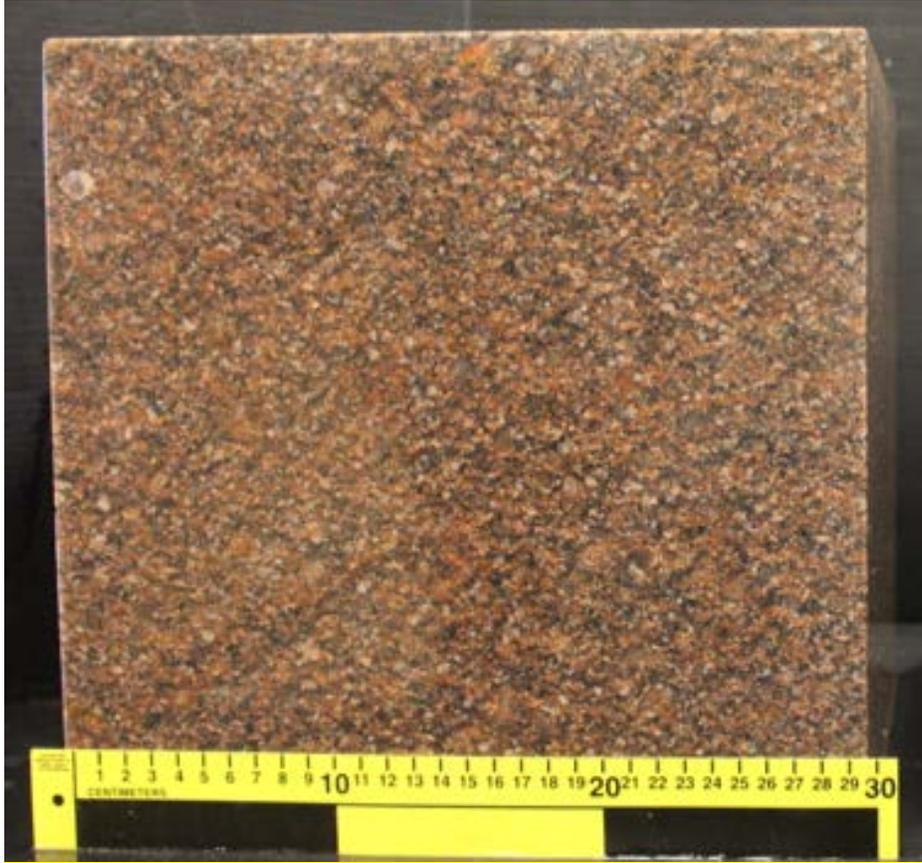
Figure 5-6: Cuboidal Sample of the Lac Du Bonnet Granite from the Canadian Shield
