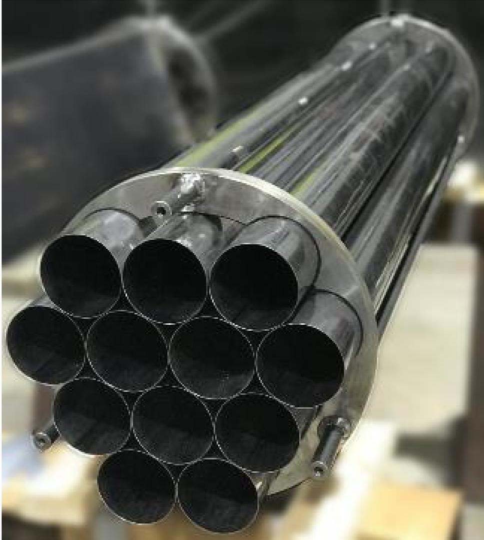
**Figure 3-3: Prototype 2018 UFC Insert Design**
