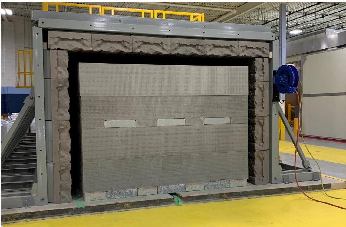
**Figure 4-10: Stacked Buffer Boxes with Fork Pockets (Top assembly)**
