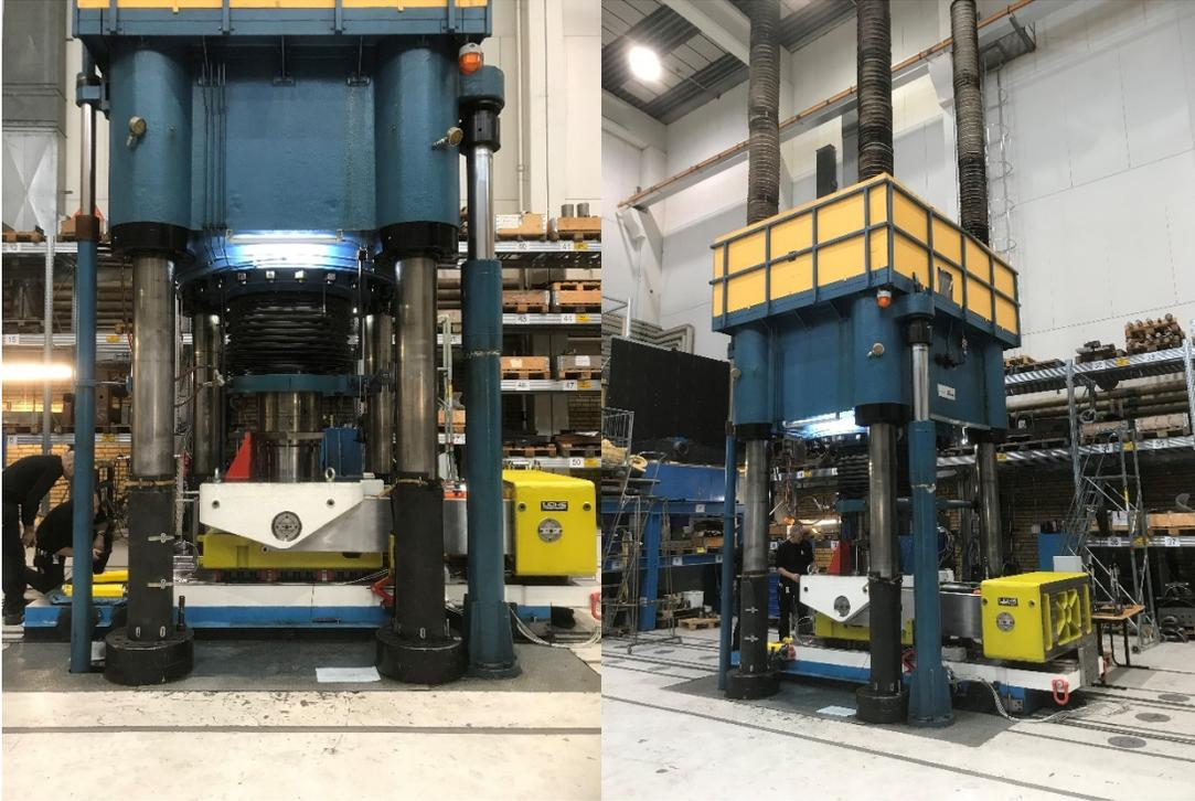
**Figure 5-11: New Shear Testing Equipment Integrated with Existing Laboratory Load Frame**
