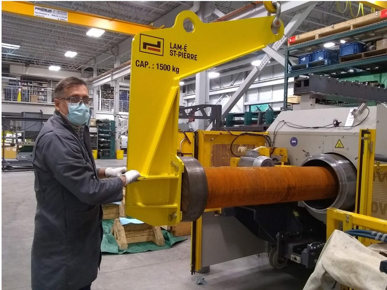
**Figure 4-5: Dummy Insert Being Loaded into Used Fuel Container (UFC) Lower Assembly Using a Custom Handling Tool at Welding Contractor Novika Solutions**
