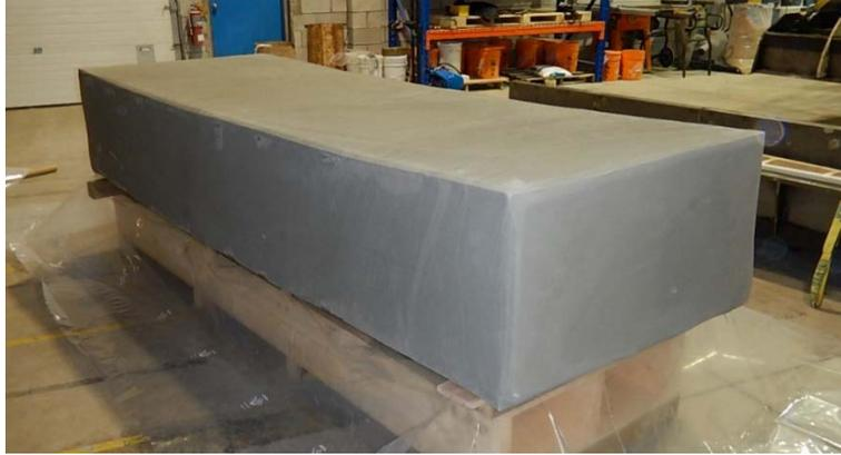
**Figure 3-11: Highly Compacted Bentonite (HCB) Block**
