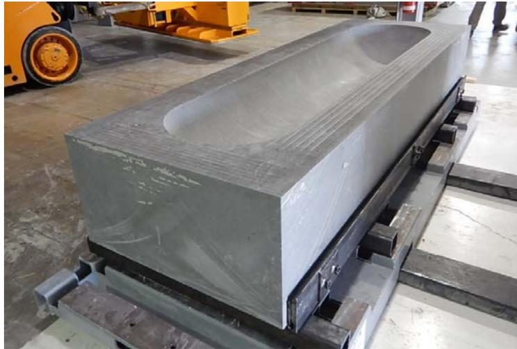
**Figure 3-12: Shaped Highly Compacted Bentonite (HCB) Block**
