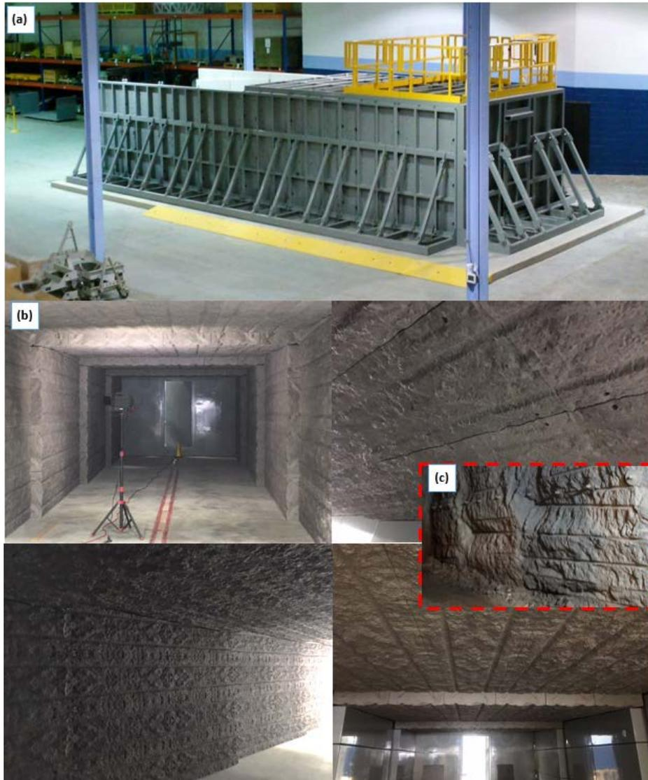
**Figure 3-16: Simulated Emplacement Room with Faux Rock Walls Simulated Drill and Blast Profile: (a) Exterior Steel Frame Approximately 3m x 3m x 15m in Size, (b) Interior with Faux Rock Walls and (c) Actual Blast Profile from Underground Research Laboratory**
