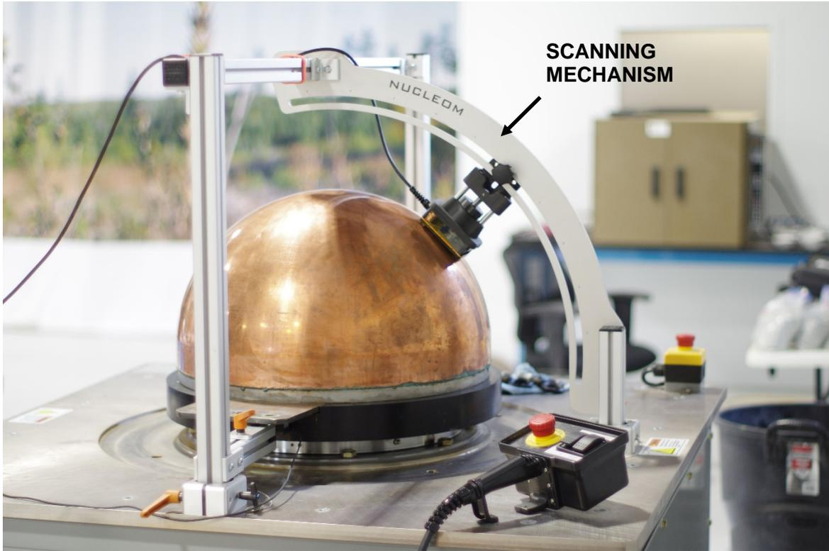
**Figure 4-20: Hemi-head Scanning Mechanism with Eddy Current Probe Attached.**
