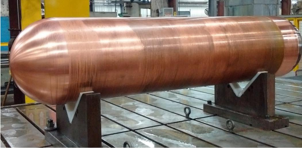
**Figure 4-2: Prototype Used Fuel Container Reference Design**
