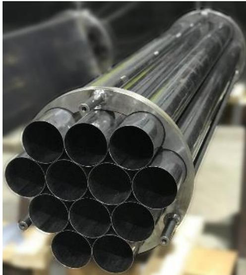
**Figure 4-3: Prototype 2018 Used Fuel Container (UFC) Insert Design**
