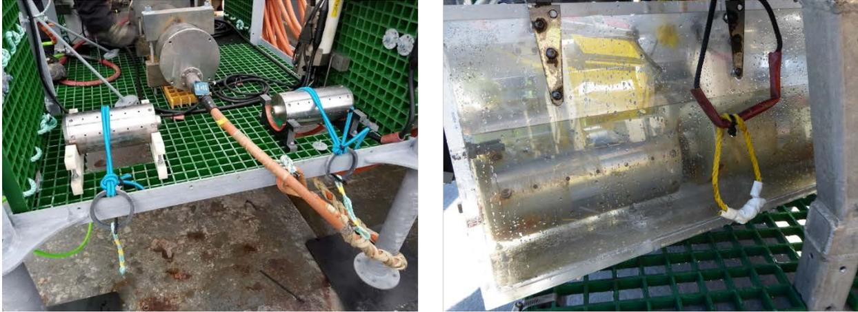
**Figure 4-26: (a) Photos of the Test Modules Containing Copper Embedded in Bentonite Clay on the Immersion Platform; (b) Recovery of Modules Following a 6-month Test Immersion in the Pacific Ocean**
