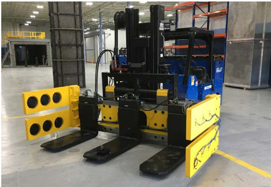
**Figure 3-17: Buffer Box Attachment Installed on Versa Lift 25/35**
