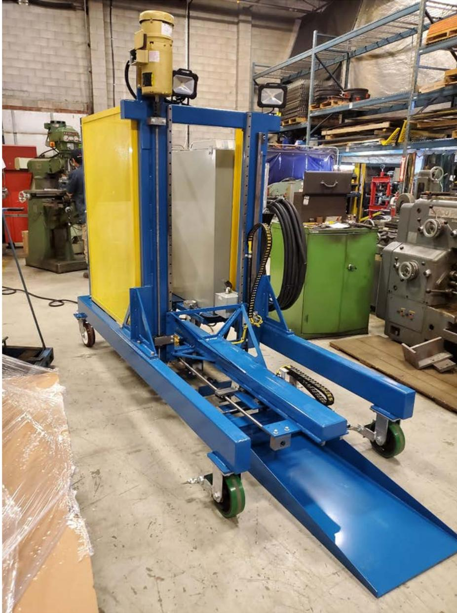
**Figure 3-18: Fork Pocket Brick Delivery Equipment**
