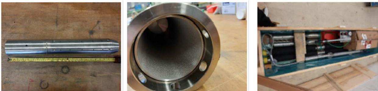
**Figure 4-27: (a) External View of Borehole Test Module Measuring Approximately 50 cm in Length; (b) Internal View of Test Module Showing Sintered Steel Mesh Which Lines the Modules; (c) Custom Made Packers (black) and Supporting Equipment to Install the Borehole Experiments.**
