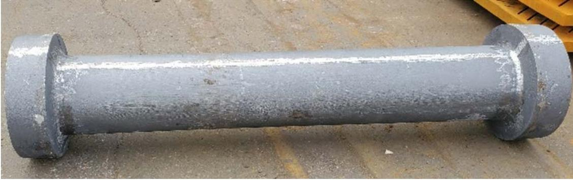
**Figure 4-4: Fabricated Dummy Cast Iron Insert**
