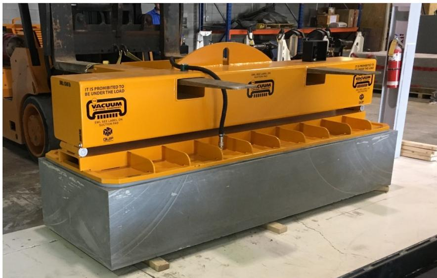
**Figure 3-14: Vacuum Lift Highly Compacted Bentonite (HCB)**
