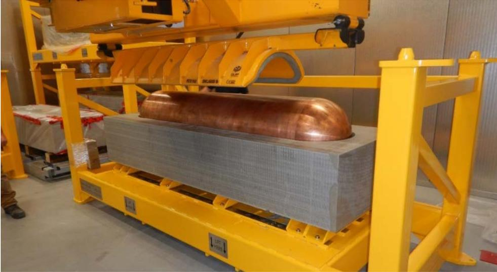
**Figure 3-15: Vacuum Lift Used Fuel Container (UFC)**
