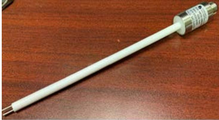
**Figure 4-36: Capacitive Based Moisture Sensor**
