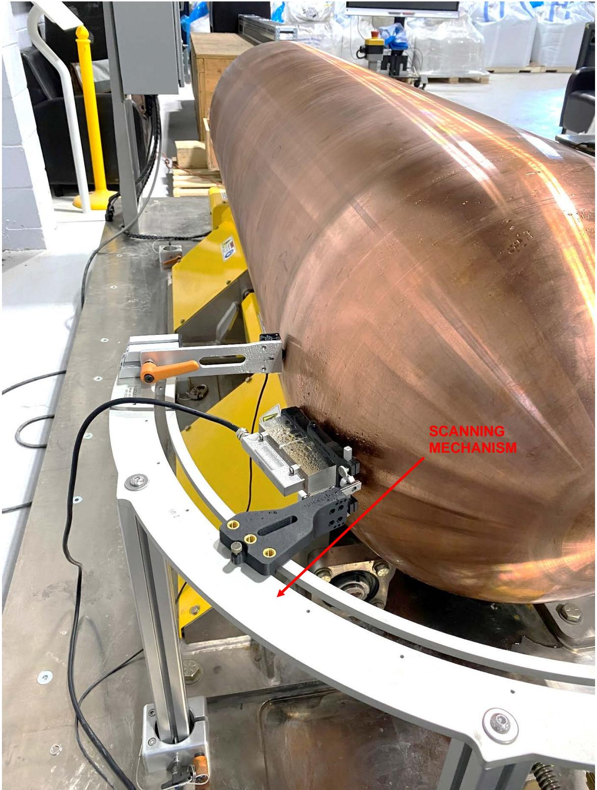
**Figure 4-21: Lower Assembly/Used Fuel Container (UFC) Scanning Mechanism with Ultrasonic Probe Attached**
