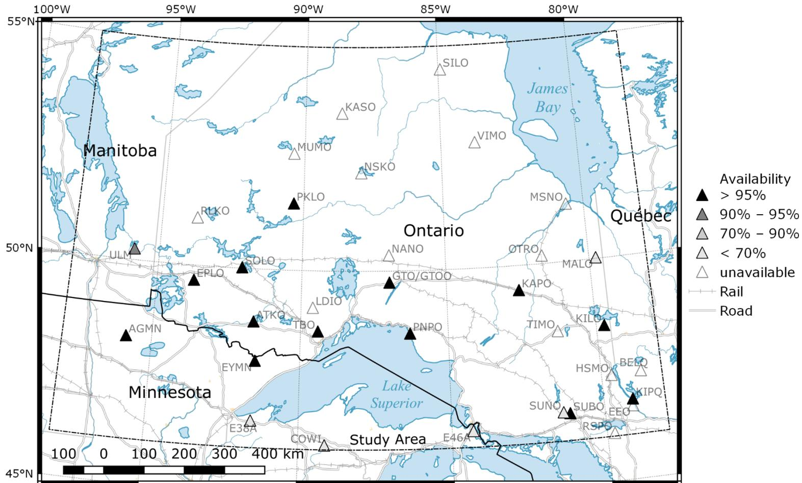
**Figure 1: Seismograph Stations in northern Ontario, 2019.** The study area is outlined with a dash-dotted line. Historical and currently active stations are shown as triangles, with the triangle filled according to data availability for 2019 (see also Table 1). Most of the stations shown as “unavailable” are former FedNor stations which were mainly active 2006–2009; an exception is EEO, which was replaced by KIPQ in 2018. Historical analog stations are not shown.
