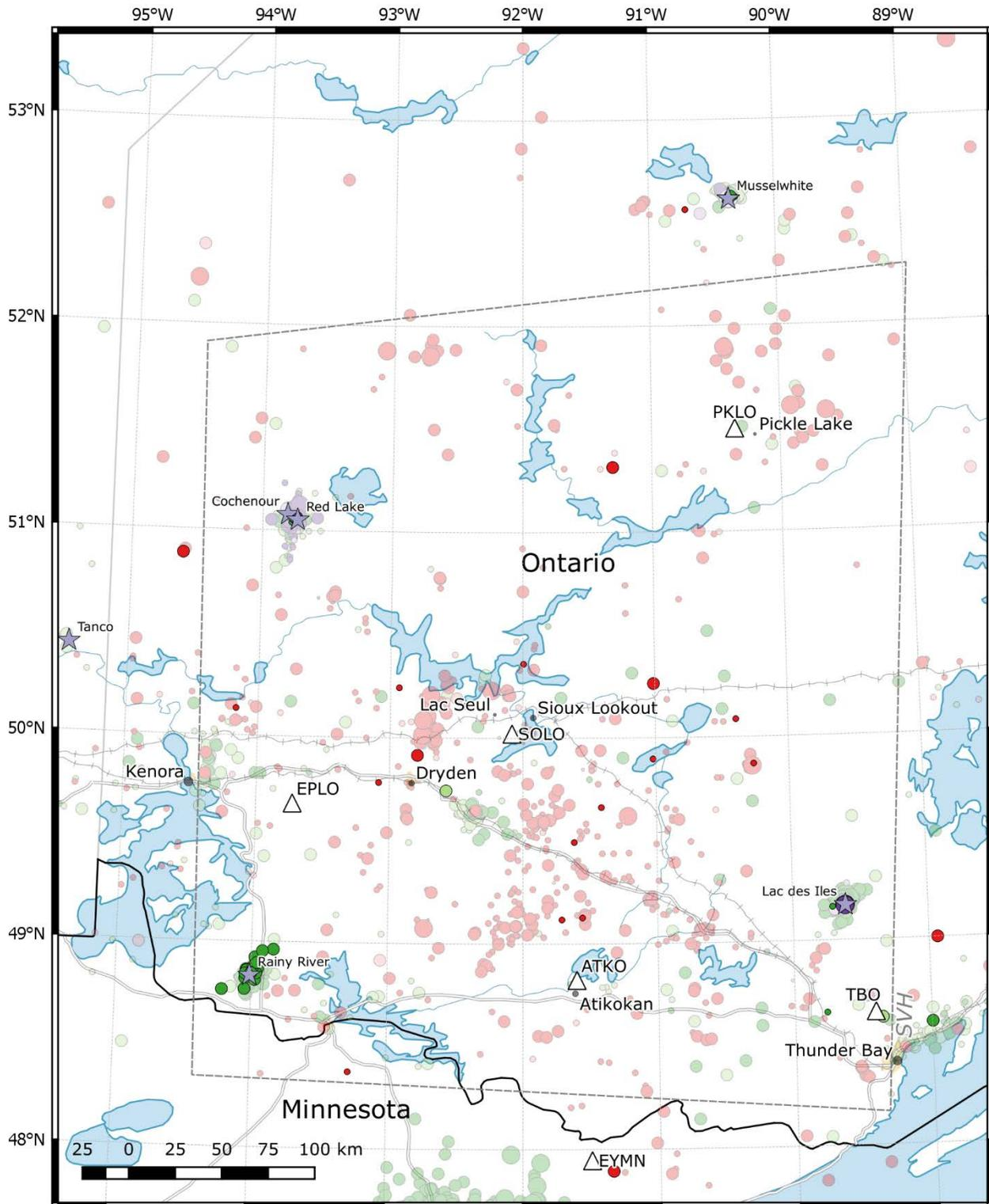
**Figure 8: Seismic events in the Severn Highlands, 2019.** Legend and notes as for Figure 6. In addition, producing mines from the Atlas of Canada (Lands and Minerals Sector; National Energy Board 2020) are shown as purple stars and seismic zones of the 2015 national seismic hazard model (Halchuk, et al. 2014) are outlined with dashed lines. Seismic zone abbreviations: SVH – Severn Highlands.
