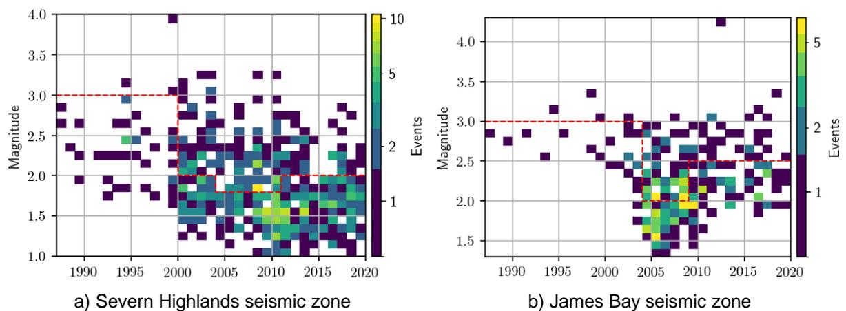
**Figure 4: Earthquake magnitude-time densities for selected sub-regions, 1987–2019.** Earthquakes have not been declustered. Dashed red lines are crude estimates of the magnitude of completeness with time, and are only intended to guide the eye.
