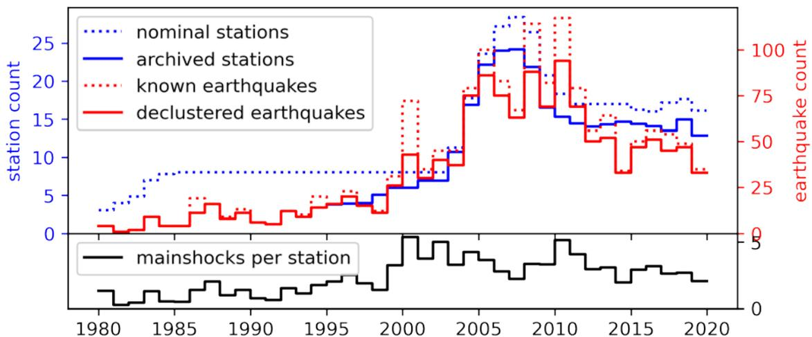
**Figure 3: Earthquake and station counts in northern Ontario, 1980–2019.** See Table 2 for explanation of terms. Note the national waveform archive only contains continuous data starting in 1995. The number of earthquakes per station is the number of declustered earthquakes per nominal station.
