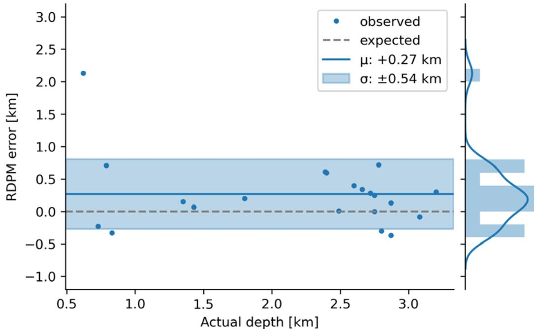
**Figure 15: Accuracy of RDPM depth estimates for shallow mining events, 2016–2019.** RDPM error is the estimated depth minus the actual depth reported by the mine operator. The mean  $\mu$  and standard deviation  $\sigma$  of the distribution are indicated.
