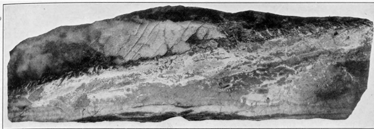
**Figure 27: Image of a vein of native copper (light) and chalcocite (dark) from the Baltic mine (Butler and Burbank 1929). The exact locations of the copper and chalcocite veins were not identified in the original publication. Credit: U.S. Geological Society.**
