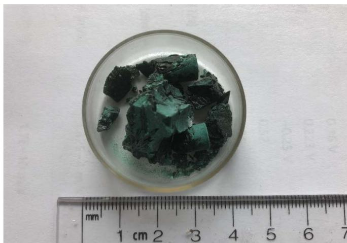
**Figure 29: Remnants of a mineral sample used to fabricate an atacamite disc electrode for dissolution studies.**
