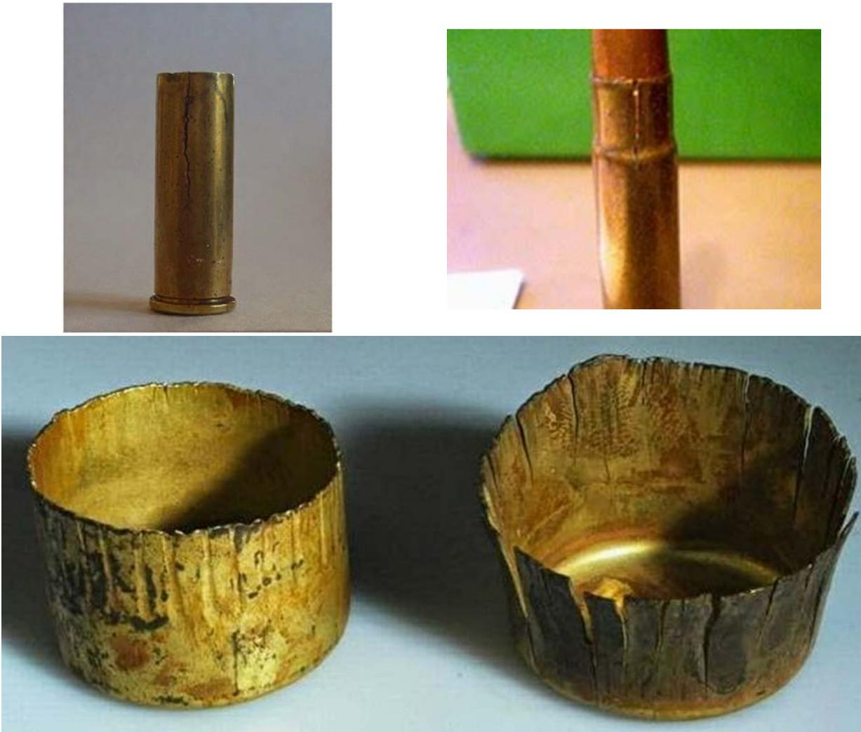
**Figure 13: Various images of the season cracking of brass cartridge case**
