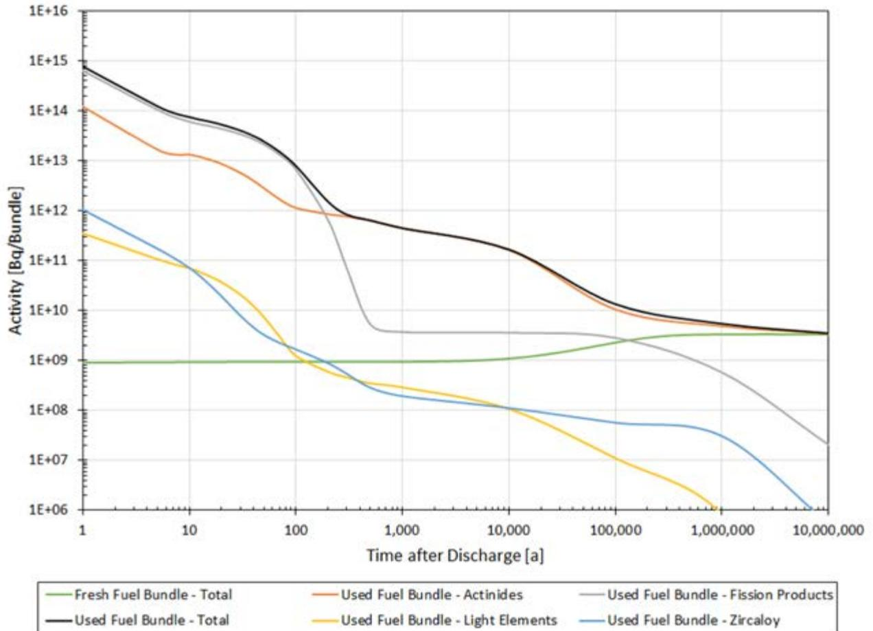
**Figure 2.2: Radioactivity of used CANDU fuel decreases with time (fuel burnup of 220 MWh/kgU)**
