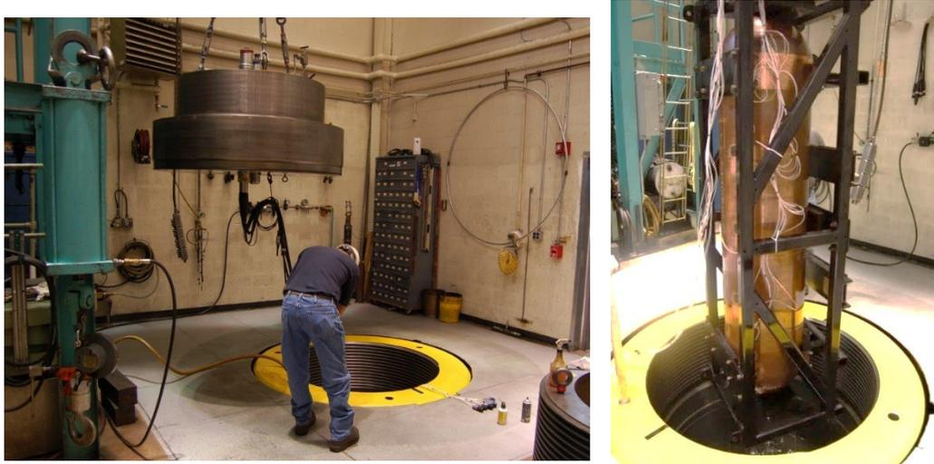
**Figure 7.5: Prototype Used Fuel Container subjected to external pressure equivalent to almost 6 km underwater. (Left) Test chamber lid being lowered into place; (Right) Container removed after testing; fully intact – no containment failure.**
