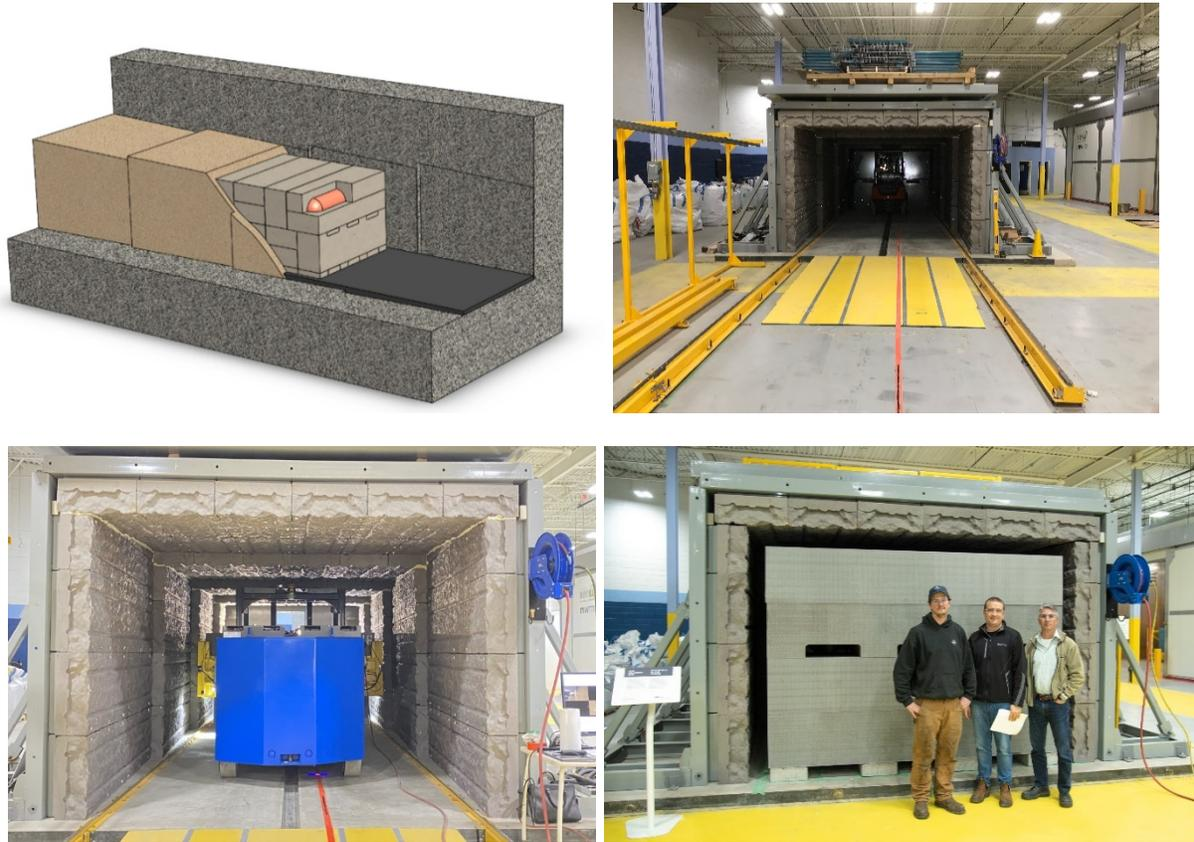
**Figure 7.8: (Top left) Emplacement room concept; (Top right) Full-scale mock emplacement room at NWMO Test Facility; (Bottom left) Emplacement machine travelling inside room; (Bottom right) Stacked buffer boxes.**
