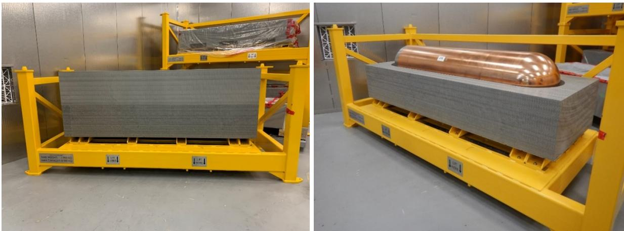
**Figure 7.6: Prototype Buffer Box and Used Fuel Container**
