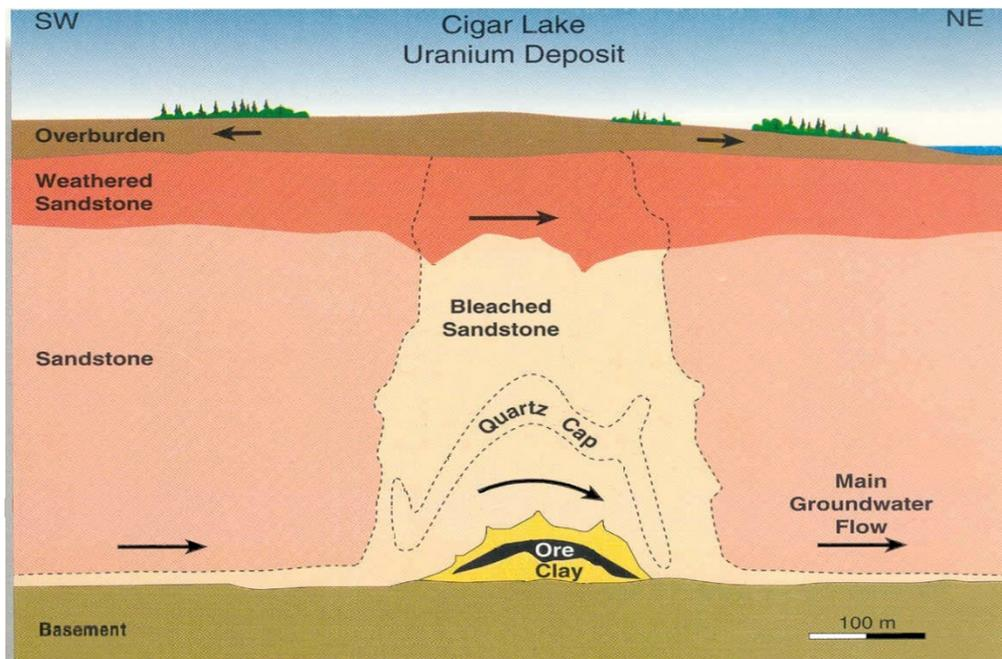
**Figure 9.1: Cross-section of the Cigar Lake uranium ore body in Saskatchewan (adapted from Cramer and Smellie 1994). The uranium ore, surrounded by a clay layer at 430 m depth, has remained isolated from the surface environment for over 1.3 billion years.**
