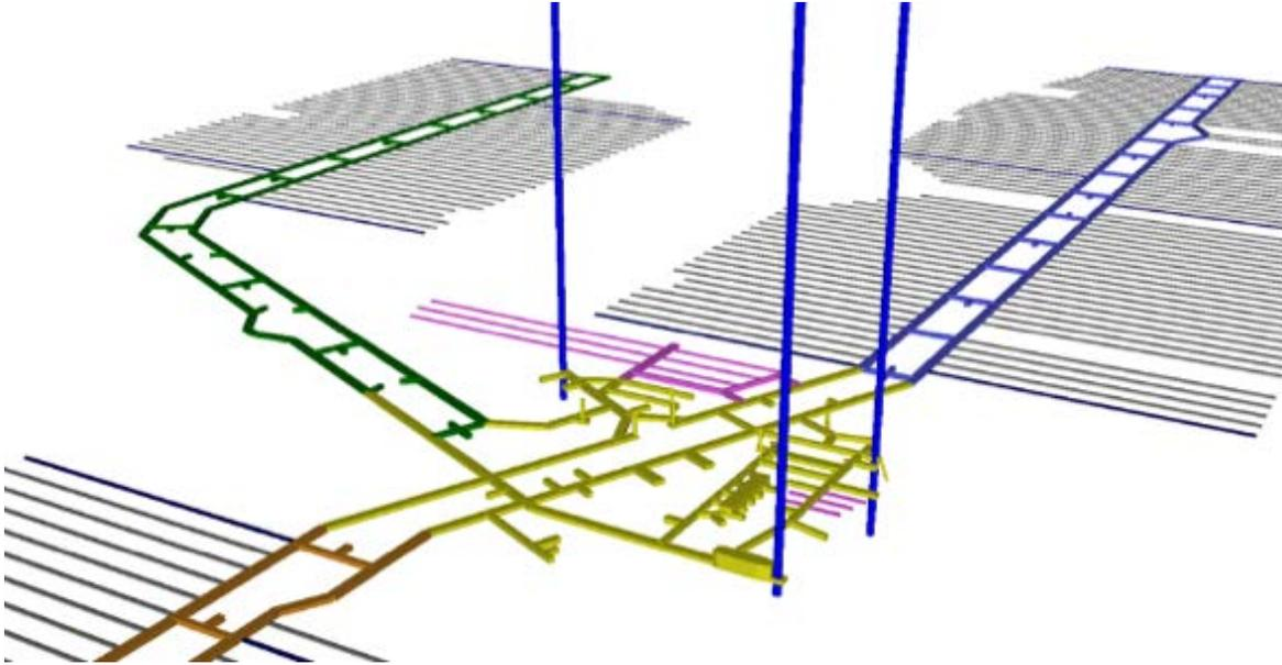
**Figure 12.1: Illustration of centralized service area of repository showing the underground demonstration areas (highlighted in purple). (For illustration purposes only; does not reflect site specific layout for Revell Site).**
