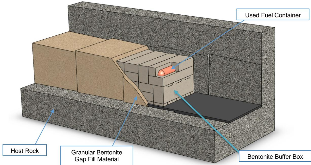
**Figure 7.3: Cutaway illustration of emplacement room concept**
