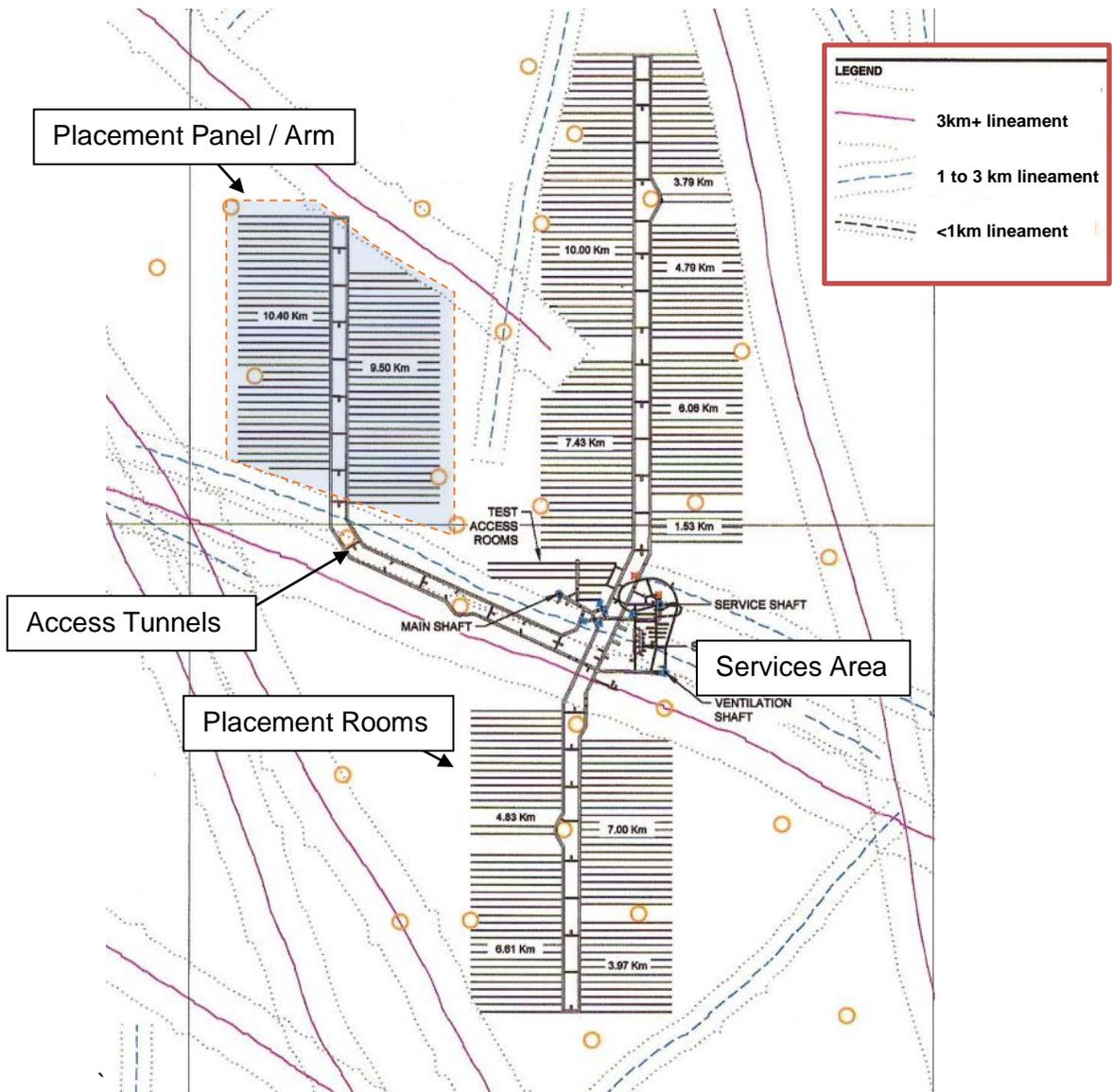
**Figure 7.9: Conceptual underground repository layout for a hypothetical crystalline rock site, showing services area, access tunnels, placement arm panels, and emplacement rooms. Lineaments and layout are for illustration purposes only and do not reflect the Revell site conditions.**
