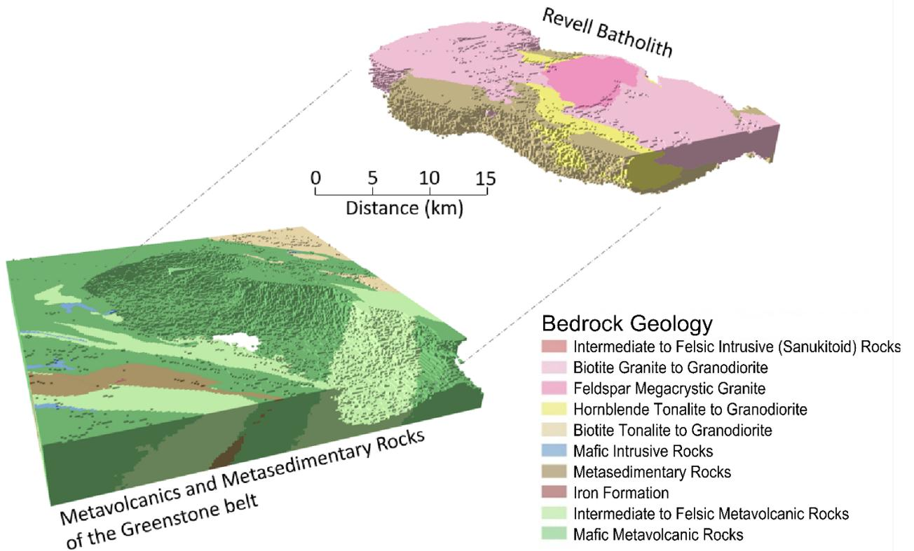
**Figure 3.2: 3D regional geophysical/geological model of the Revell area. Note that the open white space in the centre of the bottom left image indicates the lower boundary of the model, at 4 km below ground surface.**
