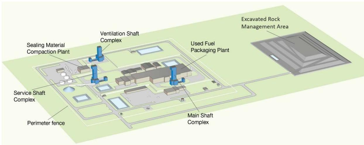
**Figure 7.10: Illustration showing conceptual DGR surface facility layout**
