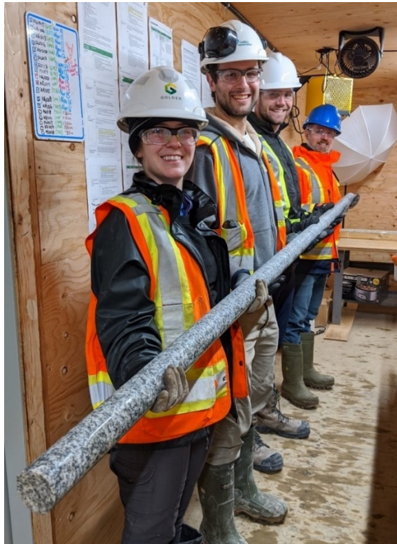
Figure 3.3: Example of an intact, three-metre long, section of drill core displaying the low fracture frequency typical of the Revell Site.
