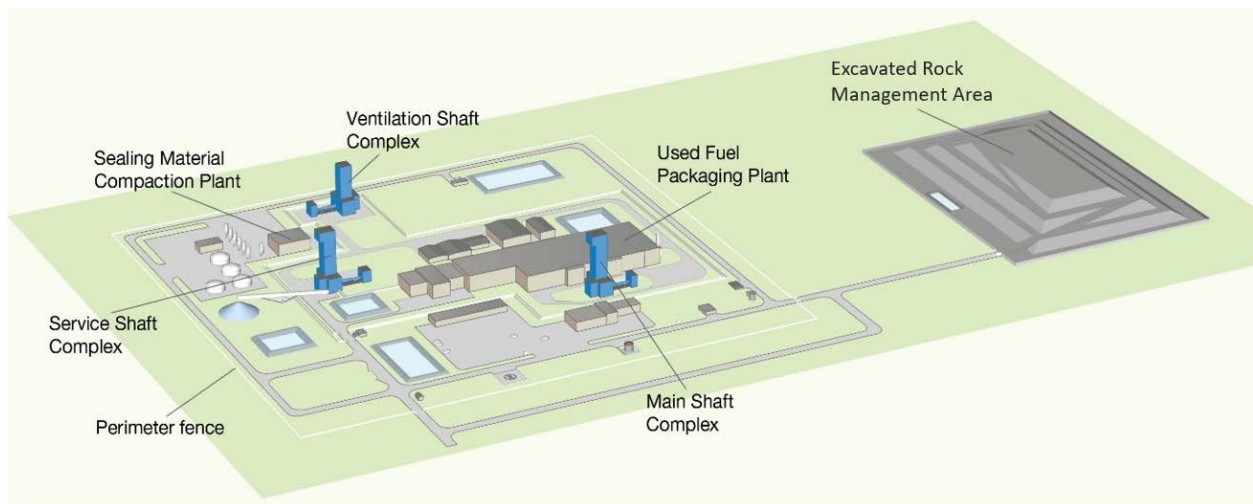
Figure 7.10: Illustration showing conceptual DGR surface facility layout
