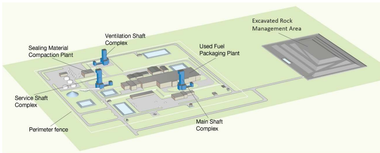
Figure 7.10: Illustration showing conceptual DGR Surface Facility Layout
