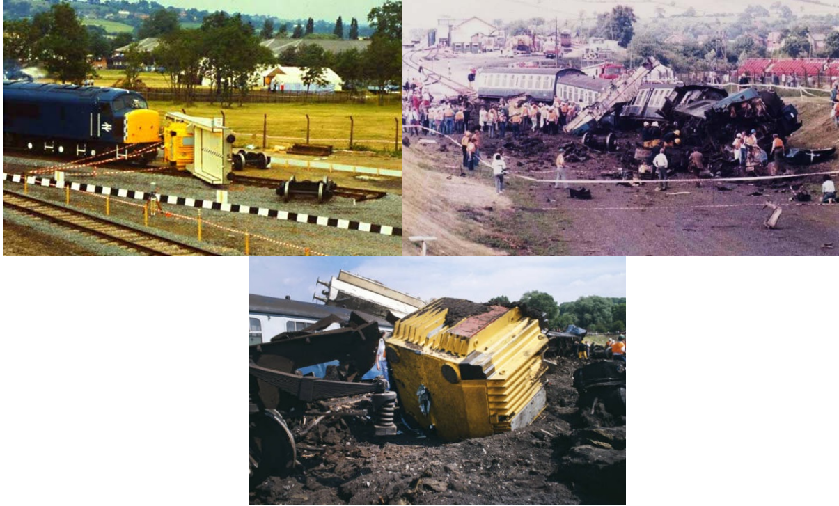
Figure 8.3: Photos from "Operation Smash Hit". A used fuel transportation package in direct collision with train traveling at 160 km/h with no release of contents. (Clockwise) Depicts train just before collision, after collision, and dented but intact package among wreckage.
