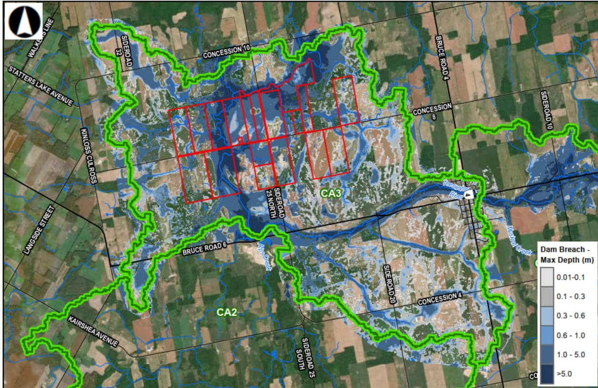
**Figure 20: Scenarios 13 and 14 – Floodplain Boundaries for End-of-Century (95%) for Dam Breach showing Maximum Depth of Water**
