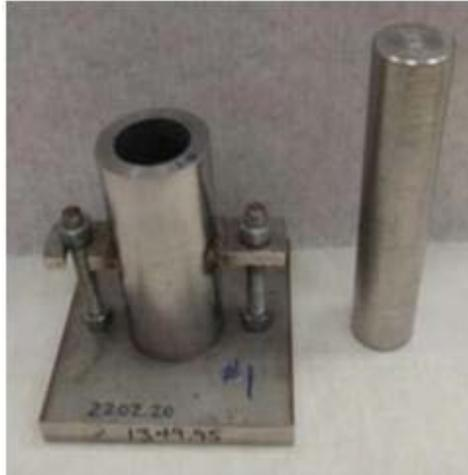
**Figure 5.1. Miniature compaction device**
