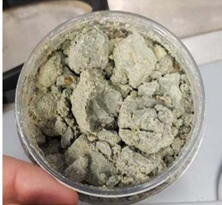
**Figure 4.1. Example of raw, unprocessed Wyoming bentonite**
