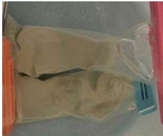
**Figure 4.2. Soluble salt removal from brine-soaked specimens by diffusion through dialysis membrane (Dixon et al. 2018)**
