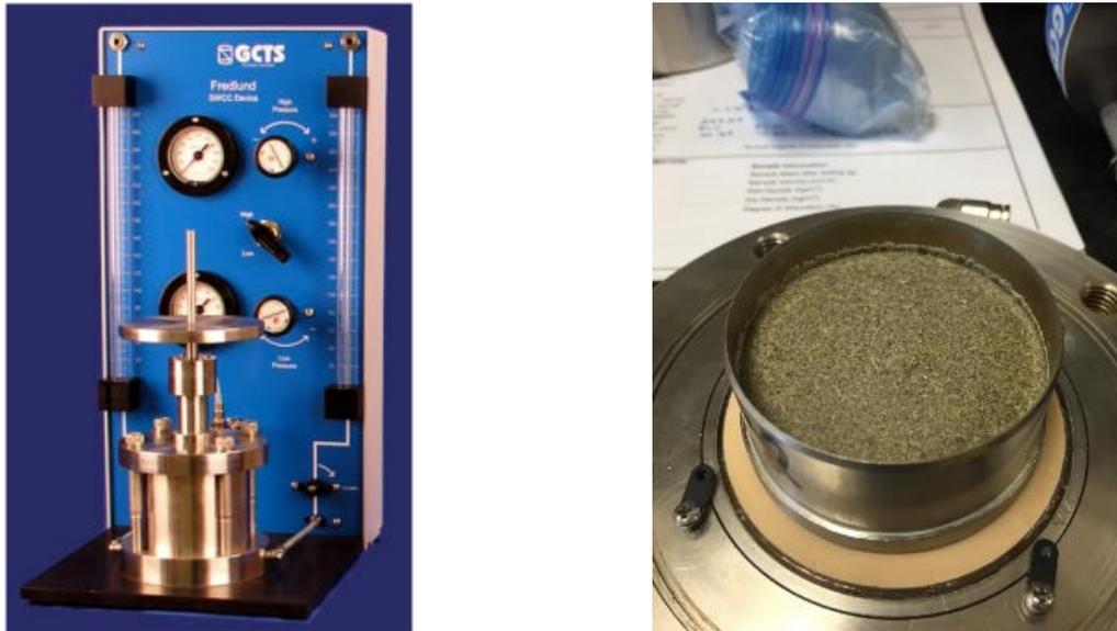
**Figure 7.2. GCTS apparatus used to measure the SWCC in low suction range and a typical SWCC specimen**
