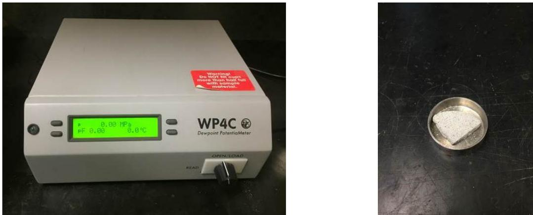
**Figure 7.3. WP4 device used to measure the SWCC in the high-suction range and example of specimen used**
