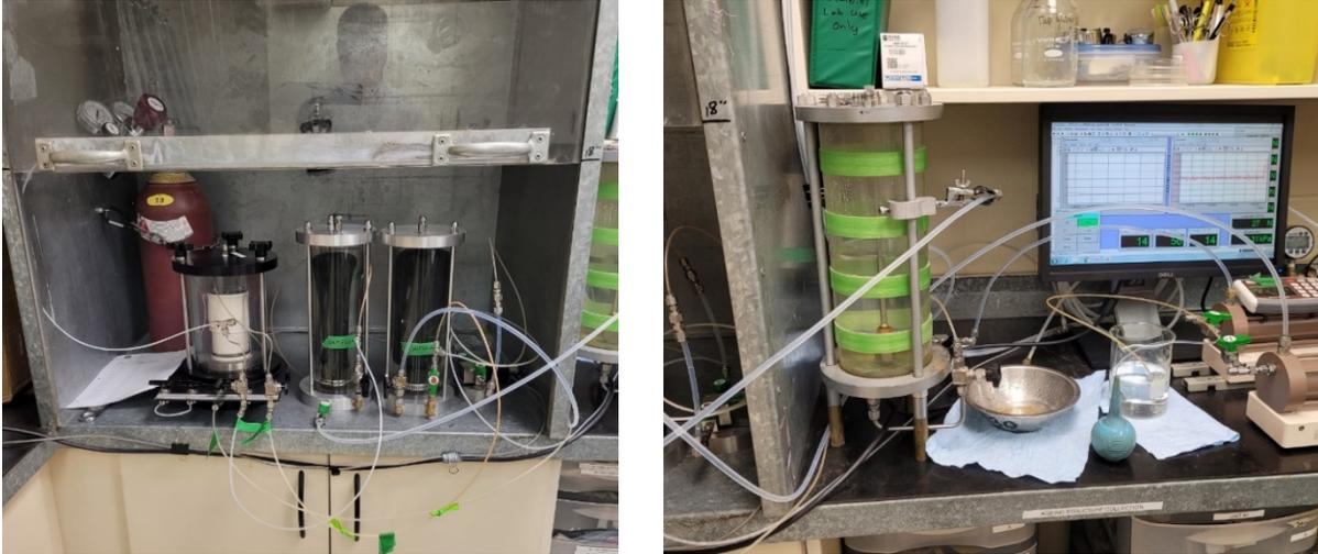
**Figure 7.10. Gas permeability equipment showing triaxial cell and methane test apparatus**
