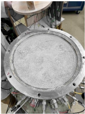
d. Final GFM layer placed
