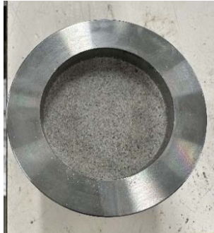
(c) Compacted bentonite-LHHPC in the cell
