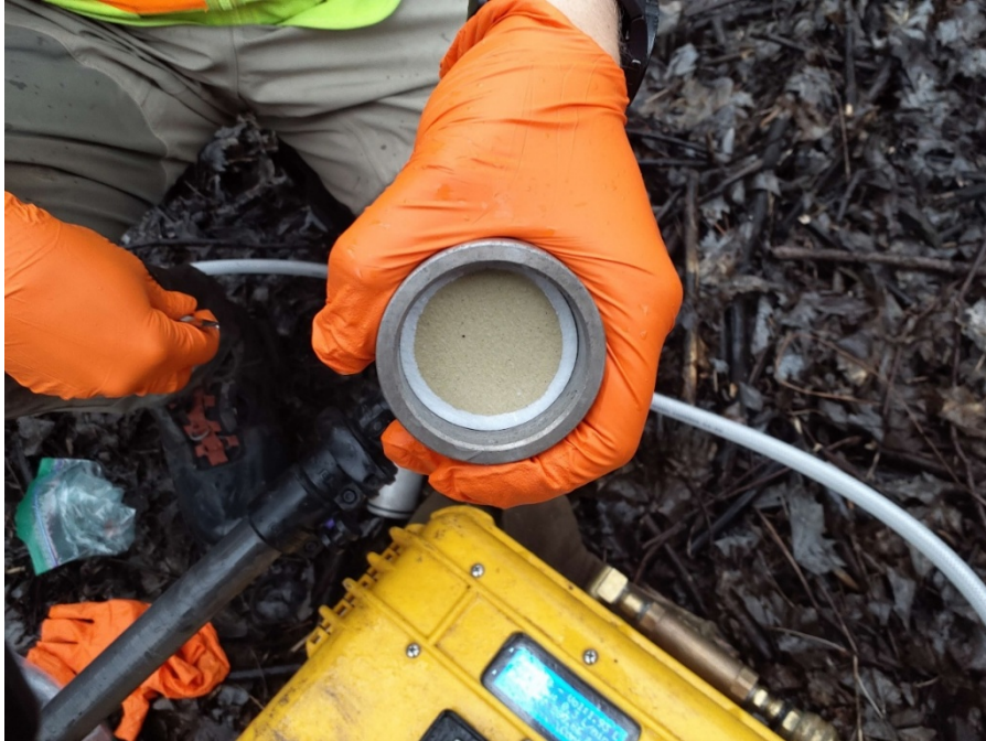
Figure 7-9: Filter paper after passes through OSMOS sampler. The filter paper is extracted using sterile tweezers and sent to Hanner Lab at the University of Guelph. Photo was taken in April 2024 by North/South Consultants.
