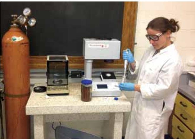
University of New Brunswick Ph.D. Candidate Magda Celejewski calibrates a near infrared (NIR) spectrometer to determine the mass of water extracted onto filter papers from low porosity rock cores.
