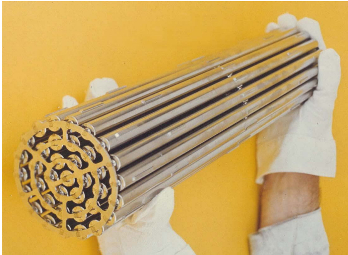
FIGURE 3: NUCLEAR FUEL BUNDLE USED IN CANDU REACTORS
