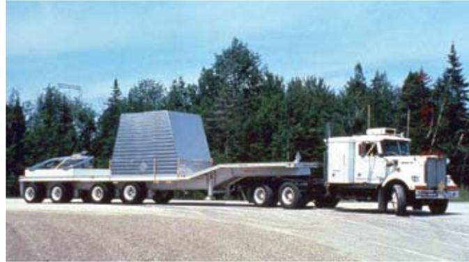
Figure 3: Tractor-trailers for road transport of used nuclear fuel: OPG (above); Areva (right).
