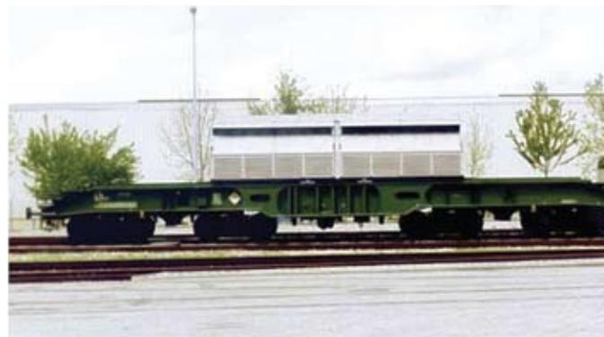
Figure 4: Rail car with a transportation cask used in Europe (left); the rail-to-road transfer facility near La Hague in France (below). Photos from Areva.
