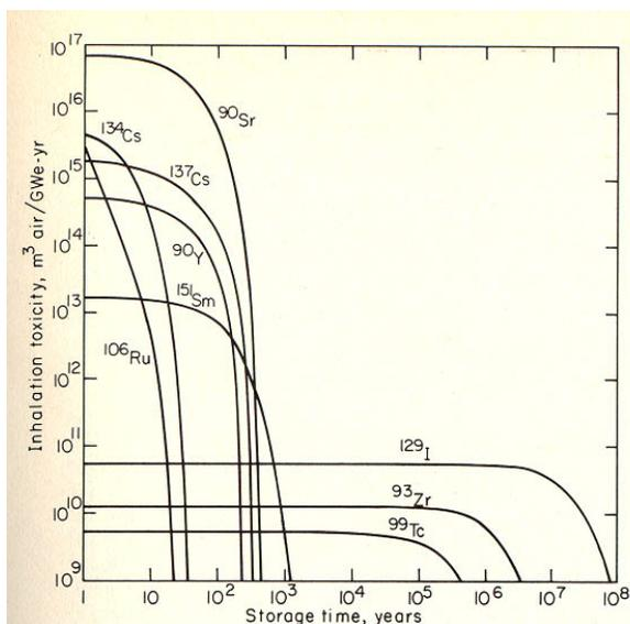
Figure 8.3 Inhalation toxicity of the fission products from a uranium-fueled LWR.
