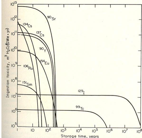
Figure 8.4 Ingestion toxicity of the fission products from a uranium-fueled LWR.
