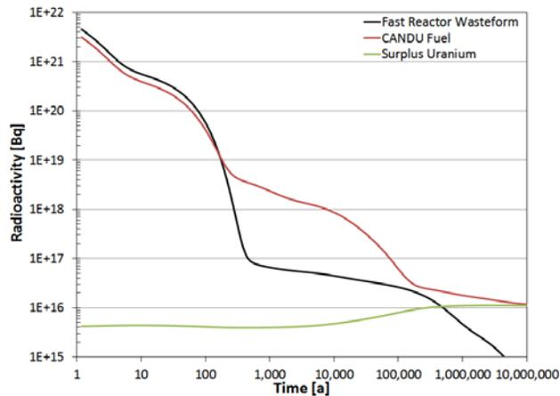
Figure 3 Wasteform total radioactivity.
