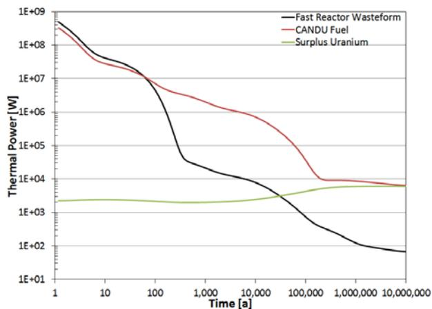
Figure 5 Wasteform total thermal power.
