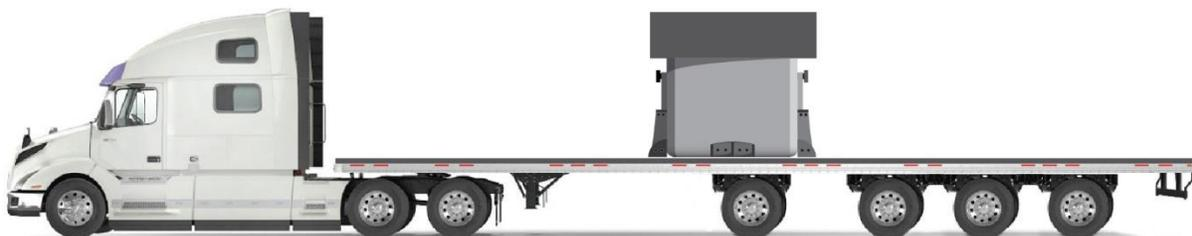
Each tractor-trailer unit proposed for the transport of UFTPs and BTPs can carry one package per shipment as depicted in **Figure 7**. A Conestoga cover could be added to the flatbed to protect the UFTP or BTP from the elements during transit.
